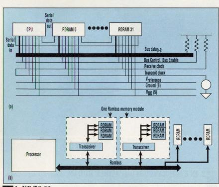
1. UP TO 32 dedicated Rambus-compatible RDRAMs can be connected directly to the CPU in a combination parallel bus and daisy-chain scheme (a). Alternatively, up to 32 RDRAMs can be grouped into a module, and up to 10 modules can be plugged into one Rambus (b).
