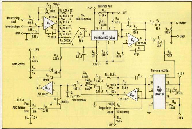
ATTACK AND RELEASE times for this AGC audio amplifier can be adjusted by the three-position Attack switch (Sw<sub>2</sub>) and the AGC Release pot (R<sub>32</sub>), respectively. The output is rated for a 10-k $\Omega$  load. To work into 2 k $\Omega$ , C<sub>8</sub> must be replaced by a 100- $\mu$ F, 15-V device.
