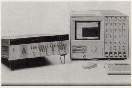
Designers who must make precise parametric measurements on digital devices with clock rates from 100 MHz to 3 GHz will find the HP 8133A ideal for the task. The instrument delivers 1-ps edge-placement resolution, 100-ps timing accuracy, and pulse widths of 150 ps to 10.000 ns. Rise times (10% to 90%) are 100 ps, and jitter is less than 5 ps. Signal accuracy is maintained continuously, even during frequency changes, eliminating the possibility of glitches that would corrupt measurement results.
