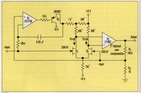
1. LOW-NOISE FETs  $Q_1$  and  $Q_2$  minimize the noise level of this chopper-stabilized amplifier. For best performance, the Toshiba 2SK147 FETs must be  $V_{\rm gs}$  matched to within 10% and thermally mated. The resistors marked with an asterisk are 1% thin-film devices.
