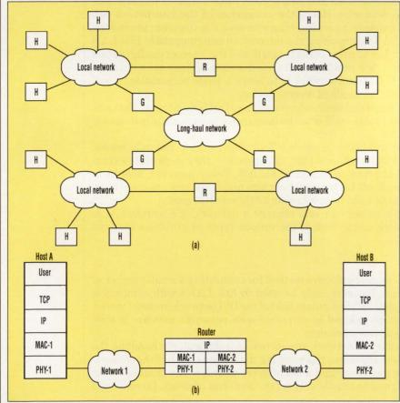
1. THIS GLOBAL INTERNET includes local-area networks (LANs); hosts (H), which concentrate user connections onto the LANs; routers (R), which connect the LANs to one another; and gateways (G) that provide access to worldwide communication services (a). The routers implement the first three layers of the OSI network protocol standard (b).
