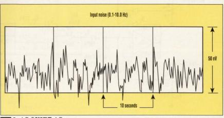
2. AS QUIET AS the best bipolar amplifiers, this FET-input circuit generates less than 50 nV of peak-to-peak noise over the band from 0.1 Hz to 10.0 Hz.
