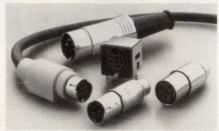
and electrical standards and comes in 3- to 8-pin configurations. All will accept #22 to #28 AWG wire sizes. Silver-plated brass contacts are standard with gold available optionally. Prices range from \$0.51 to \$0.74 each in lots of 1000.
