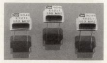
A series of ECL clock oscillators in half-size packages come in both through-hole and SMT styles. The E500 Series comes in frequencies from 24 to 180 MHz. Both standard and industrial temperature ranges are offered. Frequency stabilities are available to 25 ppm. Supply voltages are -5.2 V dc, -4.5 V dc, or 5 V dc. Model E531 (120-MHz unit) costs \$43.90 in prototype quantities. Delivery is from stock to seven weeks.
