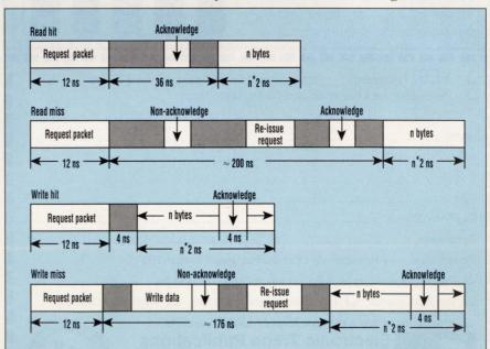
3. ALL BUS TRANSFERS for the 4.5-Mbit RDRAM start with a packet request that requires 12 ns. Once the memory chip and bus-overhead operations are completed, data transfers can take place every 2 ns. One to 256 bytes can be transferred during a Read Hit or Miss, or a Write Hit or Miss operation.
