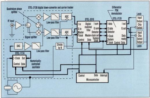
5. THIS THREE-PIECE spread-spectrum demodulator ASIC chip set developed by Stanford Telecom is used in a spread-spectrum receiver. One particular chip, the STEL-2130, integrates many functions that formerly required several chips.
