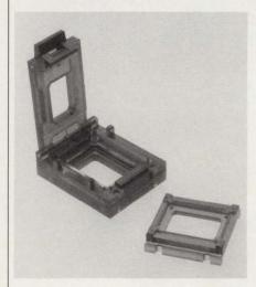
A test and burn-in socket for multichip modules handles a 256-pin unit with a 0.65-mm, 45-by-45-mm body. The socket accommodates one of the outlines included in a proposal made for package-outline standards at the recent JEDEC JC-11 meeting. Suited for high-density test and burn-in, the
