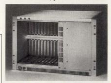
includes a 12-slot VME card cage, a 400-W power supply with integral cooling, and a Eurocard subrack featuring a 10-layer J1/J2 VME backplane. The cage fits into 12-1/4 in. of rack space. List price is \$2495 with delivery in four to six weeks.
