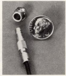
version for underwater or high-pressure applications. Capable of handling  $500\,\mathrm{V}$  dc and  $300\,\mathrm{V}$  ac at  $2\,\mathrm{A}$  per 0.5-mm contact, thi unit will accommodate a  $\#\,30$  AWG wire. Call for pricing and delivery.
