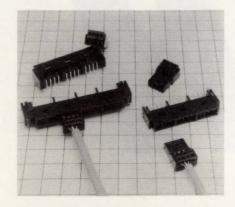
telephone equipment, the connectors are available with IDC crimping and have an applicable cable diameter of 0.40 to 0.65 mm. Current rating of the series is 2 A, rated voltage is 250 V ac, and insulation resistance is 100 MΩ minimum at 500 V dc. Pricing starts at \$1.25 in lots of one to 25 for a four-contact unit.
