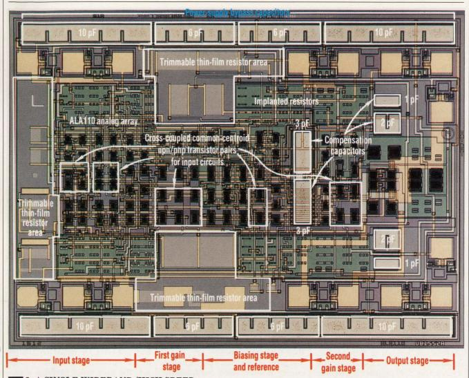
2. A SINGLE WIDEBAND/HIGH-SPEED analog circuit, such as a 200-MHz op amp or a 1-ns ECL comparator, can be contained within AT&T's ALA110 analog array. The smaller input-stage transistors are located on the left, increasing in size from left to right.
