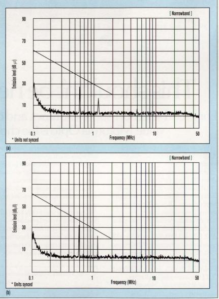
3. IN BOTH INDEPENDENT and current-sharing modes, the MFLHP converters offer several different synchronization schemes to help reduce interference from switching noise. With three current-sharing units operating in a free-run, unsynchronized mode (a), common spectral peaks are lower than in synchronized units (b). Synchronization, however, eliminates the chances of beat frequencies and allows switching transients to be timed to avoid circuit interference.
