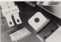
ment, residual-force crimp for termination of flat copper cable, eliminating the need to strip insulation. They're also pluggable and permit running taps off the flat cable. Connectors are rated at from 70 to 110 A, depending on configuration, with a 30°C or less temperature rise. A typical 1-ft. cable assembly with connectors on both ends runs from \$5.23 to \$6.38 in lots of 1000. Delivery is from four to six weeks.
