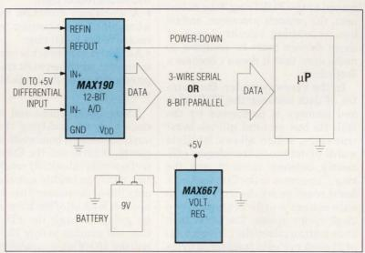
On battery power, the MAX190 converts rail-to-rail signals to either serial or parallel data in 7.5µs.
