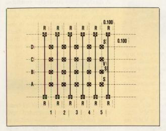
4. The actual connector pattern of the stripline design in Figure 3 shows that holes dedicated for shielding and power functions are located in a staggered position from the signal fields.
