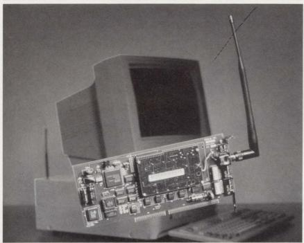
3. A PC ADAPTER CARD from Proxim is based on a patented spread-spectrum technology that provides three communications channels and a data rate of 242 kbits/s. In addition to having a small antenna that extends from the PC backplane, the full-size ISA card provides driver support for a variety of network software. Maximum transmitting range is 800 ft.
