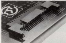
tacles which become the card interconnect, and headers which are installed in equipment to mate with the cards are included. Contacts have independent twin-beam construction for a minimum of 5000 mating cycles. Pricing is about \$0.05 per mated position. Delivery is in eight to 10 weeks.
