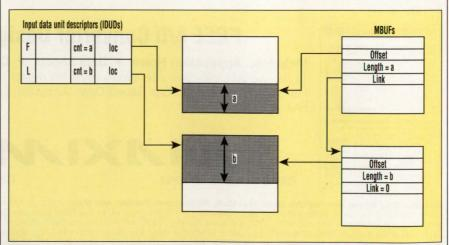
5. MEMORY MANAGEMENT in the Freeway router uses Unix MBUF structures. After a frame is delivered to the memory from the FDDI networks, the CPU links the frame segments together with MBUFs. Doing so eliminates the need to copy the data, and thereby greatly increases the router's forwarding capability.
