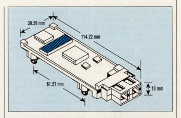
trol, laser driving, and signal retiming and demultiplexing logic. An additional chip for the optical signal detector (a transimpedance amplifier) is required for the receive channel. The chip set can be configured to handle the optical-fiber interfaces, or as an option, a limited-distance ECL coaxial-cable interface. The companies are also working on chip sets to support the higher-speed fiber-channel options.
