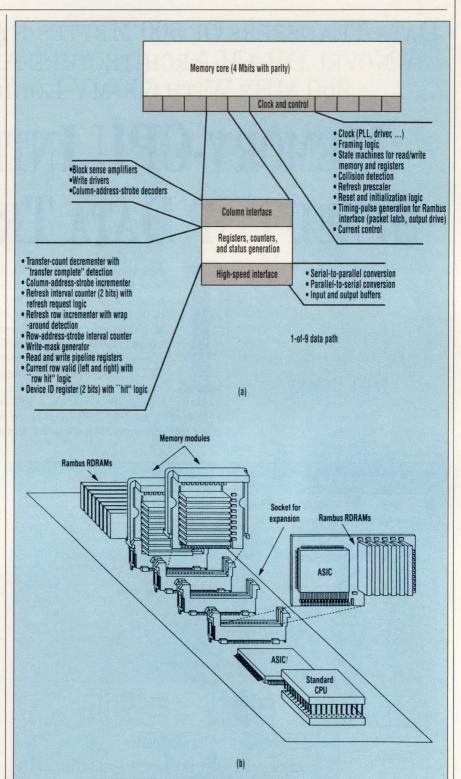
2. IN EACH RAMBUS-COMPATIBLE RDRAM, special clock and control blocks were added to handle the Rambus interface and protocol. Additional circuitry in each bit-line interface performs the serial-to-parallel and parallel-to-serial conversion needed for high-speed data transfers (a). A typical RDRAM module that contains up to 32 RDRAMs and a transceiver chip can plug into a Rambus "motherboard," which hosts up to 10 modules, for a total capacity of 160 Mbytes, using 4.5-Mbit RDRAMs (b).
