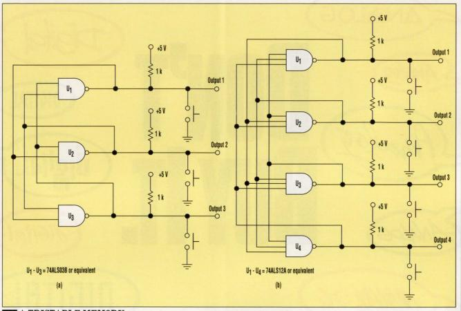
A TRISTABLE MEMORY element is formed by connecting three two-input NAND gates such that each gate's output goes to an input on the other two (a). A quadristable memory element uses four three-input NAND gates (b).
