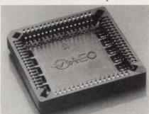
MO-47 and MO-52 plastic leaded carriers on 0.050-in. centers and permit surface-mount termination to existing pc-board footprints. A high-temperature insulator is compatible with vapor-phase and infrared soldering. Sockets come in 20, 28, 32, 44, 52, 68, and 84 positions. Typical unit price for small lots is \$2.53. Delivery is from stock to four weeks.
