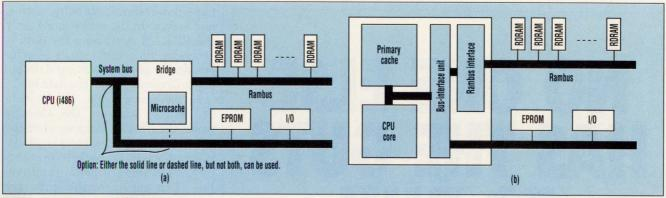
4. TO TIE A SYSTEM into the Rambus, designers can either create a "bridge" chip that ties into a standard host chip, such as an 80486 CPU (a), or create a custom host chip that has one or more Rambus interfaces as well as a standard interface bus (b).
