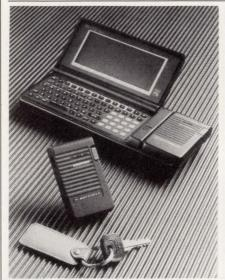
1. ONE-WAY WIRELESS transmission allows users of Hewlett-Packard's 95LX palmtop computer to receive information through national, regional, or local radio-paging services. Communications is provided by Motorola's NewsStream receiver, which mounts in a cradle tied to the computer.
