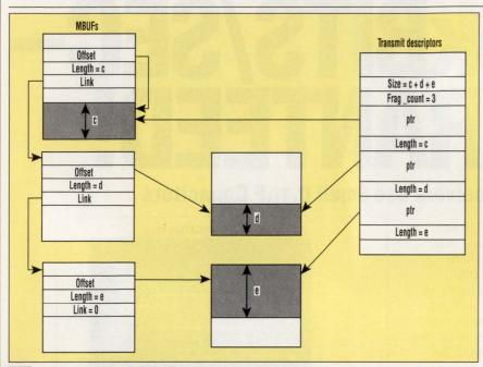
6. THE DATA FIELD of the MBUF structure can hold the frame header to more efficiently process frames. Data is easily passed from protocol processing software to the Sonic Ethernet controller by a method based on transferring pointers and length indicators. Because data needn't be copied with this approach, the maximum forwarding rate can be maintained.
