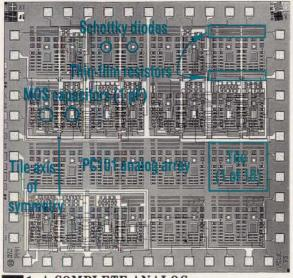
1. A COMPLETE ANALOG "system on a chip" can be built with Raytheon's PC101 analog array. It consists of 16 symmetrical and identical tiles, each with 24 npn and 16 pnp transistors. Each tile has general-purpose, precision, and high-speed/wideband macros.
