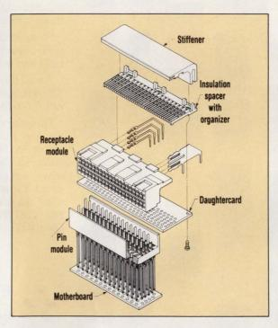
1. With 40 effective high-speed signal lines per inch and a pin count of up to 680 lines, this connector exemplifies the stripline approach used to satisfy high-speed interconnect requirements.
