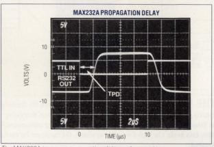
The MAX232A improves propagation delay and symmetry.
