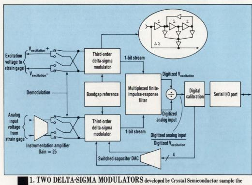
excitation voltages for, and the analog input voltage from, a strain-gage transducer to create a 22-bit (serial) digital word. The word represents the ratio of strain-gage excitation to its output.
