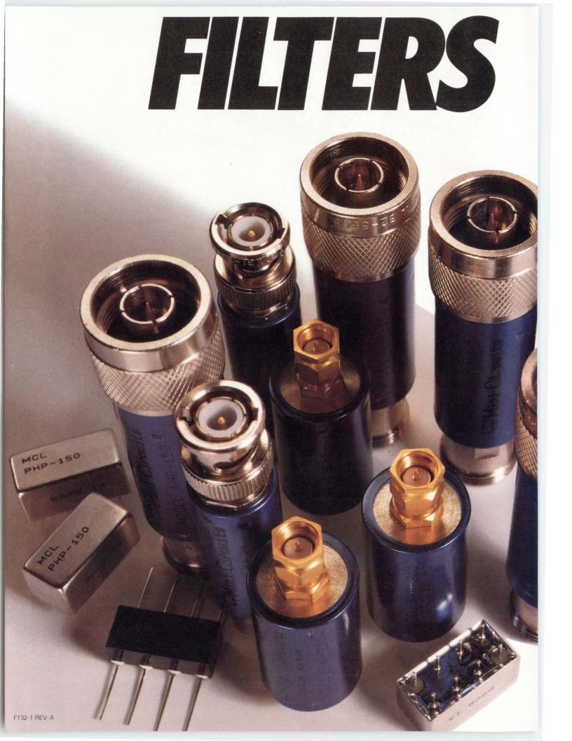
lowpass, highpass, bandpass • less than 1dB insertion loss • greater than 40dB stopband rejection • surface-mount • BNC, Type N, SMA available •5-section, 30dB/octave rolloff •VSWR less than 1.7 (typ) •rugged hermetically-sealed pin models •constant phase
