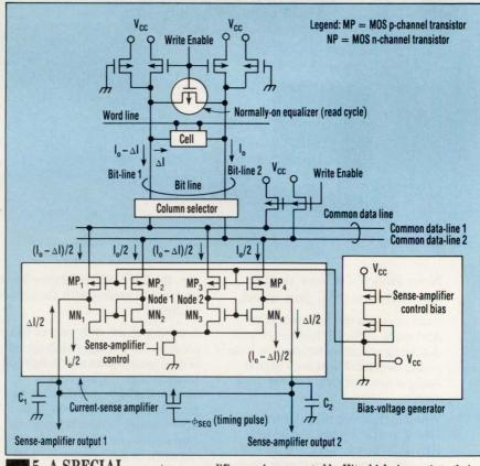
5. A SPECIAL current-sense amplifier was incorporated by Hitachi designers into their ultra-low power (140-mW) high-speed 1-Mbit static RAM. The sense amplifier turns the small current difference between paired bit-lines (the common data lines) into a large voltage swing.
