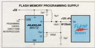
This MAX732 flash memory programmer supplies  $+12V\pm4\%$  at 120mA with 88% efficiency from a +5V source. The shutdown current for this entire circuit is 75µA.
