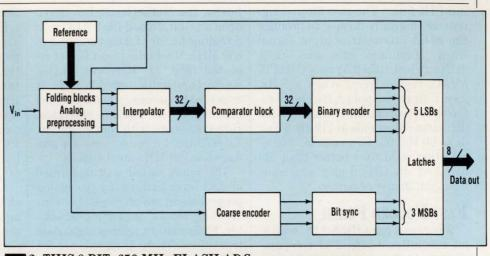
2. THIS 8-BIT, 650-MHz FLASH ADC employs a folded architecture in which analog pre-processors produce the three most-significant bits. The technique, devised by Philips Research, cuts the comparator count from 255 to 32, reducing power to 850 mW and overall die size.
