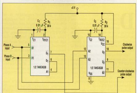
**BUILT AROUND** a dual monostable multivibrator, this circuit functions as a simple quadrature waveform decoder.  $R_1-C_1$  and  $R_2-C_2$  set the period of the outputs, which should be less than the shortest quadrature pulse seen by the system.
