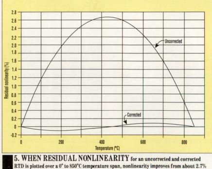
RTD is plotted over a 0° to 850°C temperature span, nonlinearity improves from about 2.7 to 0.08%, a better than 30-fold improvement. If a smaller temperature span is chosen, residual nonlinearity can be reduced to even lower levels.
