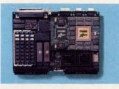
master/slave VME interface. The PaceRunner/3400 VME SBC can be used in workstations, servers, industrial and process control, imaging, communications, simulation, and software development platforms.
