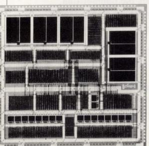
5. A VIDEO DSP CHIP from Matsushita crams 930,000 CMOS transistors on a 12.38-by-12.90mm die and uses a 16-bit fixed-point data format. The processor has a 16.5-ns instruction cycle at 60 MHz and dissipates 2.4 W at 5 V. Each of three 16-bit-by-1kword data RAMs (dark areas across the top) has an address generator. The dark areas on the right are 32-bit-by-1-word instruction memories. Discretecosine-transform circuitry appears across the bottom of the chip.
