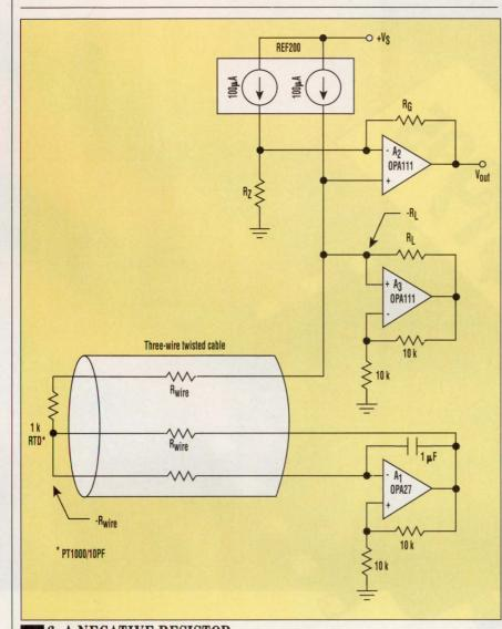
6. A NEGATIVE RESISTOR, realized with op-amp A1, cancels the effects of cable wiring resistances. Op-amp A2 forms a negative resistor that linearizes the RTD.
