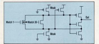
2. A SIMPLE DISTRIBUTED NOR circuit developed by Sun Microsystems and Texas Instruments takes all 36 address inputs. The circuit is used in the translation look-aside buffer of the SuperSparc processor to perform high-speed matching of the memory address bits.
