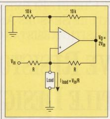
2. ANOTHER circuit example based on negative-resistor concepts is the familiar Howland current pump. The circuit functions as a V-I converter.
