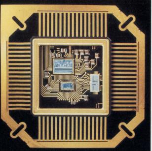
**1. PARTITIONING THIS DAC** into three chips allows it clock out 12-bit words at 500 MHz, making it useful for direct digital synthesis of arbitrary waveforms. The three chips forming Burr-Brown's DAC650 are a GaAs IC that provides the speed (lower left), and a silicon IC and a thin-film nichrome-resistor device that supplies the precision and accuracy (upper left, and right, respectively). The entire circuit is housed in a 68-pin surface-mount package with gull-wing leads.
