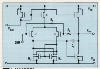
8. MOSFETS  $M_3$  AND  $M_4$ , called MAGFETs, have magnetic-field sensitivity an order-of-magnitude greater than Hall-effect sensors. The devices, developed at Ireland's NMRC, modulate the op amp's offset voltage.
