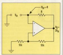
3. TRY THIS circuit when a negative resistor needs to be driven from a source impedance greater than R. The topology is similar to that of Figure 1, except that op-amp input terminals are interchanged to maintain a net negative feedback.
