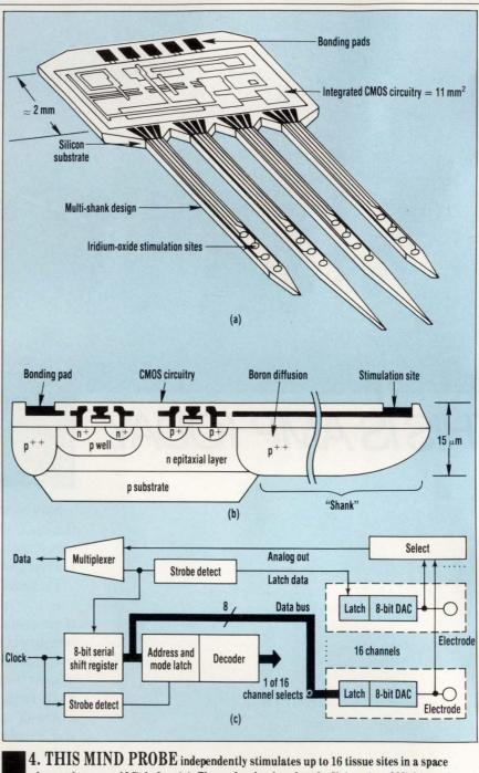
where only one could fit before (a). The probe, developed at the University of Michigan, is built on a CMOS process (b). Micromachining was added to the process to build the 15- $\mu$ m thick "shanks"(c). The active circuit contains 16, 8-bit DACs.
