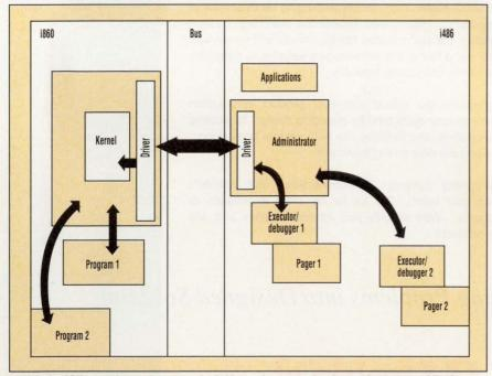
5. With the APX operating environment, the i486 runs its conventional operating system while the i860 operates under the APX kernel. The host executive communicates with the APX kernel to create new processes for the i860 when needed.
