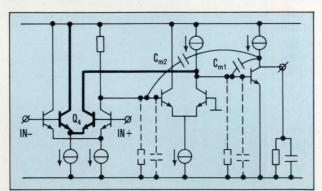
**9.** ADDING FEED-FORWARD circuit Q<sub>4</sub> to a "nested Miller" integrator compensation circuit for a three-stage op amp results in bandwidth that's equal to a two-stage op amp, without loss of open-loop gain (from Delft University).
