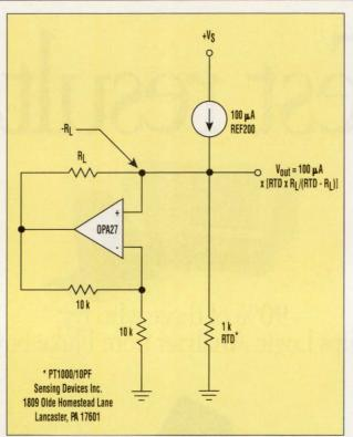
4. A GOOD WAY TO LINEARIZE a platinum RTD is paralleling it with a negative resistor. The value of negative resistance required is determined by the temperature range of interest. solve for R<sub>G</sub>.
