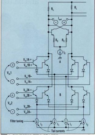
6. BY USING TWO STAGES (A and B) instead of one, and by adding the currents of the two stages, the dynamic range of Silicon Systems' transconductance amplifier for  $G_m/C$  filters was raised by a factor of three. Signal-to-noise ratio was increased by a factor of 2.4.
