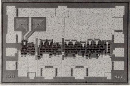
4. HIGH-FREQUENCY PERFORMANCE of NEC's silicon-bipolar frequency divider is enhanced by the spiral inductors in series with the load resistors of the Gilbert multiplier, which comprises the dynamic first stage. The inductors, shown above the first stage at left, increase the maximum frequency by 7% over that of a conventional circuit.
