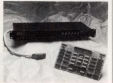
puts or outputs in 8-bit multiples. Each 40-line channel has six handshake lines: trigger, data strobe, inhibit, clear output, service request, and external data ready. An optional HVCX1 daughter board allows each port to control 200mA open-collector drivers. The option also makes the interface compatible with 12-, 24-, and 48-V logic when the unit is used with non-TTL devices. The Digital488/80A costs \$995 and the
