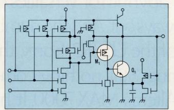
3. A QUASICOMPLEMENTARY biCMOS structure, demonstrated by this three-input NAND gate designed by Hitachi, can operate at twice the speed of similar CMOS circuits when either is powered by 3.3 V. The PMOS device  $(M_1)$  drives the base of the pull-down npn bipolar transistor  $(Q_1)$ , improving the gate speed.
