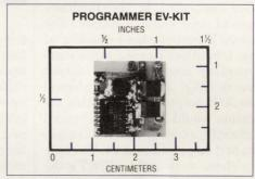
The complete surface mount MAX732 flash memory programmer fits into less than  $1/2 \text{ in}^2$  (3.2 cm<sup>2</sup>). Additional capacitors can be added for higher current operation — up to 200mA.
