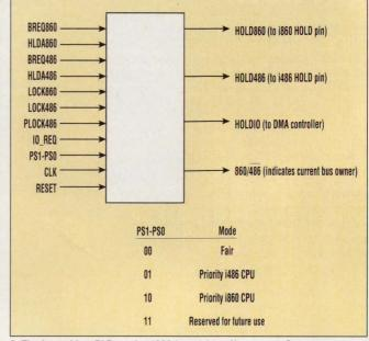
3. The bus arbiter PLD on the 4860 board from Hauppauge Computer Works uses the HOLD and HLDA pins to implement three bus access modes: Priority i486, Priority i860, and Fair.
