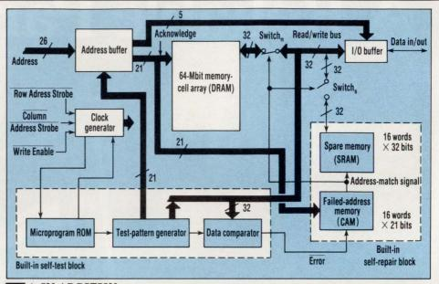
4. IN ADDITION to incorporating on-chip self-test circuits, a 64-Mbit DRAM developed by NEC includes spare memory cells that can be switched in if the self-test block detects any failed bits. When a failed DRAM bit is detected, the error signal generated by the data comparator activates the match line in the failed address memory. That line then activates the spare memory cells whenever the address for the defective cells is sent to the main DRAM array.
