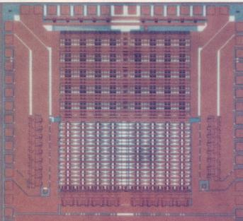
1. THE CROSSPOINT SWITCH CHIP from IBM contains about 4200 transistors and measures 3 mm on a side. The chip has 64 pads, 20 of which are used for the +1.4-V and -2.2-V power supplies and ground. The 16-by-16 switch multiplexers and outputs are located on the lower part of the die. The setup circuits with latches sit on the upper part.
