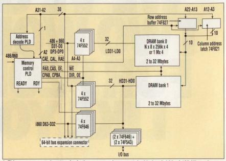
4. This memory control system for both processors h<u>as</u> a sustainable bandwidth of 133 Mbytes/s at 33 MHz. It pipelines i860 XR accesses by activating  $\overline{NA}$  when it latches address and control lines.
