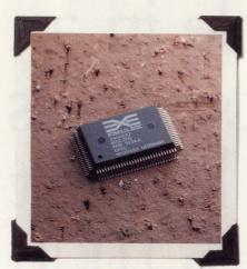
1988-MAC 200. Our advanced merged architecture controller is the first to include an automatic Data Flow feature for faster clata handling.
