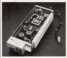
channels and latches itself off if any voltage is out of specification (high or low), if output currents exceed ratings, or if an overtemperature condition occurs. Pricing is \$259 in lots of 1000. Large lots are delivered in 16 weeks.
