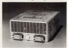
er features built-in 0.99 power-factor correction. With nominal inputs of 170 to 264 V ac, outputs can be configured from 310 to 380 V dc. The converter measures 4 by 8 by 11 in. and weighs 10 lbs. Unit price is \$895. Call for delivery information.
