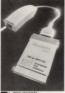
**1. THE MODEM** 2400 + fits in a PCMCIA Type II package (5-mm thick). The 2400-baud modem, from Intel, is compatible with the PCMCIA Release 2.0 specification, as well as the company's ExCA standard. No external power is needed to run the modem.
