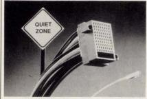
The Quiet Zone SC modular coaxial cable assemblies offer the highest signal fidelity available in 0.025-in. square post packages. Over 90% V<sub>p</sub> signal speeds and 0.5% crosstalk at sub-nanosecond rise times is featured. A patented 360° shielding technique completely shields the signal line, both within the cable and through the connector. This keeps insertion loss to around 2 dB at 1 GHz for 10-ft lengths. Call for pricing.
