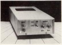
A line of ruggedized ac-dc conditioned power sources is well suited for use with distributed-power dc-dc converters and systems. The PB Series is available with single- or threephase ac input and dc outputs from 24 to 300 V, including 28, 48, 155, and 270 V. True N+1 current sharing as well as 0.99 power-factor correction is featured. Call for pricing and delivery.
