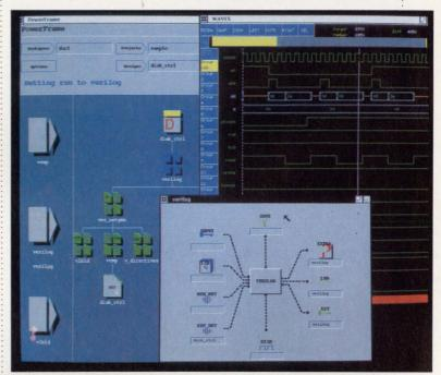
3. By exploiting the windowing power of modern workstations, PowerFrame displays the design environment and the work in progress. Tools are selected and run simply by pointing at their icon.
