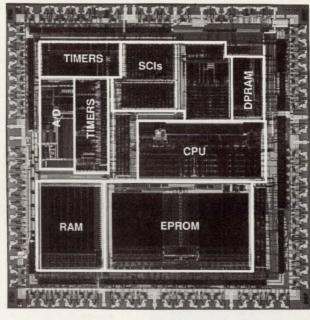
ing the ADC, some I/O lines, and adding a second serial port and a choice of 20 interrupt sources turns the 330 series of microcontrollers into the 320 series. The 320 series of microcontrollers can find a variety of homes in real-time control, office automation, and mobile-communications hardware.
