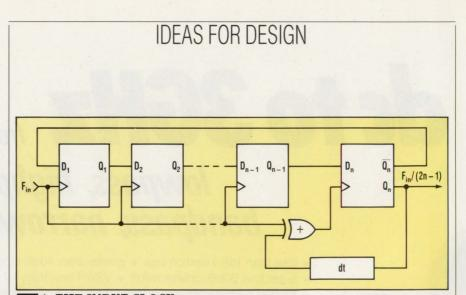
1. THE INPUT CLOCK frequency fed into this circuit is divided by 2n - 1. The circuit consists of n clocked flip-flops and one exclusive-OR gate. The dt delay is zero in most cases.
