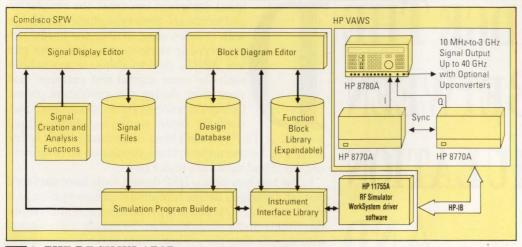
2. THE RF SIMULATOR worksystem consists of the Comdisco Signal Processing WorkSystem tightly integrated with two HP 8770A Arbitrary Waveform Synthesizers, each with a 50-MHz baseband bandwidth. The synthesizers drive the I and Q modulation inputs of an HP 8780A Vector Signal Generator.
