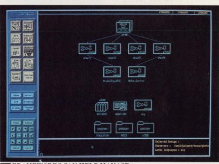
FRAMEWORKS CAN HELP MANAGE both tools and data. Computervision's Design Desk Framework is an open environment that provides intertool communications and file management. Users can integrate Computervision applications, third-party tools, and their own internally developed software.
