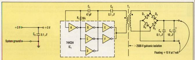
THIS COST-EFFECTIVE CIRCUIT is a dc power supply isolated to  $\pm 2500$ -V. Because none of the circuit's components (except for the transformer T<sub>1</sub>) see the full  $\pm 2500$  V, expensive high-voltage parts are not needed.
