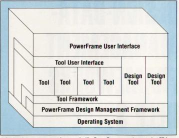
1. Design-data-management frameworks like PowerFrame complement what EDA frameworks can do. PowerFrame brings together applications, design-data management, and design-process management under a consistent graphical user interface across disciplines such as ECAD, MCAD, embedded CASE, and documentation.
