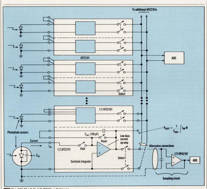
EACH HALF OF THE AFC2101 dual switched integrator converts currents, from a few picoamperes to tens of microamperes, to a voltage. This is done by integrating the current on the chip's 100-pF oxide capacitor. Logic inputs (not shown) control the on-chip hold, reset, and select analog switches.
