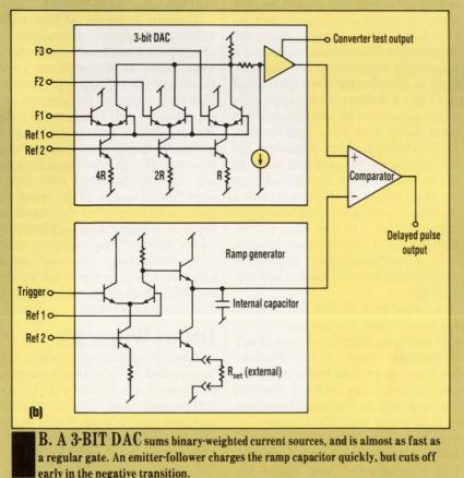
source has a very low temperature coefficient with respect to the negative supply. In this way, if a resistor with a low temperature coefficient is used to set the current, then the overall delay span will display good temperature stability.
