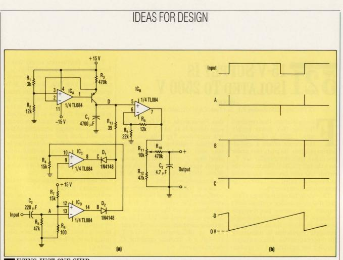
USING JUST ONE CHIP (a TL084), this circuit converts an input signal's period to a dc voltage. Then the period can be measured with a multimeter. The circuit's measurement range is from 100  $\mu$ s to 5 ms (a). The waveforms show what's happening at different points in the circuit (b).
