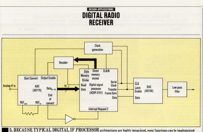
in the DSP software. In this example circuit, only a few ICs are needed to perform the functions, as described in Figure 4.
