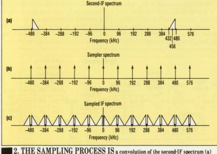
with the sampler spectrum (b). The resulting spectrum shows that if the second-IF bandwidth is increased, aliasing distortion will occur (c).
