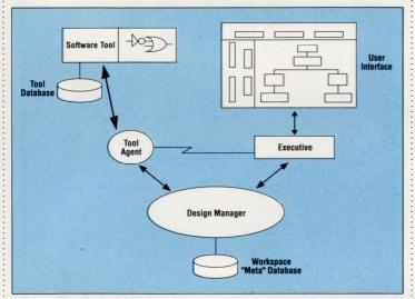
2. PowerFrame is made up of a set of functional components. The Design Manager Server maintains an active meta database, called a workspace, that tracks design, library, and tool data. The PowerFrame Executive, which is the graphical interface to the system, provides a straightforward method for invoking tools and displaying design, library, and tool data.
