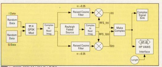
4. THE SIX MAIN PARTS of a single-ray model in a cellular faded channel simulation are (from left to right): a digital source of data, a modulator, the required I and Q Nyquist filtering, a source of Rayleigh distributed signals satisfying the model, mixers to combine the effects of fading on the modulated signal, and the HP VAWS interface block.
