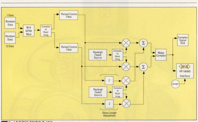
9. ADDING MORE RAYS to the single-ray model causes the received signal to contain delayed and faded versions of the transmitted signal. These added rays are needed to model a received signal in a typical environment with several far and near reflectors.
