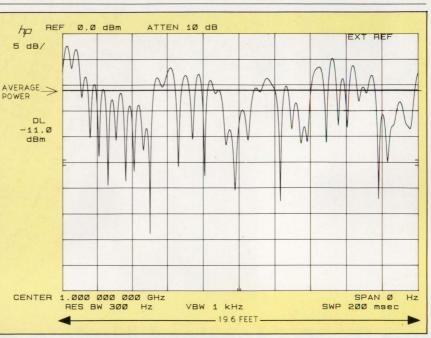
6. THE VAWS CHANNEL SIMULATOR OUTPUT is the signal envelope power over time. Fades and peaks occur with reference to the average power. Fdoppler = 100 Hz (67 m.p.h.), and the signal power is measured over a distance of 19.6 ft.
