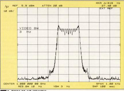
5. THIS PLOT SHOWS the signature spectrum of the channel simulator with a 100-Hz Fdoppler. The modulator was disabled for this signal. As expected, the power spectral density has the "smile" shape.
