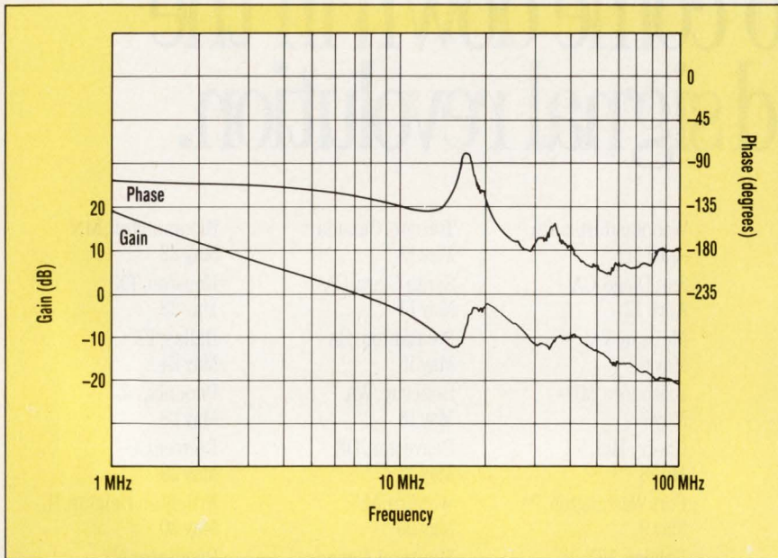
5. THE RESONANCES SEEN by the supply pins of an op amp translate into rapid changes in op-amp gain and phase with an attendant loss in phase margin and increased potential for oscillation. The effect is shown here at 16 MHz.
