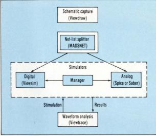
2. "NETWORK-SPLITTER" software is used in glued mixed-signal simulators, such as Viewsim/AD from VIEWlogic. The splitter sends digital models to a digital simulator and analog models to a circuit simulator. Models tagged for a simulator are available in the frameworks library. Designers can tag them at the schematic-capture stage.
