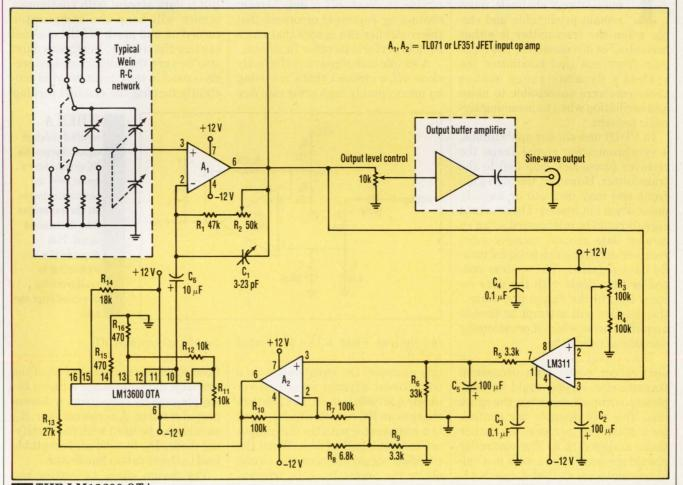
THE LM13600 OTA, connected as a variable resistance in the negative feedback loop of a Wein Bridge oscillator, stabilizes the output. This serves to eliminate amplitude variations as the frequency is changed.
