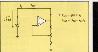
1. THIS circuit derives reference voltages not readily acquired by common reference ICs. But, because the Zener voltage is toleranced at  $\pm$ 5%, a gain adjustment is needed to get the exact reference voltage.
