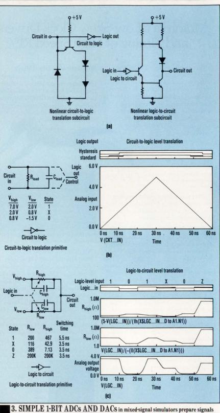
5. SIMPLE PD11 ADUS AND DAUS in mixed-signal simulators prepare signals for alternative forms of processing. Called "circuit-to-logic" and "logic-to-circuit" translators by MicroSim, they may contain active, nonlinear elements (a). They may also be simple primitives (b and c). However, even in the latter two cases, the effects of resistance and capacitance are considered when handling, or creating, real-world waveforms.
