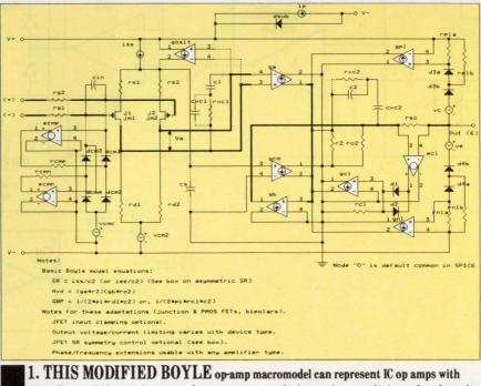
virtually any differential transconductance stage on the input. As a result, it can be adapted for op amps with npn, pnp, JFET or MOSFET input stages.
