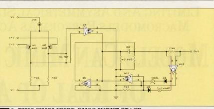
2. THIS SIMPLIFIED PMOS-INPUT-STAGE op-amp macromodel provides accurate simulation of op amps with dissimiliar output current sink-to-source ratios.
