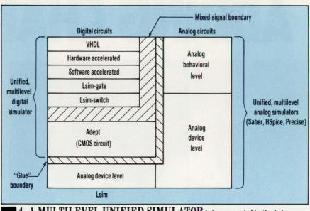
4. A MULTILEVEL UNIFIED SIMULATOR is incorporated in the Lsim mixed-signal tool within a glued simulator. The mixed-signal boundary may be crossed vertically while simulating digital circuits, or horizontally to handle analog circuits.
