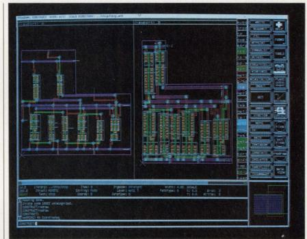
THE DEVICE-LEVEL COMPACTOR in Construct P.I. is the essential element in process-independent IC design. The compactor references the technology database to shrink or expand all layers of the layout while keeping design-rule correctness. In this screen, the compacted layout is in the right window.
