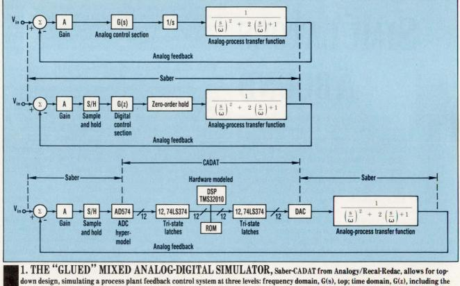
acquisition and processing of sampled data, center; and circuit level (bottom). At the circuit level, the TMS32010 digital signal processor is operated within a hardware modeler.
