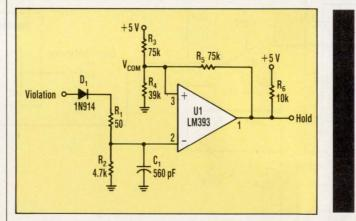
the figure). First, a line associated with decode violations is rectified. In this example, the violation pin on a transparent asynchronous receiver (AMD AM7969) is used. The line then charges an RC circuit, which is input to a comparator with the other input set to about half of  $V_{\rm CC}$ . When the rectified signal charges the circuit above the preset level,  $U_1$  triggers and generates a low signal that masks off the received signal.
