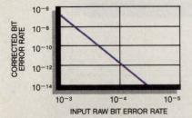
Corrected Bit Error Rate vs. Input Raw Bit Error Rate for random bit errors. Code: RS (72,62) corrects 5 errors.
