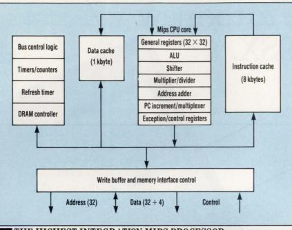
THE HIGHEST-INTEGRATION MIPS PROCESSOR from LSI Logic packs 8 kbytes of instruction cache, 1 kbyte of data cache, a DRAM controller, and three counter-timers. The chip's features let the processor tackle demanding control applications.
