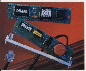
Plug 'n' Go Telephony: The FCC-certified DS2245 Soft Modem and the DS2249 DAA offer the AT command set, DTMF decoding, and direct connection to the public telephone network.
