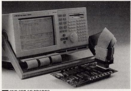
ONE SET OF PROBES, attached with quick-connect adapters, acquires both state and timing data on the PM 3580-series logic analyzers. Users can display both sets of data on the widowed interface.
