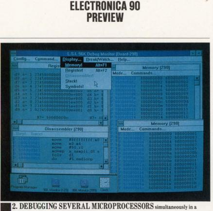
2. DEBUGGING SEVERAL MICROPROCESSORS simultaneously in a multiprocessor system (each with its own window) is possible with the DSP96002 DSP board from Loughborough Sound Images. Register, disassembler, and memory activity can all be displayed at the same time to ease software development.
