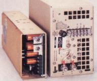
Designed for high-end computer products, TODD's MAX-750 combines a compact size, 13.5" x 5" x 2.6" compared to the typical 5" x 8" x 11" shoebox switcher (see photo insert), and very competitive pricing. OEM product designers can reduce product size with a MAX-750 or build in power supply redundancy, replacing one "shoebox" switcher with two MAX-750's in the same space.
