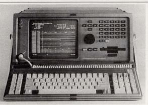
2. IN ADDITION TO OFFERING up to 192 channels, the PLA/2 portable logic analyzer from Kontron holds a complete PC/AT-compatible host computer. The 3.5-in. floppy drive and a 25-Mbyte hard disk are standard.
