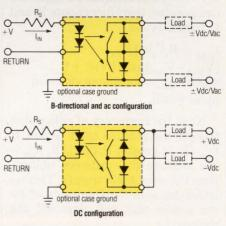
tes: 1. A series resistor is required to limit continuous input current to 50mA (peak current can be higher).
