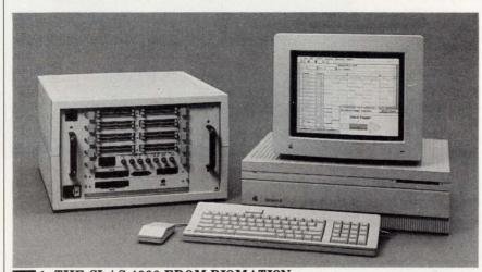
1. THE CLAS 4000 FROM BIOMATION (left) is hosted by a Macintosh II computer. The analyzer mainframe can hold up to four 96-channel cards, which can be used as one 394-channel instrument or four separate units.
