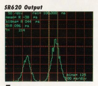
The SR620 brings graphic statistical analysis to time interval and frequency measurements. The SR620 shows you more than just the mean and standard deviation - multimode frequency distributions or systematic drift for example. Histograms or time variation plots are displayed on any X-Y oscilloscope, complete with Autoscale, Zoom, and Cursor functions. Hardcopy to plotters or printers is as easy as pushing a button.
