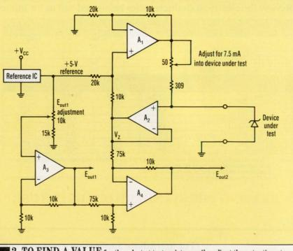
2. TO FIND A VALUE for the select-at-test resistor easily, adjust the potentiometer so that  $E_{out1}$  equals the  $V_{REF}$  from the first circuit. Then measure  $E_{out2}$ . This number, in millivolts, is equal to  $R_{SAT}$  in ohms.
