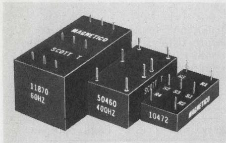
**Scott T Transformer.** 11870: 60HZ, 90v, L-L in. 1.1x2.1x1.1. 50460: 400 HZ, 90v, L-L in. 7/8x1-5/8x11/16. 50642: 400HZ, 11.8v, L-L in. 7/8x5/8-11/16. 10472: 400-HZ, 11.8v, L-L in. 3/4x1-1/2x3/8. All with 6v RMS sine & cosine output. MAGNETICO, INC., 182 Morris Ave., Holtsville, N.Y. 11742 516-654-1166.
