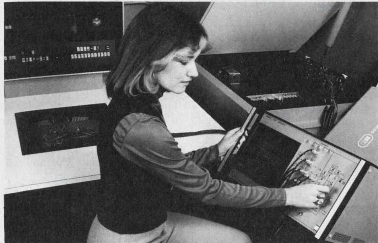
By now almost everyone agrees that the conventional oscilloscope isn't the best tool for finding failures in digital systems. The old 'scopes have been superseded by logic analyzers—multichannel devices that observe a set of digital signals, trigger on a particular combination of them, and display a timing diagram or bit array that shows the events before and after the trigger.
