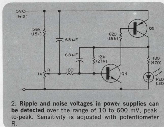
2. Ripple and noise voltages in power supplies can be detected over the range of 10 to 600 mV, peak-to-peak. Sensitivity is adjusted with potentiometer R.
