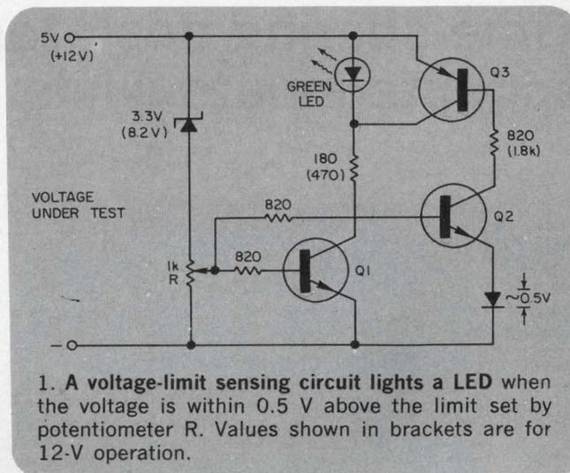
1. A voltage-limit sensing circuit lights a LED when the voltage is within 0.5 V above the limit set by potentiometer R. Values shown in brackets are for 12-V operation.
