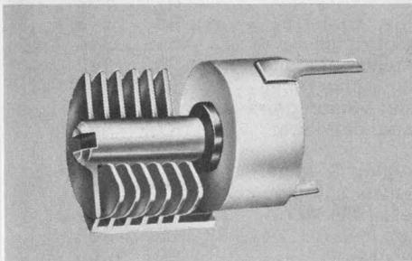
**High performance Type "T" sub-miniature machined-plate capacitors.** Rotors and stators machined from solid brass extrusions provide excellent stability and uniformity. High Q, low temp. coefficient (plus 30 ±ppm/°C). Available in horizontal and vertical tuning for PC and stripline mounts. E. F. Johnson Co., Waseca, MN., (507) 835-5222.
