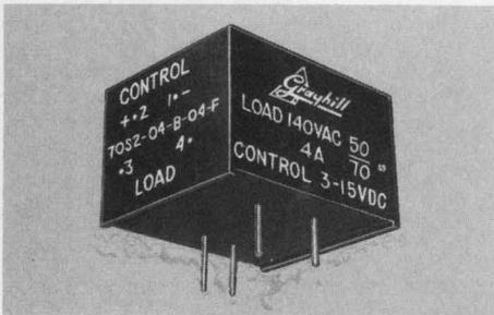
**SPACE-SAVING 4 AMP SOLID STATE RELAY** occupies only 1 cubic inch, is logic compatible, with switching capability from 0.1 to 4 amps, rated @25°C. Optically coupled; zero voltage turn-on. Offers inductive load switching, excellent transient protection. PC mountable. Prototype quantities from stock. Grayhill, Inc., (312) 354-1040.
