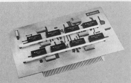
**EASIER ECL VOLTAGE AND GROUND DISTRIBUTION SYSTEMS**—Reduced system noise, high packaging density and less design time for PC boards with ECL circuits are yours with Mini/Bus®, the Rogers way to eliminate the cost of multi-layer boards by off-board voltage and ground distribution. Rogers Corp., Chandler, AZ 85224 (602) 963-4584.
