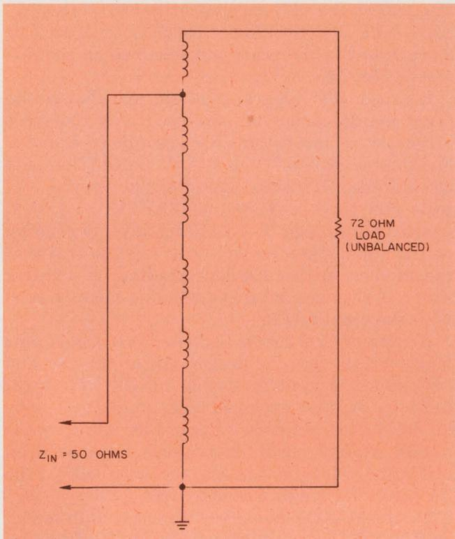
9. A hexafilar winding is used in this example to match a 72-Ω load to a 50-Ω cable.
