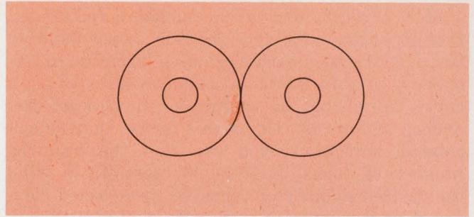
13. Two toroidal cores placed side by side offer a better form factor than a simple toroid.
