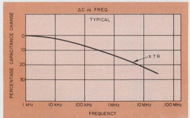
**5. Electrical characteristics for Class II capacitors** vary widely with temperature, offered voltage and frequency.
