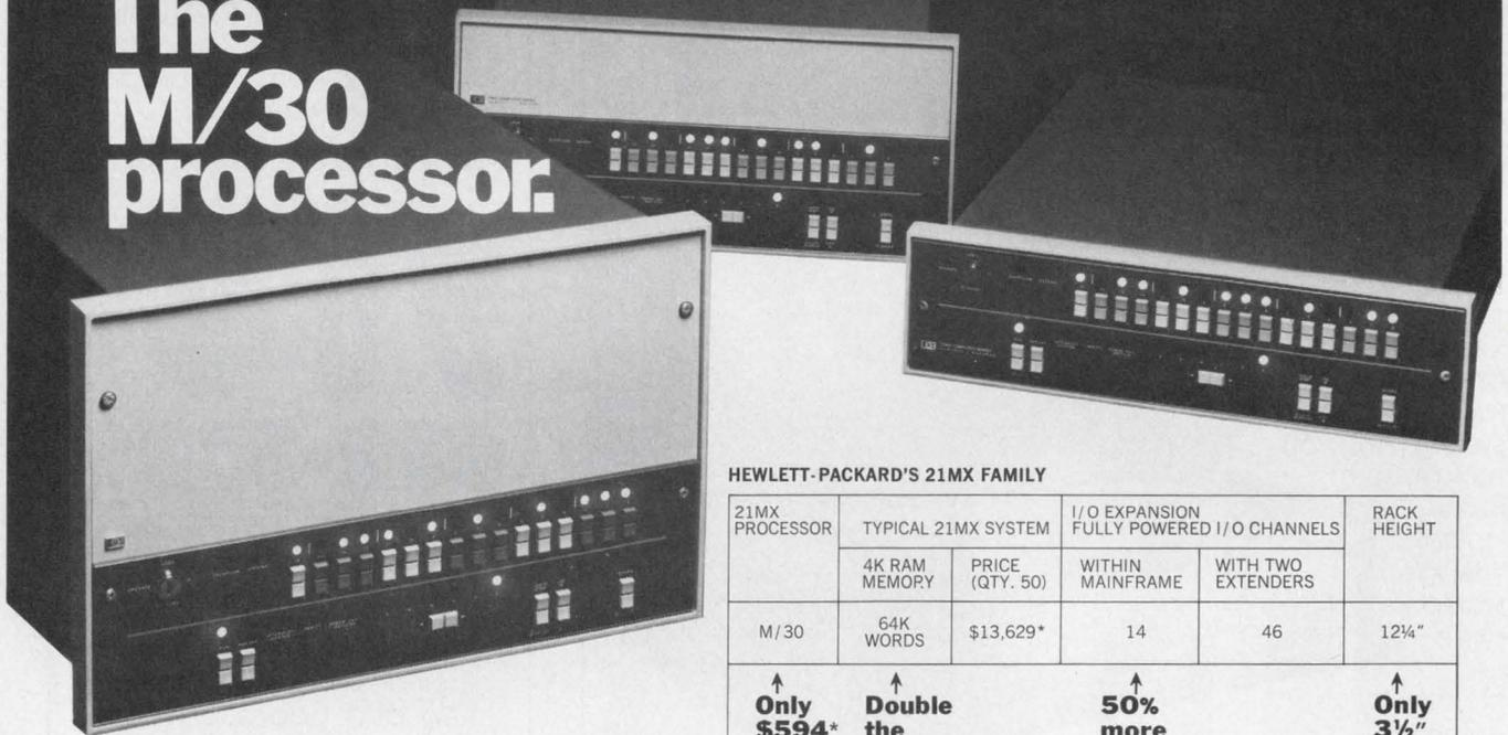
Now Hewlett-Packard brings 4K RAM semiconductor technology to OEM's with large memory needs. Compatible with all previous 21MX minicomputers, the new M/30 offers the same modularity, the same flexible user microprogrammability.
