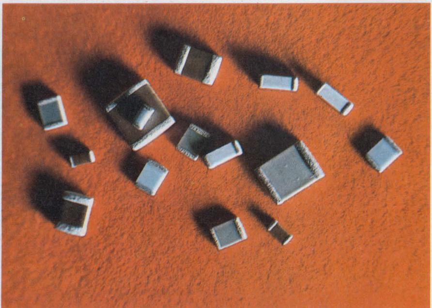
**Ceramic chip capacitors** in various sizes, including these from USCC/Centrolab, range in value from 0.1pF to over 200  $\mu\text{F}$ . Ratings are from 4 to 200 V.
