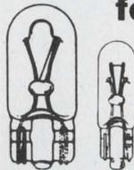
Now you can have greater design freedom than ever before with wedge base lamps. GE now offers six large lamps in its line of T-1 $\frac{3}{4}$  (.230" max.) all-glass, sub-miniature wedge base lamps. In addition to our three 14V lamps (#37, #73 and #74), we now also offer two 6.3V lamps (#84 and #86) and a 28V lamp (#85).
