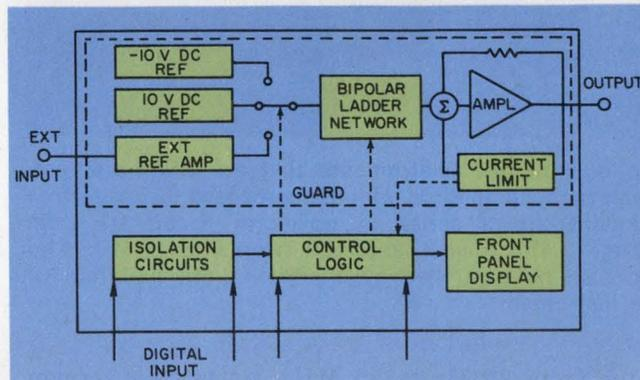
Fluke's programmable power DAC uses a bipolar ladder network digital-to-analog converter, connected through a power amplifier, to provide precision programmable power. Outputs are available at 65 V and 110 V.
