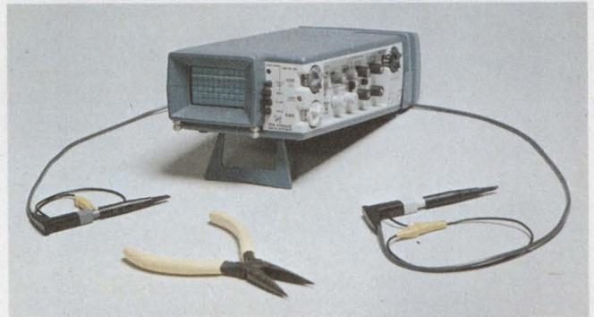
change too slowly to be seen as waveforms on regular CROs (Fig. 3). Such signals are not at all uncommon in mechanical systems and in transducer-based applications, where standard CROs can't meet the measurement demands. The auto makers, for example, are one of the largest users of storage CROs, with most of their applications involving mechanically generated signals.
