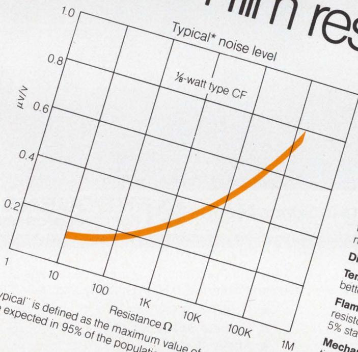
\*"Typical" is defined as the maximum value of measurement unit to be expected in 95% of the population of a distribution.
