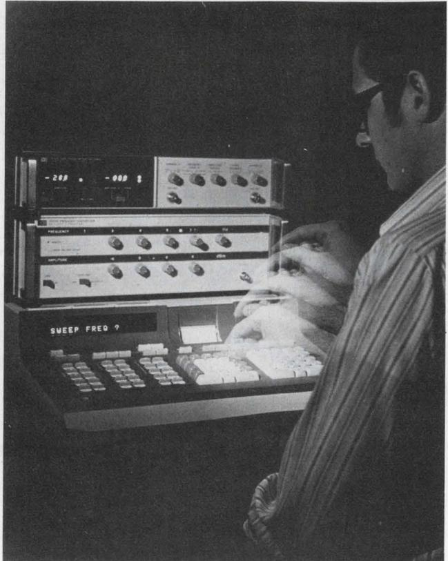
1. Systems using calculators can take data from a variety of instruments, process the data and output the results to an assortment of peripherals.
