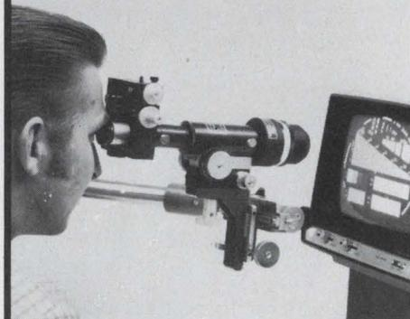
A work horse when it comes to measuring the output characteristics of electronic displays; that's the Gamma Scientific Model 2900MR Scanning Microphotometer System.
