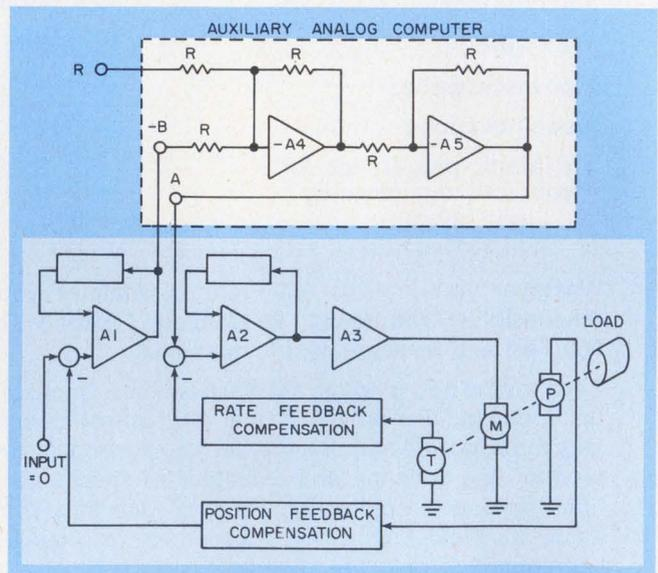
2. **To measure open-loop (and closed-loop) response** with the loop closed, a break is made at the summing junction between amplifiers A<sub>1</sub> and A<sub>2</sub>, and an auxiliary computing chain is inserted at the break. With zero reference signal, the servo-loop gain remains unchanged.
