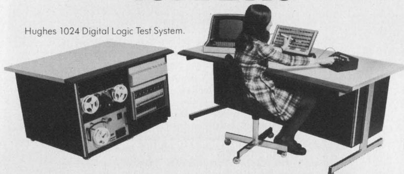
Hughes 1024 Digital Logic Test System answers yes to all the questions above. It also provides an optional simulation system, Digital Fault Analysis (DFA), which generates a logic model; simulates the unit under test; verifies using fault insertion techniques; and generates fault isolation data for the automatic guided probe. Time independent gate level simulation identifies "race" conditions and traces them to their origin.
