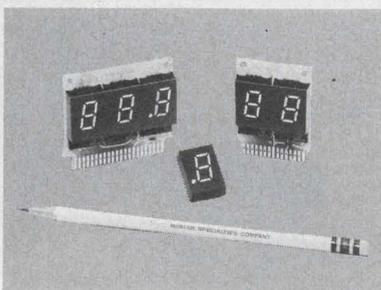
Plug-in LED Display Assemblies with decoder/driver circuits already assembled, ready to plug-in and read-out. Accepts 4-line BCD input. Operates from 5 VDC. Utilizes 0.6" high red numeric LED display. Master Specialties, 1640 Monrovia, Costa Mesa, Calif. 92627. (714) 642-2427.
