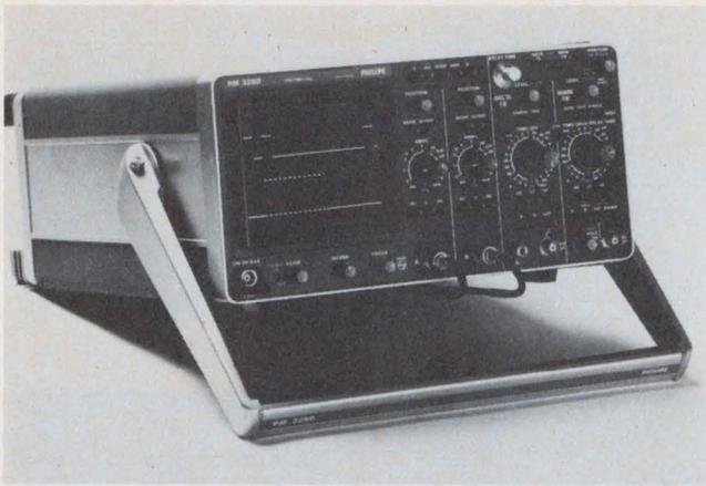
Phillip's PM 3260 120-MHz oscilloscope has a very clear and uncluttered, easily used control panel. Cold switching enables the designer to place the controls for best layout.
