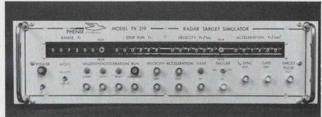
A simulator for radar range provides a target pulse at a precise time after a trigger pulse. The output pulse is controlled to simulate target velocity and range. Model PX 219 provides use times under 5  $\mu$ s for a 400- $\mu$ s target pulse. The PX 219 from Phenix Electronics can be programmed remotely.
