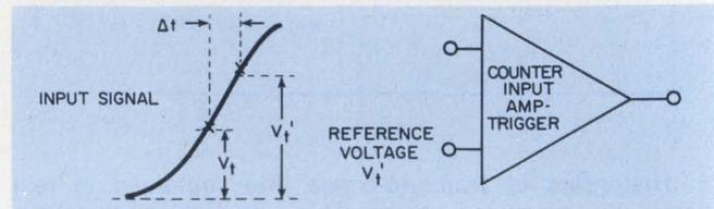
6. Setting reference voltage  $V_t'$  via the counter trigger-level control establishes the voltage level,  $V_t$ , of the input signal at which the counter triggers.
