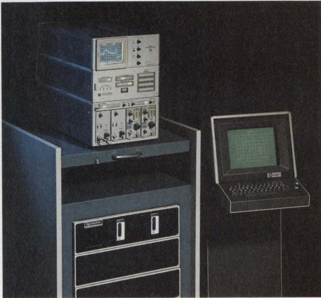
Available storage oscilloscopes today range from a 3.7-pound, battery-powered, bistable miniscope (below) to a sophisticated digital-processing unit (left). The miniscope will hold a signal for hours so that you can bring the unit to the job and even carry the trace home. With the digital system you can calculate data and hook up a computer for further analysis.
