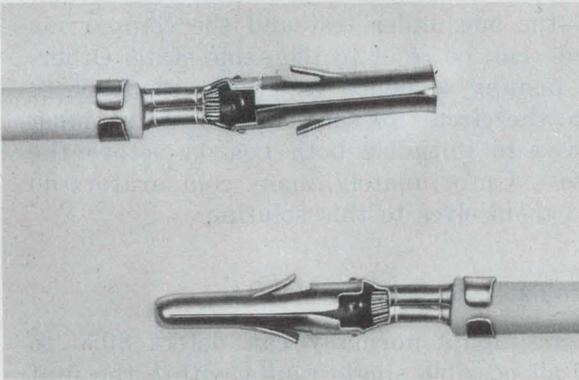
cover the full range of wire sizes. Number 24 to 16 AWG and .040" to .130" insulation diameter. They also feature serrated wire barrels to break up surface oxides and a stepped insulation barrel to keep the conductors in perfect alignment with the contacts.
