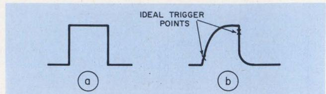
5. Triggering on the fastest portions of a signal waveform minimizes measurement error. Input signal "a" appears as "b" at the input amplifiers.
