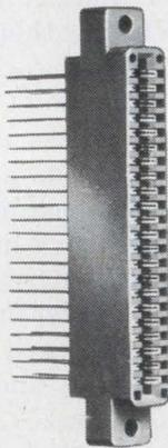
Continental's continuous process selective plating deposits an equal amount of gold on each contact. The contacts pass through various cleaning and plating baths, resulting in a controlled amount of gold uniformly deposited on the critical contact area.
