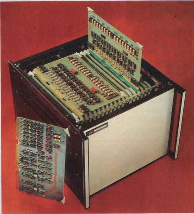
The E-H 1604 word generator generates simultaneous pulses for up to 48 pins (at rates to 20 MHz) and compares the measured output with expected levels stored in its own memory. Each pin can provide 512 bits. And all the parameters on this device are programmable.
