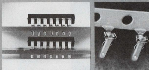
For use where space is restricted; extends just .030" above and .088" below board, allows .400" board-to-board spacing. One size MINISERT<sup>®</sup> socket fits wide range of hole sizes—.050" to .058" in diameter. RTV diaphragm seals foreign matter out of the socket. MINISERT socket accepts round or flat leads of DIP's, LED's and LSI's. Free-standing design can be used in any socket pattern. Semi-automatic machine inserts at rates up to 2000 per hour. Write for Bulletin 120, or call:
