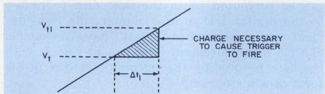
8. Although charge starts to accumulate at  $V_t$ , triggering does not occur until  $V_{t1}$ , when the input signal has a high slew rate.
