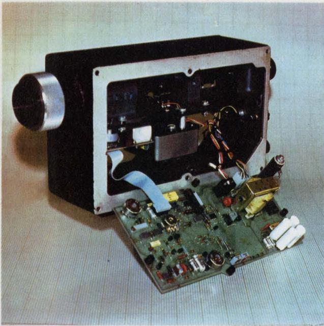
Infrared thermometer from E<sup>2</sup> Thermodot of Carpinteria, CA, measures temperature by optically sensing the intensity of radiant energy emitted by a warm surface.
