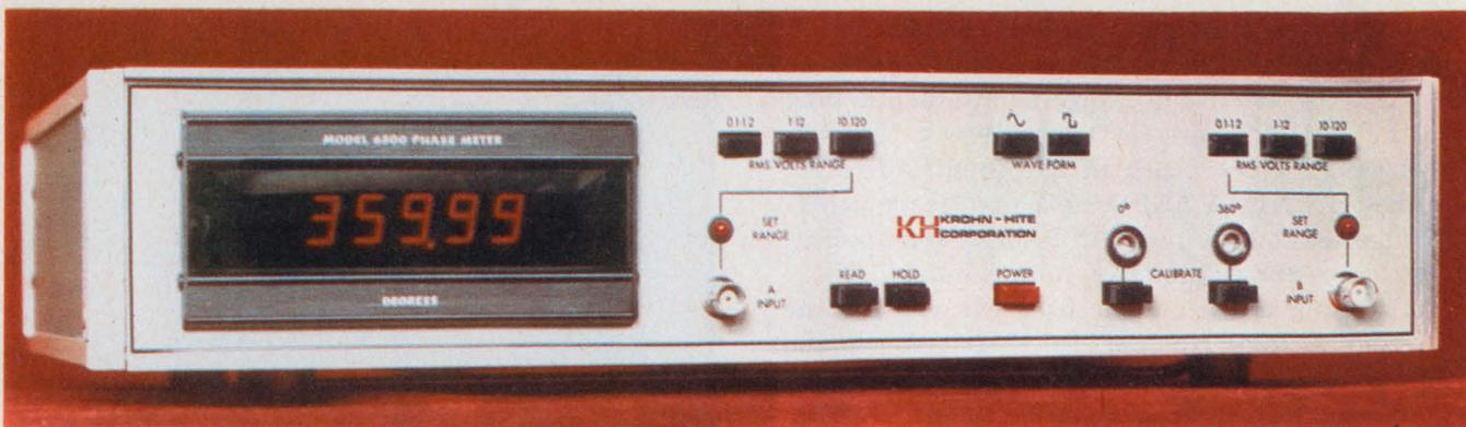
The 6500 digital phasemeter from Krohn-Hite features an accuracy of  $0.05^\circ$  with a  $0.01^\circ$  resolution. The fre-
