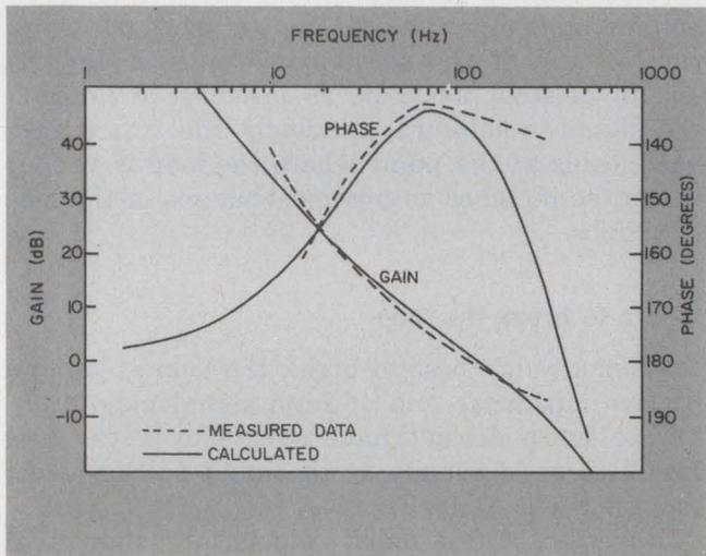
6. **Open-loop response of the bearing-torque tester:** Measured gain and phase agree closely with the calculated data for the frequencies of interest.
