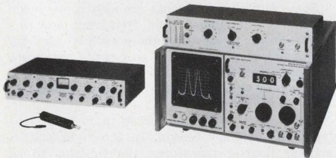
Communications signal analysis is the forte of this unit, the Nelson-Ross CSA-290. The 43-MHz analyzer can handle inputs to 400 MHz with a range extender.
