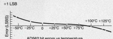
AD562 bit errors vs temperature.
