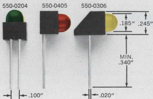
Mix 'em or match 'em. LED logic state fault indicators are available in red, yellow and green, in a variety of shapes, some with a built-in integral resistor. Can be driven from DTL and TTL logic. Designed for easy alignment on PC boards so that multiple functions can be displayed.
