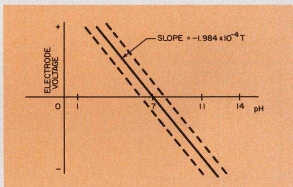
In a neutral solution—one that is neither acidic nor basic—the pH is 7.0 at 25 C. This decreases for acidic solutions and increases for basic solutions. Each unit change in pH number represents a tenfold change in hydrogen-ion activity,  $a_{\text{H}}$ , which is related to the concentration of hydrogen ions in a solution—specifically  $\text{pH} = -\log a_{\text{H}}$ .
