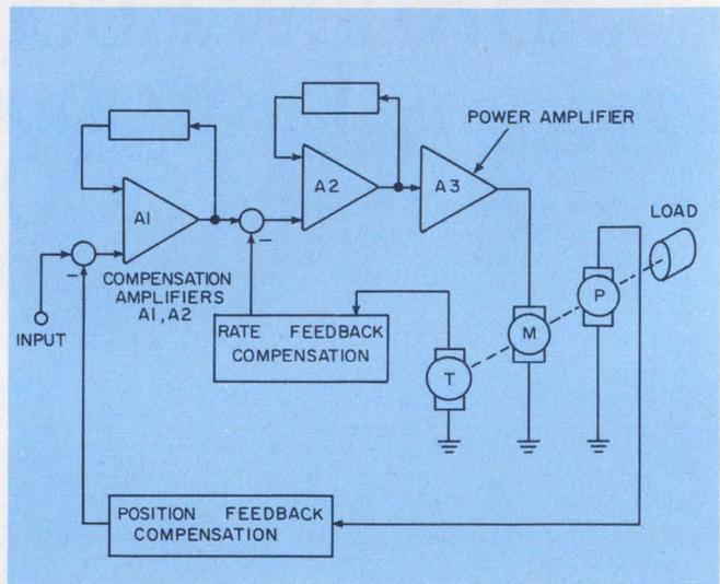
1. **Typical position servo** has two feedback loops: one to carry back the load position and the other to adjust the servo damping. When the main loop is broken at any point, one of the servo amplifiers usually saturates, which makes measurements impossible.
