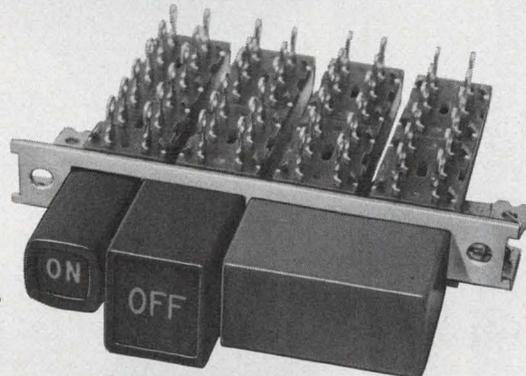
applications, specify a DW Power Module—one per station maximum. Turret terminals are brass with tin-lead coating. The snap-action switch is Form 1-C rated at 11 amps, and is U.L. and C.S.A. listed. The mounting brackets and insulating shields are designed to meet those same requirements.
