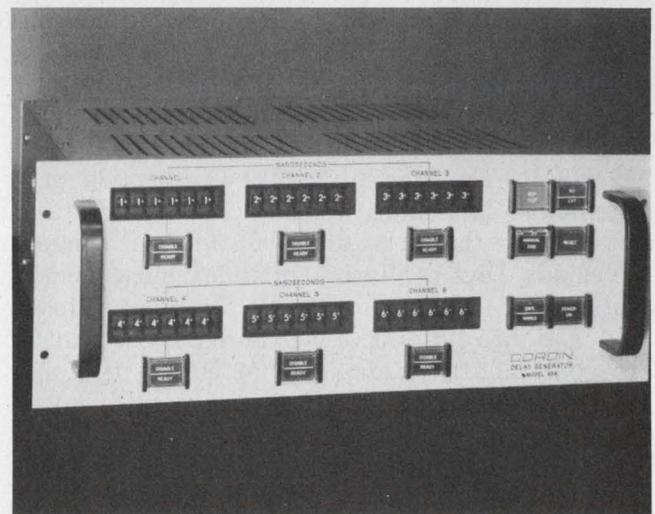
Time-delay generators provide delayed triggers calibrated to nanosecond increments. The Model 438 from Cordin (right) provides delay from 0 to 999.999  $\mu$ s with outputs to 40 V into 50  $\Omega$ . Model 7030 (left), part of Berkeley Nucleonics modular system, offers 1-ns increments to 100  $\mu$ s. These devices are often used in the operation of Image Converter Laser Diagnostic Cameras and flash X-ray analysis.
