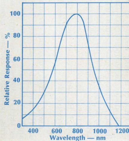
Standard Vactec phototransistors provide very high sensitivity and good blue response. Liberal design flexibility is also offered with trade-off for some characteristics, including: light current; response time; spectral sensitivity; and breakdown voltage. Selection of packages are TO-18, co-axial, pill, non-hermetic TO-18 size and special arrays on 50-mil or 25-mil centers.
