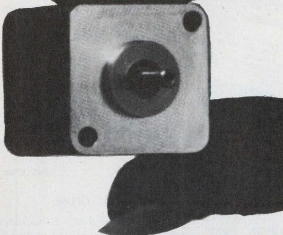
One cubic inch . . . that's all the space it needs. But it sends a strong, reliable signal up to 6.5 V/1000 RPM. Maximum deviation from linearity will not exceed 1% assuring high degree of accuracy. Low friction and rotor inertia will not load down equipment. Speeds to 5,000 RPM.
