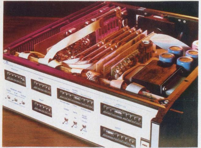
counted-burst option (\$300) enables the generator to output 1-to-9999 pulses on receipt of a trigger, and the same number of pulses occur regardless of the rep-rate setting.
