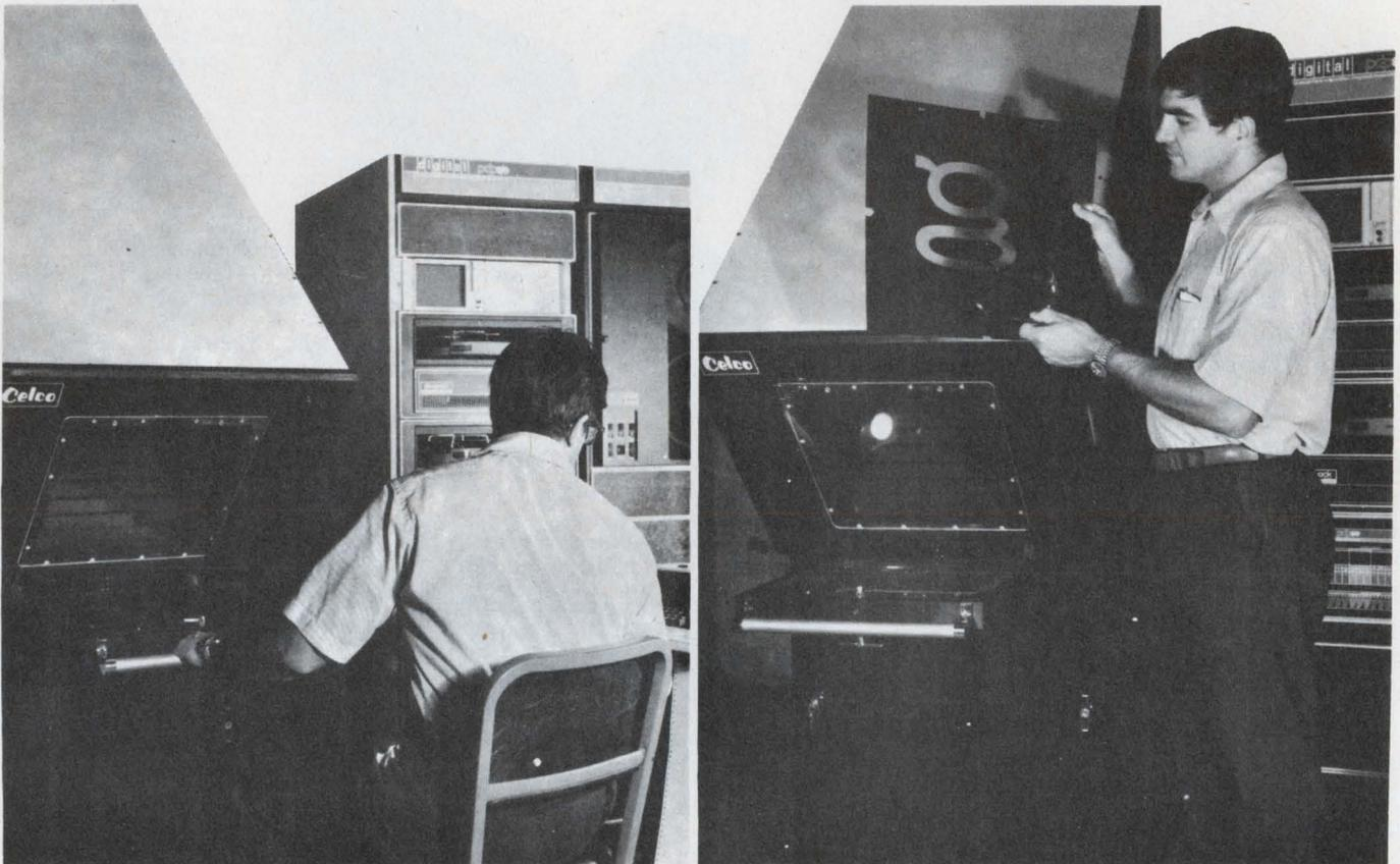
**CELCO's Large-Format Scanner is a unique solution for automating the production of master fonts for a manufacturer of computer typesetting equipment. Scanning a 16-million point area, this system calibrates itself and reduces an artwork master 14 inches x 14 inches to a digital record in 16 seconds.**
