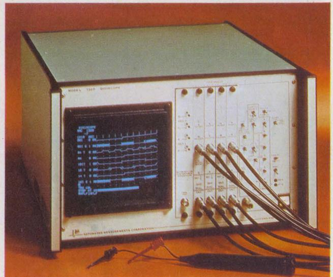
The AMC 1320 logic analyzer is capable of displaying the simultaneous time relationships of up to 8 parallel channels of data.
