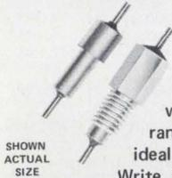
The combined technologies of SPECTRUM CONTROL, INC. and ALLEN-BRADLEY CO. have produced this exciting line of multi-layer feed-thru capacitors. Their tubular design and coaxial construction gives low inductance with capacitance values to 1 MF. The operating temperature range is -55°C to +125°C at 10 amps and 50 VDC. They are ideally suited for bypassing, filtering and coupling applications. Write today for our complete catalog.
