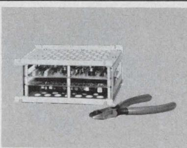
**Model MOD-815 A/D Converter.** Digital data with 8-bit resolution at any random or periodic word rate from DC through 15 MHz. Only 100 cu. in. Power dissipation approx. 20 watts. Computer Labs, 1109 S. Chapman St., Greensboro, N.C. 27403.
