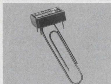
New low profile low cost TTL DIP Crystal Oscillator measures only 0.3" high x 0.49" w x 0.78" L; plugs into single IC socket; available at any fixed frequency from 4 MHz to 20 MHz, with frequency tolerance  $\pm 0.01\%$  from  $-25^{\circ}\text{C}$  to  $+75^{\circ}\text{C}$ ; fan-out 10 TTL. Supply 5 Vdc  $\pm 5\%$ . Connor-Winfield Corp., West Chicago, Ill. 60185 (312) 231-5270.
