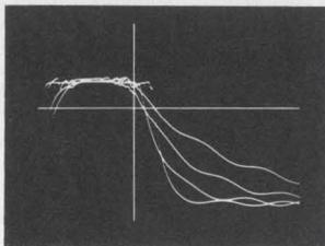
The 1090 offers numerical readout of any selected data point. Selection is made with an easily moved cursor. Wherever the vertical cursor intercepts the waveform the alphanumeric readout on the CRT displays time from trigger and voltage
