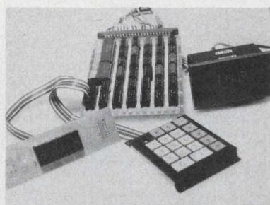
Calculator - BCD Interface. Complete 4 function calculator accepts up to 5 BCD decades from DVM, counter or keyboard. Outputs 7 segment info plus 8 decades BCD. Board TTL compatible - single 5V supply. Many options. \$365. unit quantity. Elcom Ind. Inc., Civil Air Terminal, Bedford, MA 01730 (617) 274-6656.
