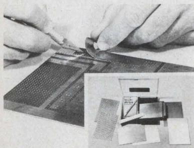
**Cut & Peel Circuit Board Kit.** Cut prototype boards or ground planes. Assortment of 7 includes one and two sided Cut & Peel Boards on .100" grid drilled and plain epoxy-glass, "X" and "X-Y" Board, a plug-in Cut & Peel GP Board with etched gold/nickel edge connector, and a special knife. Kit #8964 is \$37.00. Circuit-Stik, Inc. Box 3396, Torr., CA 90510.
