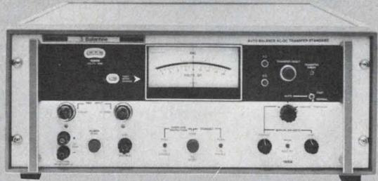
The 1600A Auto-Balance AC/DC Transfer Standard. Precise repeatable measurements every 30 seconds. Traceable to NBS. Takes tedium and guesswork out of 100 ppm transfer measurements in Lab, QA and production.
