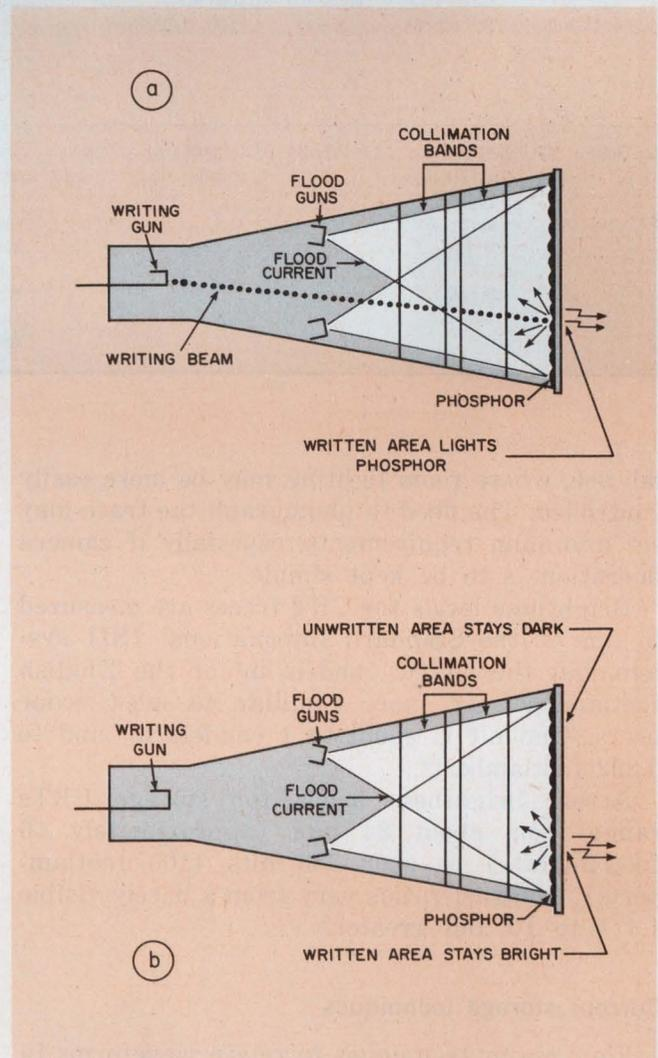
5. In bistable storage, the writing beam traces the waveform on a target (a). Flood guns reinforce the written portions to keep those areas bright (b).
