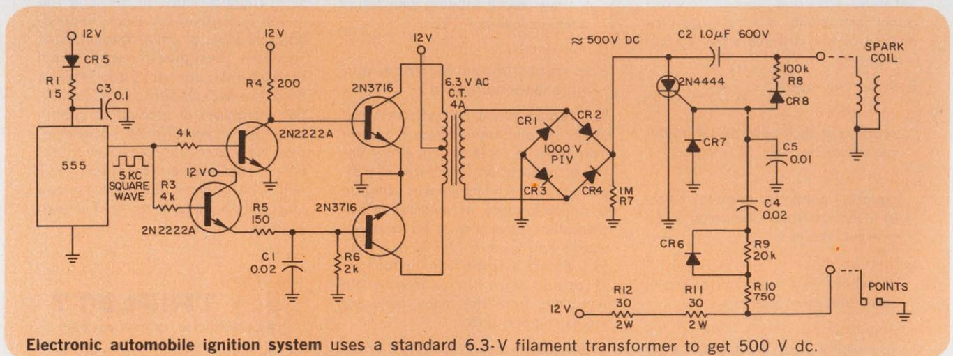
Electronic automobile ignition system uses a standard 6.3-V filament transformer to get 500 V dc.
