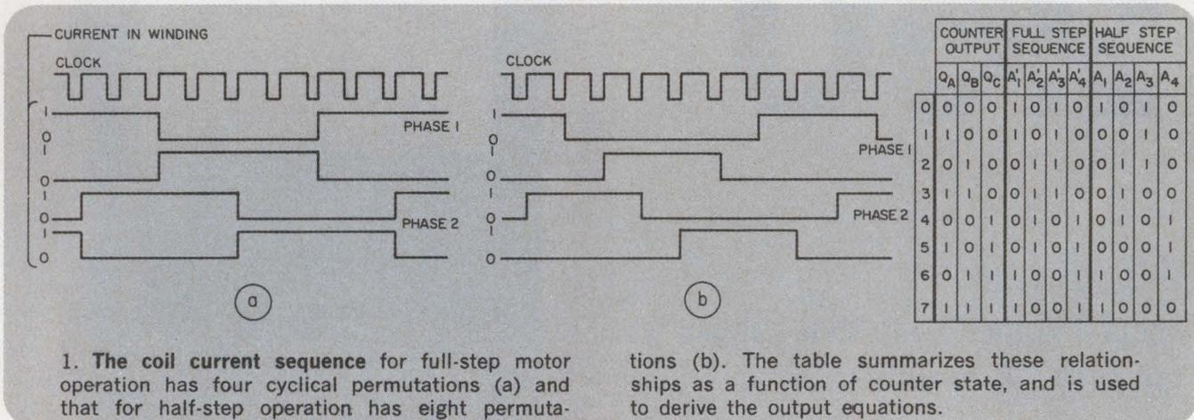
1. The coil current sequence for full-step motor operation has four cyclical permutations (a) and that for half-step operation has eight permuta-
