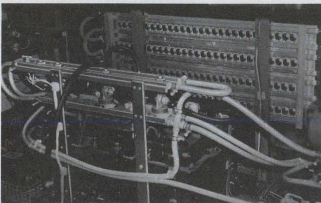
**6000 watts of heat** produced by 125 TO-3 case transistors in an industrial welding machine power supply was raw-power problem solved by IERC E4 liquid cooled sinks. Designer brazed together four standard E4's cut to 36 inches in length and tier stacked two other E4's to cool high power SCR's. Total area of heat sinks used only a fraction of the space required for a blower-cooled system of similar capacity.
