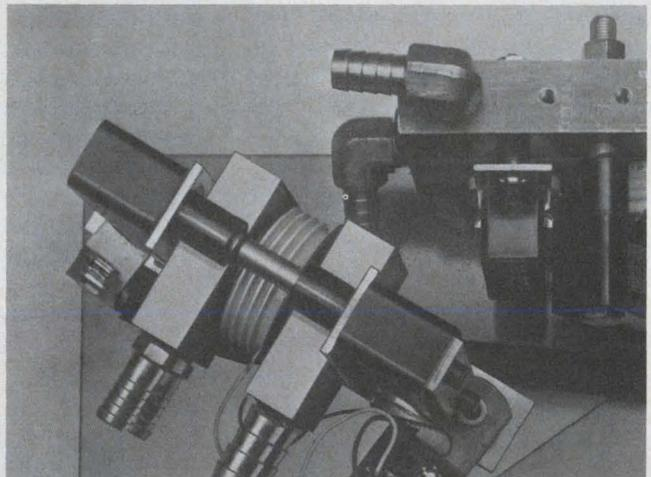
**Fork-lift truck speed control** used SCR's in hocky puck packages to handle thousands of watts in drive power. Big heat problem was solved with IERC liquid-cooled, double-side heat exchangers specially designed to let these big pressure-mount semiconductors dissipate on the order of 1000 watts each with just a 20°C case rise above ambient. Where did the designer get the coolant? He routed vehicle hydraulic fluid through the heat exchangers.
