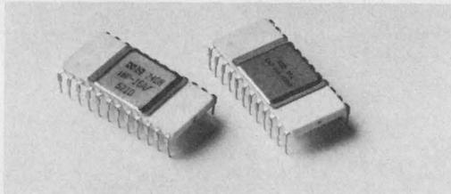
Chip #1, the one that does the work, is a Register and Arithmetic Logic Unit (RALU). And chip #2, the one that tells the RALUs what to do, is a Control and Read-Only Memory (CROM).
