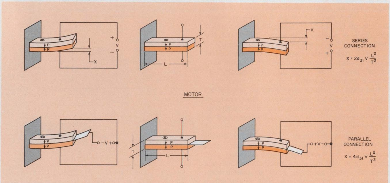
6. **Simple motor-bender applications** use a piezoelectric ceramic bonded to piezoceramic substrates.
