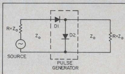
$D_2$  is less than that of  $D_1$ .  $D_2$  then ceases to conduct, and the output voltage rises towards the input-voltage level at a speed determined by the transition time of  $D_2$ . As soon as the  $D_2$  transition is complete,  $D_1$  recovers and stops conducting, so that the output voltage falls to zero.
