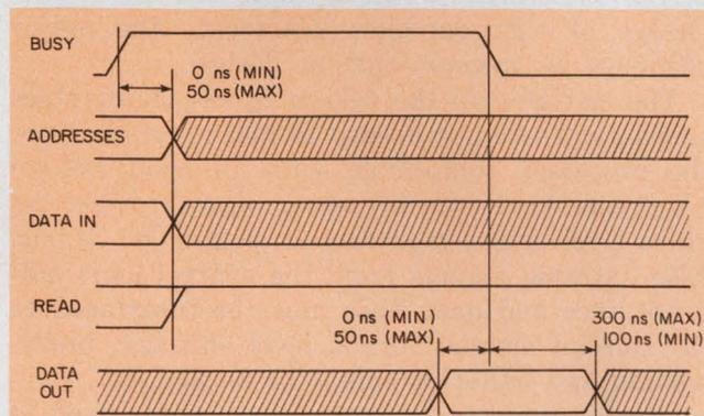
2. These control and data signals are sent back to the processor by the memory system.
