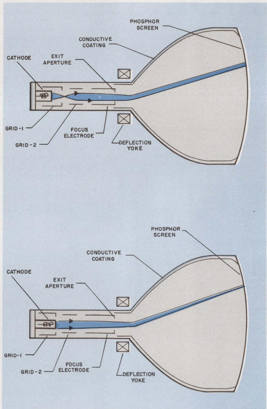
Electrons emitted from the cathode of the laminar flow gun (bottom) travel in a nearly parallel path beam until they converge to a focus at the viewing screen. This contrasts with the electron beam trajectory for the standard crossover type cathode-ray tube.
