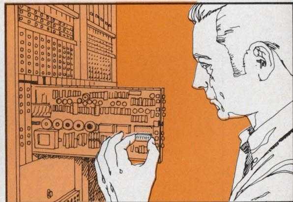
New CTS 206 Series switches will streamline your logic programming. These dual-in-line packages mount on the same PC board as other circuit components, eliminating the need for special mounting hardware/interconnection wiring. Program up to 10 different functions and/or signal levels with one compact switch.
