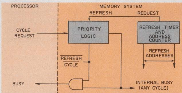
4. The controller section of an asynchronous design can include refresh-cycle interrupt logic needed for dynamic semiconductor memories.
