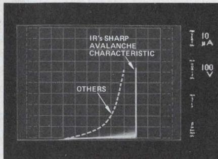
The avalanche curve pictured shows our "sharp" curve and the "soft" curve of the others. Convincing evidence of better junctions that you can operate at full rated specs without a worry.
