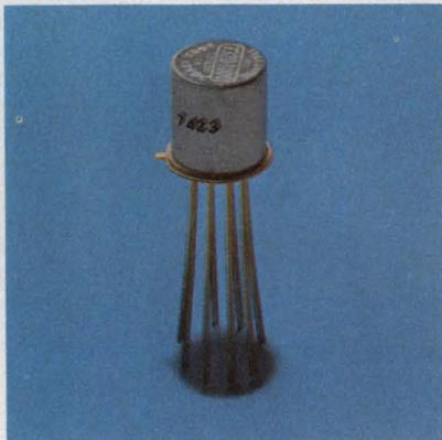
RF circuit and packaging engineers are discovering that Teledyne TO-5 relays make excellent subminiature rf switches for frequency ranges up through UHF. Their reasons are: inherently low inter-contact capacitance and low loss contact circuit geometry. Typical rf performance: Isolation — 45db at 100 MHz, 35db at 500 MHz;
