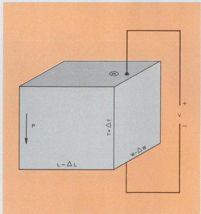
2. The electric fields required to pole the ceramic material are often as high as 100 V/mil.
