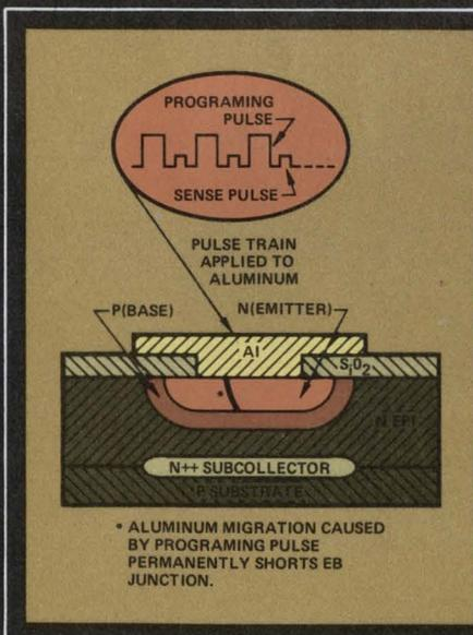
us to measure and control the quality of the programmed short, whereas it's impossible to measure a programmed "open" to a quality level that assures reliability.
