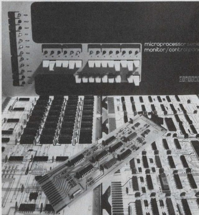
**A building-block approach to microcomputer designs** is offered by Digital Equipment Corp. The modules, using Intel's 8008 PMOS processor, contain the peripheral circuitry usually needed to operate the microprocessor.
