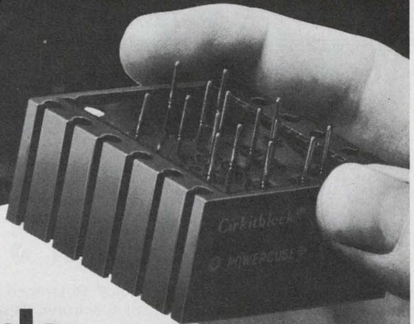
Powercube® has now added high-reliability, low-cost DC to DC Converters to our menu of off-the-shelf Circuitblock® modules.
