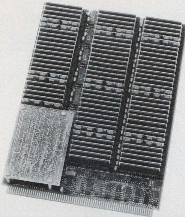
Hybrid packaging yields a 32-k x 18-bit 'micromemory' on a single board. General Automation offers the unit for use with the company's LSI-16 system.
