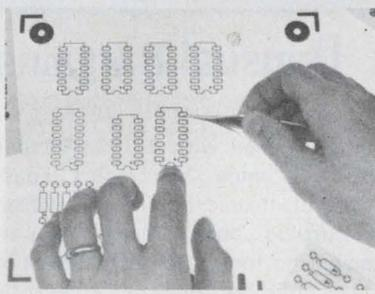
**Cut PC layout time 75% with PUPPETS™,** Bishop's die-cut, transparent, reusable layout patterns in 2X or 4X scale that represent electronic components. Contain no adhesive yet adhere to any clear, non-matte drafting film. FREE Sample & technical bulletin. Bishop Graphics, Inc., 20450 Plummer Street, Chatsworth, CA 91311 (213) 993-1000.
