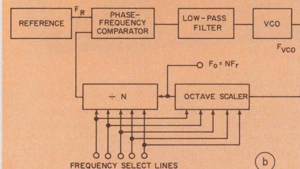
1. Conventional frequency multipliers (a) require selection of M and N. An improved version (b) requires selection of only N, and it reduces the VCO tuning range.
