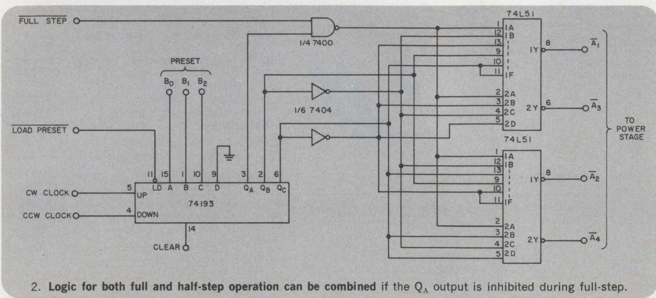
2. Logic for both full and half-step operation can be combined if the  $Q_A$  output is inhibited during full-step.
