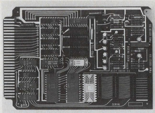
Microcomputers on PC boards are offered by Pro-Log, Models available include a 4-bit system for dedicated-controller applications and an 8-bit model for data processing. Both systems use Intel chips.
