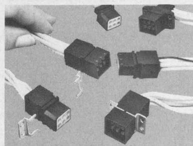
CAPITRON subminiature LGH high-voltage connectors. They're lightweight—a mated pair is less than 14 gr. And compact—requires less than .6 sq. in. of mounting surface. Operates up to 5 KVDC at 70,000 feet. And within a temperature range of -55°C to +125°C. AMP Incorporated, Capatron Division, Harrisburg, Pa. 17105. (717) 564-0100.
