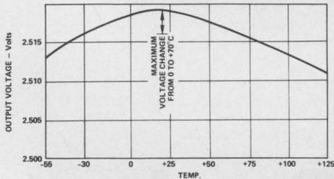
It's a three terminal, bandgap voltage reference that you just plug in—no external components. And it's the only one that works from the same power supply as your logic system—5 volts.
