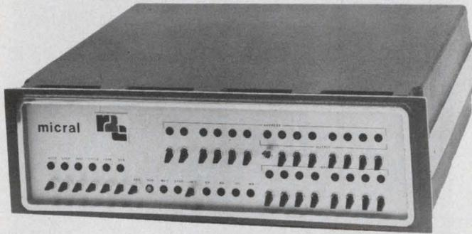
**Complete microcomputers extend the capabilities** of the basic microprocessor used. R2E's Micral system, for example, provides additional instructions for interrupt handling and data manipulation. R2E uses Intel chips.
