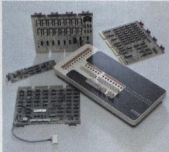
Software development is easier, too. Control programs are prepared on a small, low-cost PDP-8 minicomputer, using the MPS software development kit of six basic programs. And the modular construction of the MPS allows you to buy only what you need for your application.
