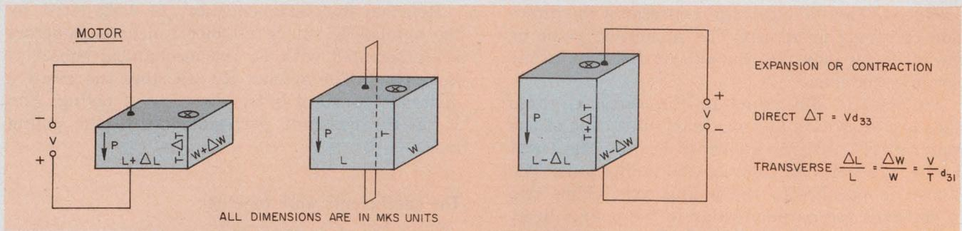
5. **Motor applications of the ceramic** let the material expand or contract when voltage is applied. Be careful
