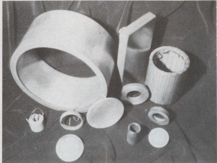
1. Piezoelectric ceramic materials are available in many shapes and sizes.
