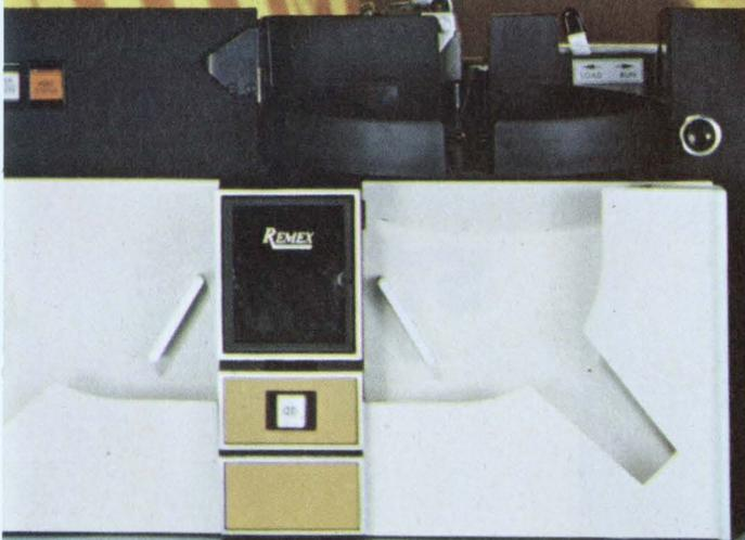
High speed punched tape perforator/reader combos
