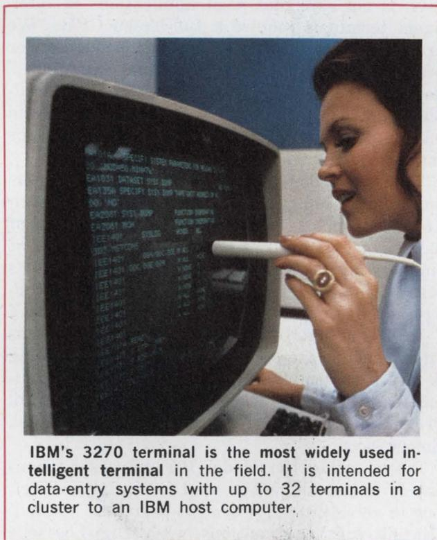
IBM's 3270 terminal is the most widely used intelligent terminal in the field. It is intended for data-entry systems with up to 32 terminals in a cluster to an IBM host computer.
