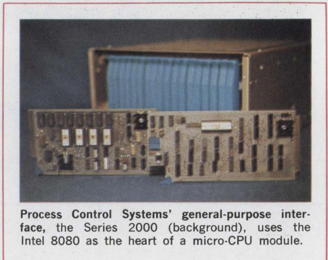
Process Control Systems' general-purpose interface, the Series 2000 (background), uses the Intel 8080 as the heart of a micro-CPU module.
