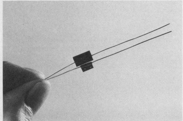
These microminiature solid tantalum capacitors are epoxy-sealed in a polyester sleeve. They're available in both cylindrical cordwood and rectangular modular form, with a choice of axial or radial leads. Capacitance values are 0.001 to 220MFD, working voltages are 2 to 50VDC, and tolerances are  $\pm 10\%$  and  $\pm 20\%$ . They're in excellent supply. We can meet your needs now.
