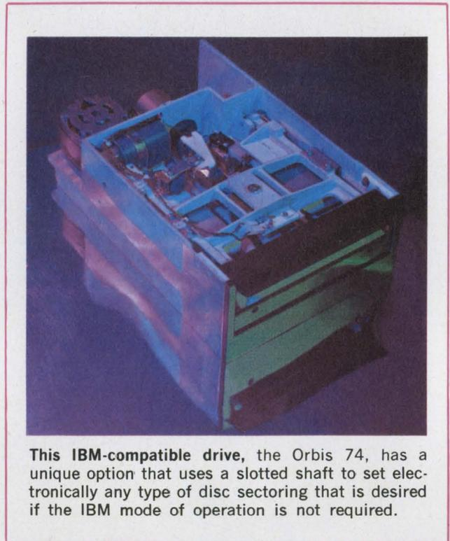
This IBM-compatible drive, the Orbis 74, has a unique option that uses a slotted shaft to set electronically any type of disc sectoring that is desired if the IBM mode of operation is not required.
