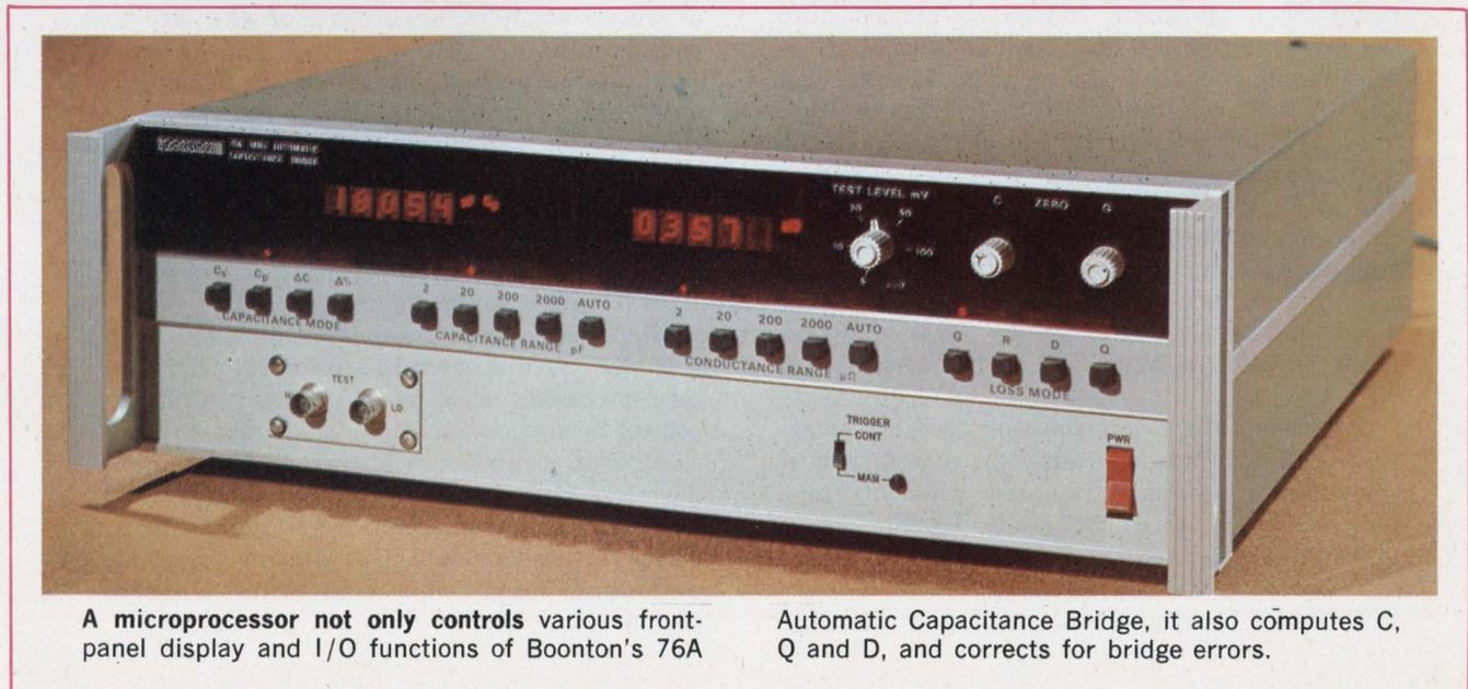
A microprocessor not only controls various front-panel display and I/O functions of Boonton's 76A
