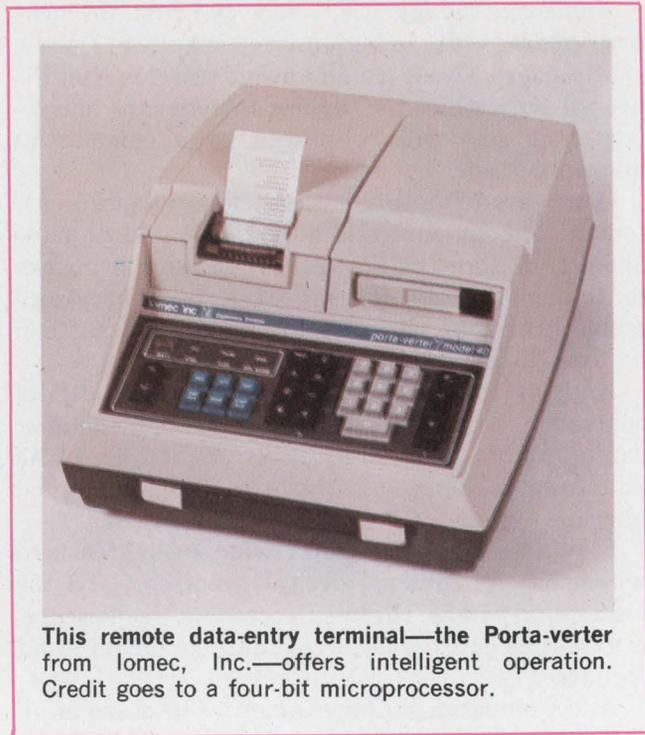
This remote data-entry terminal—the Porta-verter from Iomec, Inc.—offers intelligent operation. Credit goes to a four-bit microprocessor.
