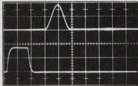
Sine<sup>2</sup> pulse (top waveform) and 100 ns pulse (bottom waveform).
