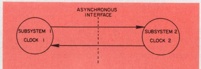
5. In a complex computer system each subsystem is likely to have its own clock. With this arrangement, problems can occur at the asynchronous interface of the subsystems, and errors can result.
