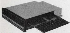
The 306/MFFT Fast Fourier Transform Processor is delivered with all control programs and plugs directly into any Data General Nova computer. It offers a complete Fourier Transform capability including Forward and Inverse FFT, Spectral magnitude, Hanning Weighting, and Complex Multiplication. Arrays from 16 to 16,384 real samples can be processed. An array of 1024 real samples is transformed in only 139 ms.
