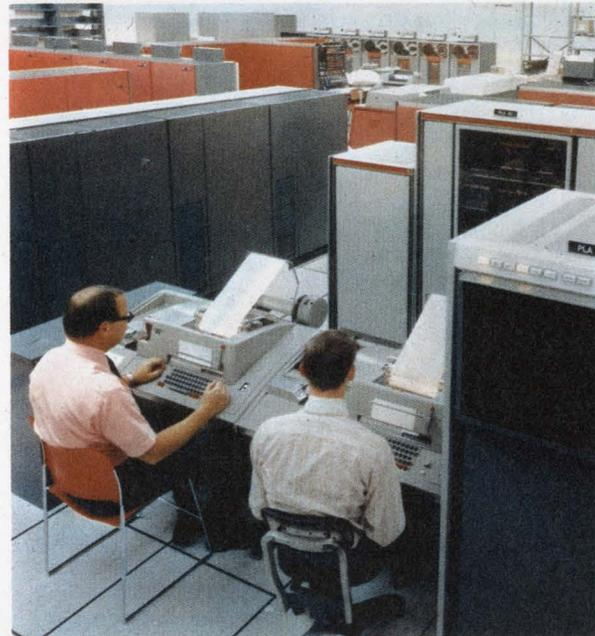
**The Collins C-System uses a localized high-speed ring to join hosts and storage devices. Low-speed loops drive terminals and input devices. The system shown provides a statewide Iowa police network, with access to more than seven million traffic records and 250,000 criminal records on file in a System/370 complex at Des Moines.**
