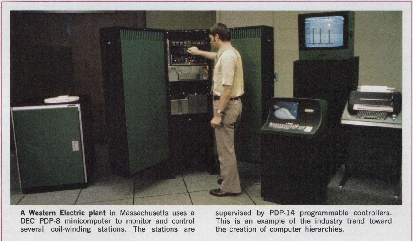
**A Western Electric plant in Massachusetts uses a DEC PDP-8 minicomputer to monitor and control several coil-winding stations. The stations are**
