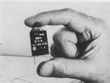
**Overcurrent Protector**, manual reset eliminates fuse replacement. Convenient panel mounting. 15 fractional ratings from 0.1 to 3 amp. Other models up to 400 amp. Trip-free and fool-proof, UL and CSA approved. High quality, low cost-\$1.12 ea. in 1000 lots. E-T-A Products Co. of America, 6284 N. Cicero Ave., Chicago, Ill. 60646. Tel. (312) 545-1553.
