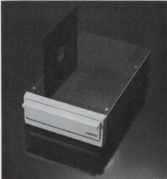
The smallest, lightest and cheapest IBM-compatible drive is from Perotec. The D0330 is also the only totally dc driven drive. All others use an ac motor to spin the disc.
