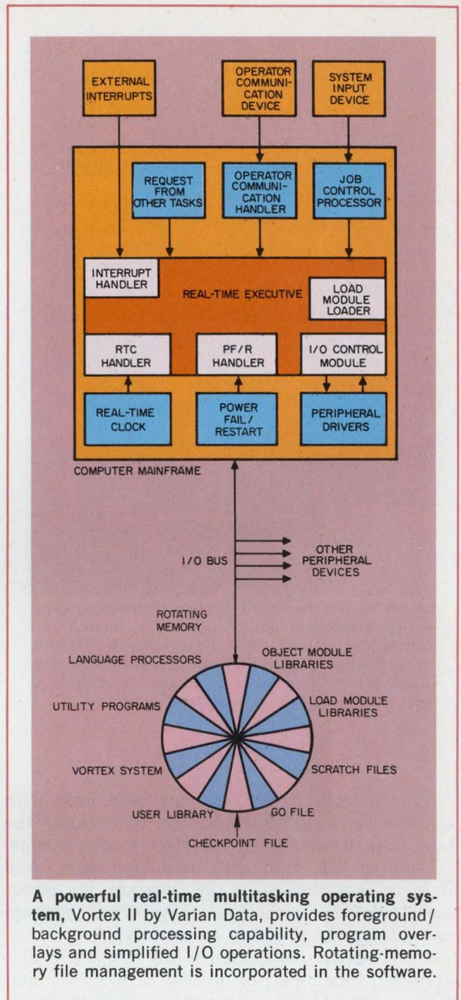
**A powerful real-time multitasking operating system, Vortex II by Varian Data, provides foreground/background processing capability, program overlays and simplified I/O operations. Rotating-memory file management is incorporated in the software.**
