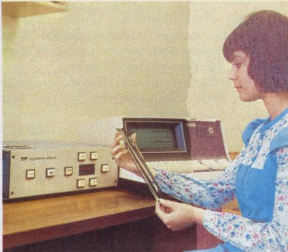
**Holographic data retrieval unit** from TRW is used to read data stored on 35 mm film. A separate holographic recorder is used to store data.
