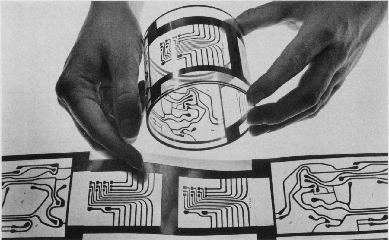
**Copper conservation** is an objective of this printed-circuit process introduced a number of years ago by Western Electric Co. In the process, copper cir-
