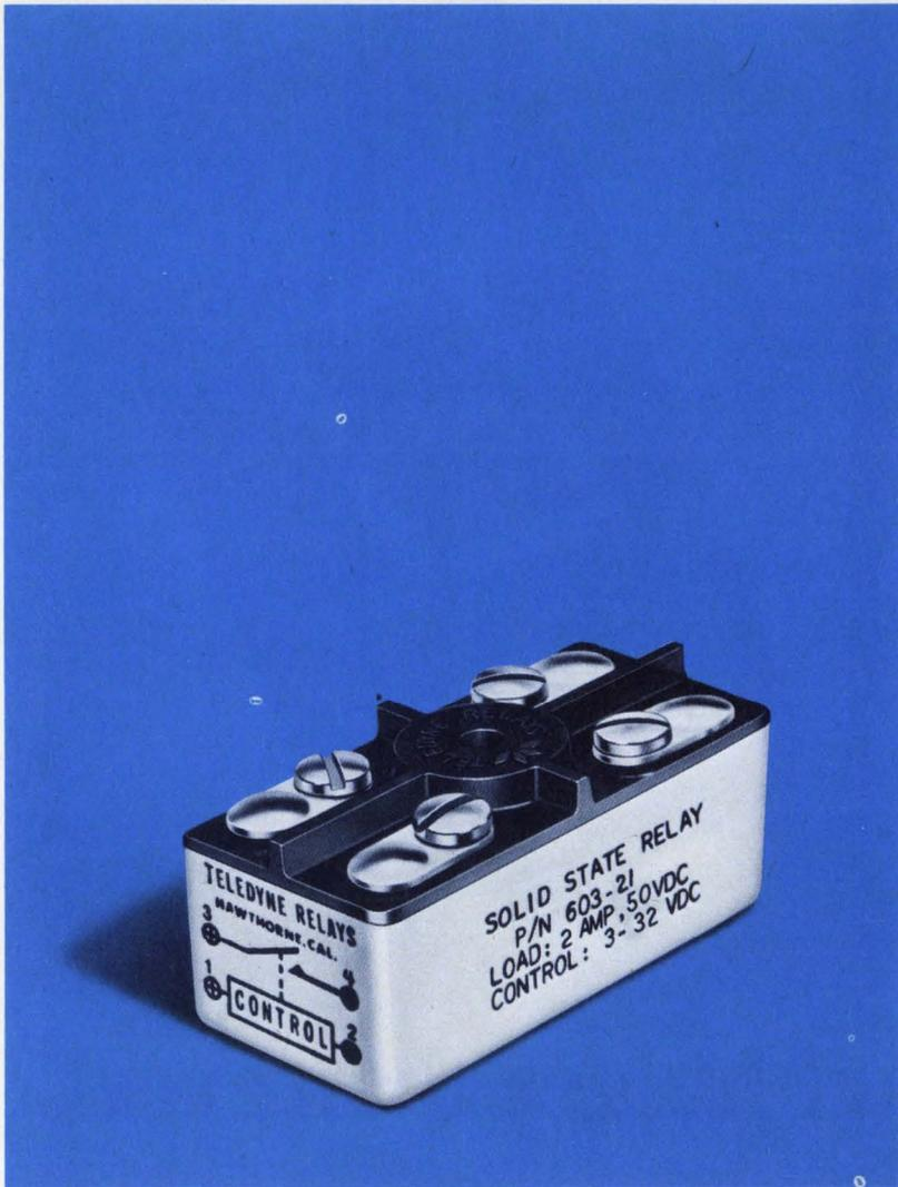
Take a good solid state DC relay — Teledyne's 603, for example — add some shaping circuitry so its response waveshape is carefully altered (rise time, turn-off slope, etc.), and something good happens for designers. In-rush currents for capacitive and lamp loads are limited, and so are turn-off transients for inductive loads. Also, controlled rise and fall time minimize EMI and switching transients.
