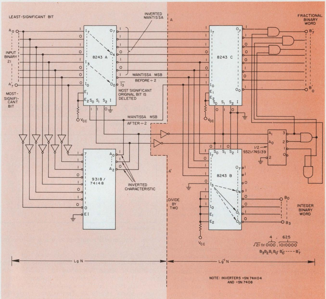
2. A combinational 8-bit square rooter needs only a  $\log_2$  circuit, a wired divide-by-2 and an antilog<sub>2</sub> circuit.
