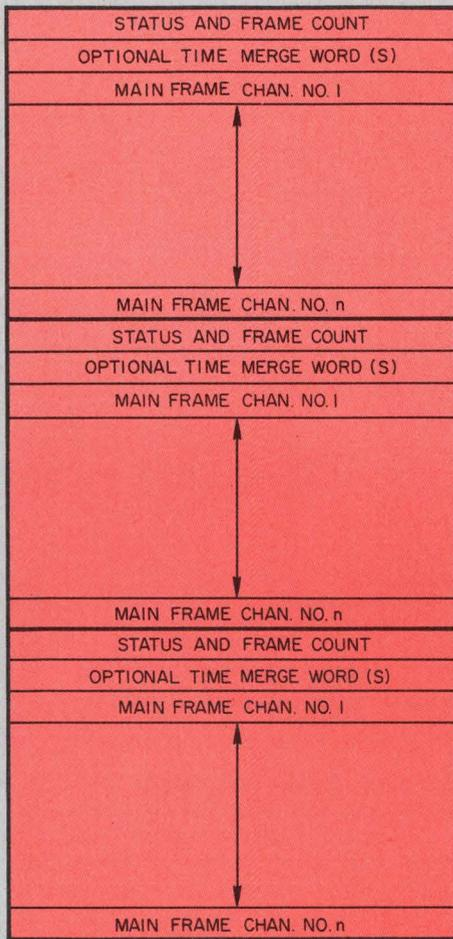
5. A typical data block in memory starts at location  $x$  and consists of  $y$  words. The status block permits the computation of the subframe or channel at which sampling began. The buffer signals the computer via an interrupt when a block is completed and begins a new block in an alternate buffer area.
