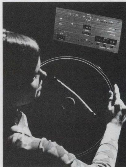
**LED auto control panel** conceived by Monsanto. About 1500 individual light-emitting diodes on this dashboard give information on gallons of gasoline left, miles per hour, cumulative miles driven, exact time, elapsed time, seat-belt status and door and hand-brake status.
