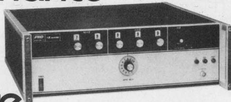
**Our 7828 Frequency Synthesizer** is offered with 1 kHz phase-locked steps from 1 kHz to 80 MHz. An optional vernier provides 1 Hz resolution. It's fully programmable with contact closures, RTL, DTL, or TTL logic; 1 part in  $10^6$ /mo stability; up to 1.0 volt output into 50 ohms.
