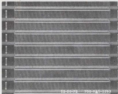
Adjacent stripes of silicon and aluminum nitride are deposited on a wafer of sapphire. The delay line goes on the aluminum nitride substrate and the MOS detectors on the silicon. This is a 63-tap switchable delay line with a center frequency of 200 MHz.
