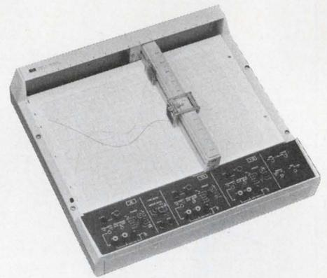
You can plot two signals at once with HP's 7046 high-speed two-pen x-y recorder. Acceleration of the y axis is  $> 2,500 \text{ in/sec}^2$  (6.3 meters/sec<sup>2</sup>); and on each x axis,  $1,500 \text{ in/sec}^2$  (3.9 meters/sec<sup>2</sup>). The y axis pens go from 0 to 30 in/sec (76 cm/sec) in less than 15 milliseconds. Even at these fast speeds, accuracy is  $\pm 0.2\%$  of full scale and overshoot is  $< 1\%$  of full scale.
