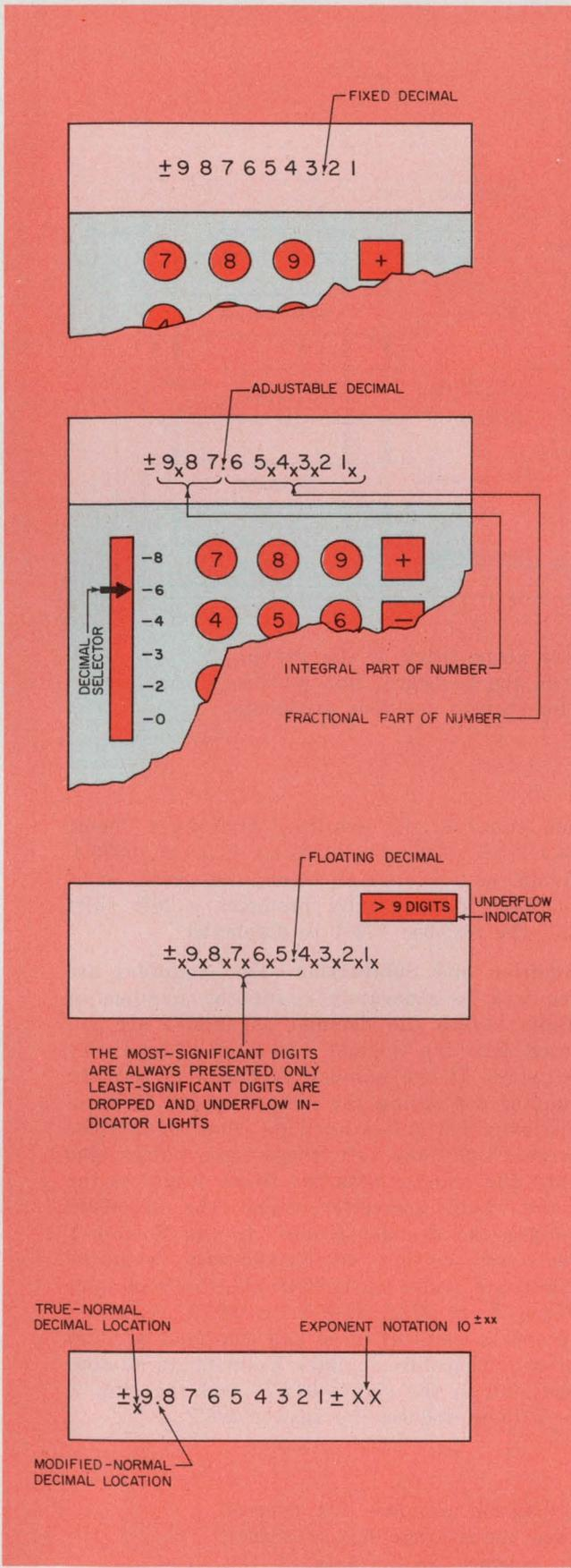
**Calculator displays use a variety of methods** for handling the decimal point. They vary from the simplest fixed-point system used in accounting machines to the most advanced floating-point and exponential notation methods for scientific calculations.
