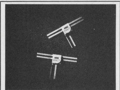
**The V981 and V982 very high speed switching transistors** have FT of 8 GHz and 6.5 GHz respectively. These NEC Transistors are for fast switching in an ECL configuration for systems operating at speeds in the hundreds of megabits per second. California Eastern Laboratories, One Edwards Court, Burlingame, Calif., 94010. (415) 342-7744.
