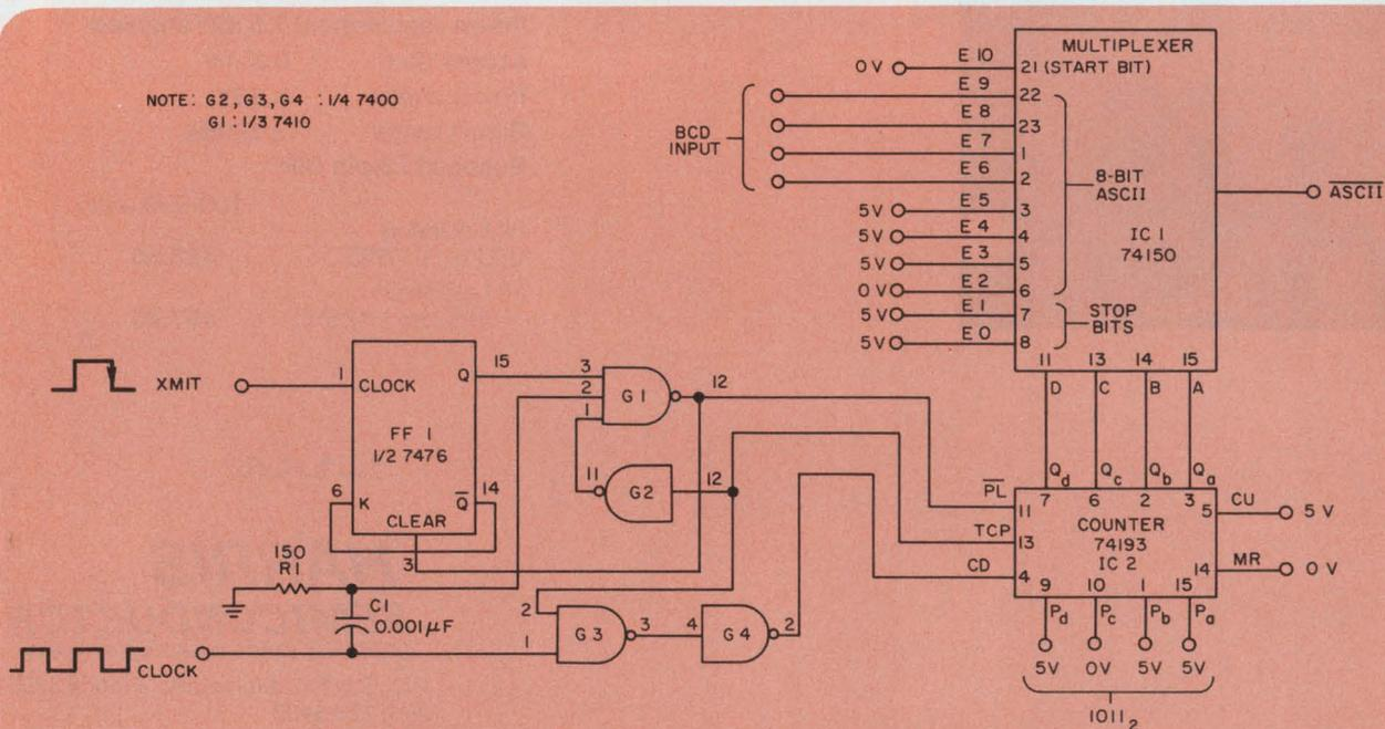
Multiplexer IC furnishes complemented eight-bit serial ASCII output with each countdown of IC<sub>2</sub>. A single countdown by IC<sub>2</sub> provides the eight-bit
