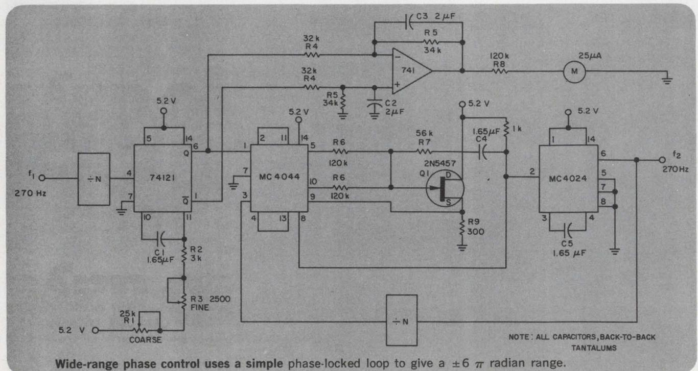
Wide-range phase control uses a simple phase-locked loop to give a  $\pm 6 \pi$  radian range.
