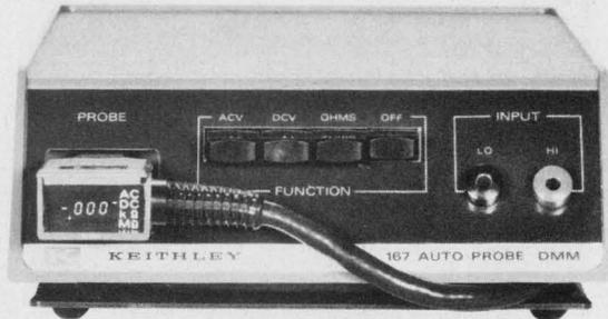
An in-probe readout makes Keithley's 167 an unusual DMM. The autoranging unit costs \$325.
