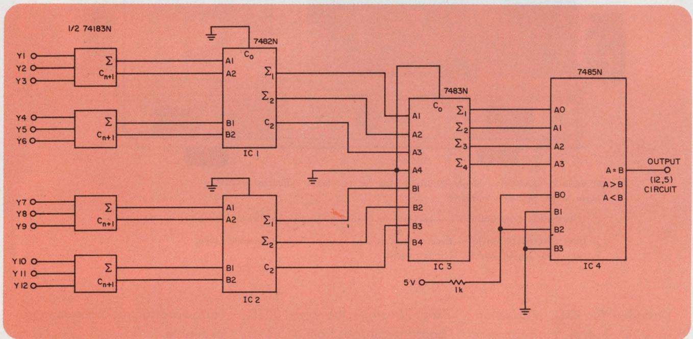
Circuit detects when five out of 12 inputs are true, by examining the binary sum at the output of IC<sub>3</sub>.
