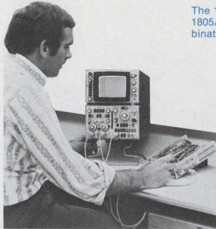
The 184A fast-writing storage scope with 1805A and 1825A plug-ins is the ideal combination for capturing elusive transients.
