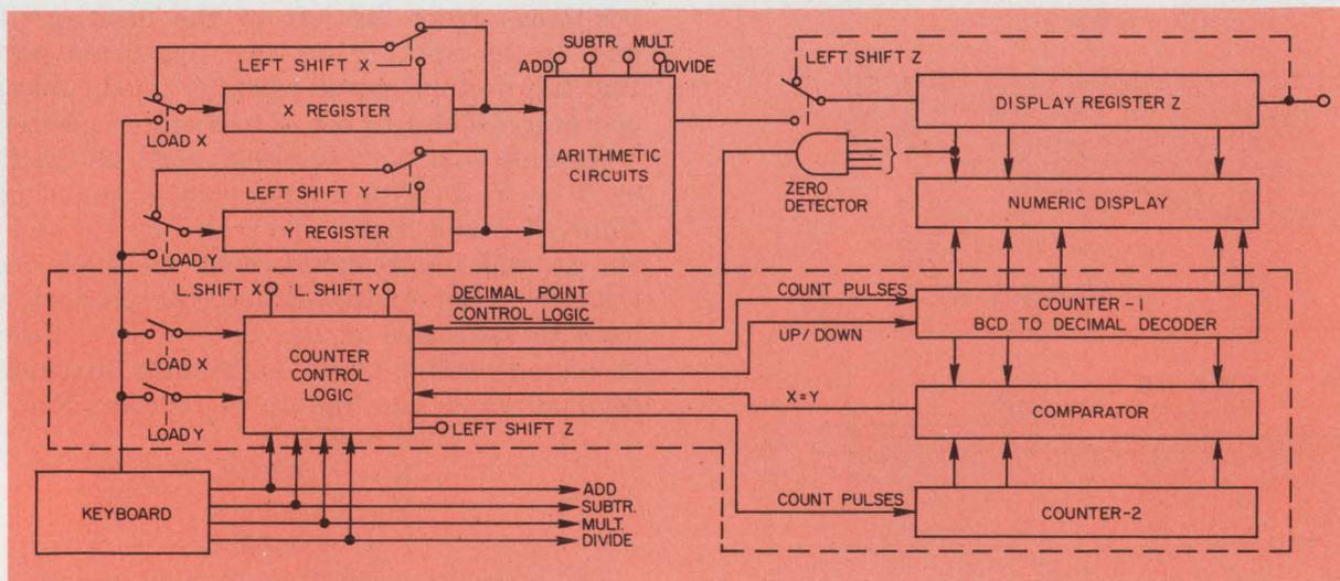
A floating-point calculator automatically keeps track of the decimal with the help of the decimal-point key on the keyboard. The routines performed by the circuit are different for each of the four arithmetic operations, thus:
