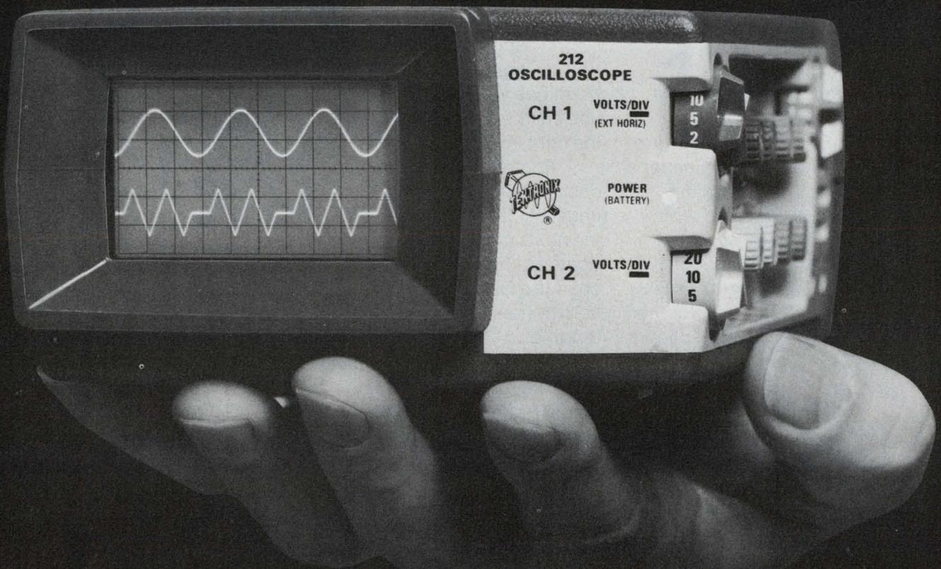
With the 212. A completely new DUAL-TRACE, 500-kHz, 3 x 5/4 x 9-inch scope that weighs only 3.4 pounds and costs just \$725. The high-impact plastic case withstands severe environments — double-insulated construction helps protect you while making high-voltage measurements.
