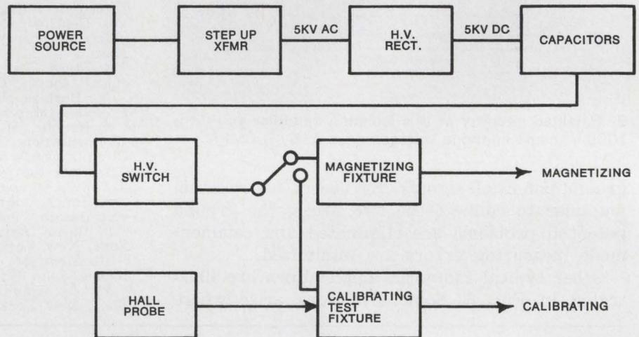
The magnetizing power unit in a typical system charges in as little as 30 seconds and delivers calibration pulses up to 20,000 watt-seconds.
