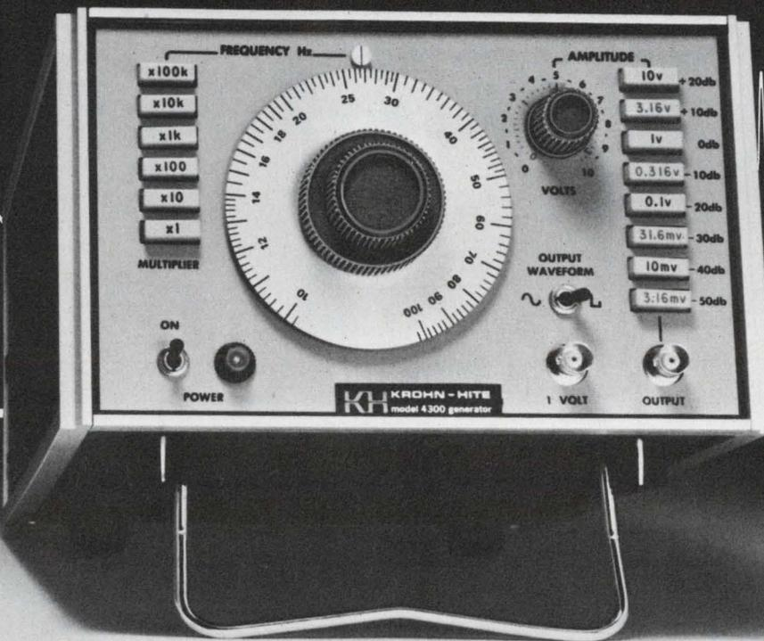
**Model 4300 oscillator with 0.025 db frequency response and precision calibrated attenuator eliminates need for constant monitoring and adjustment.**
