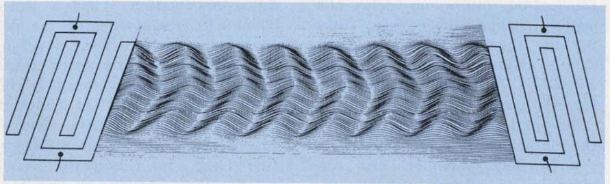
**Basic interdigital electrode patterns** for excitation and detection of surface acoustic waves on a piezoelectric substrate. The surface-wave pattern shown was derived from voltage-probe measurements at the Lincoln Laboratory.
