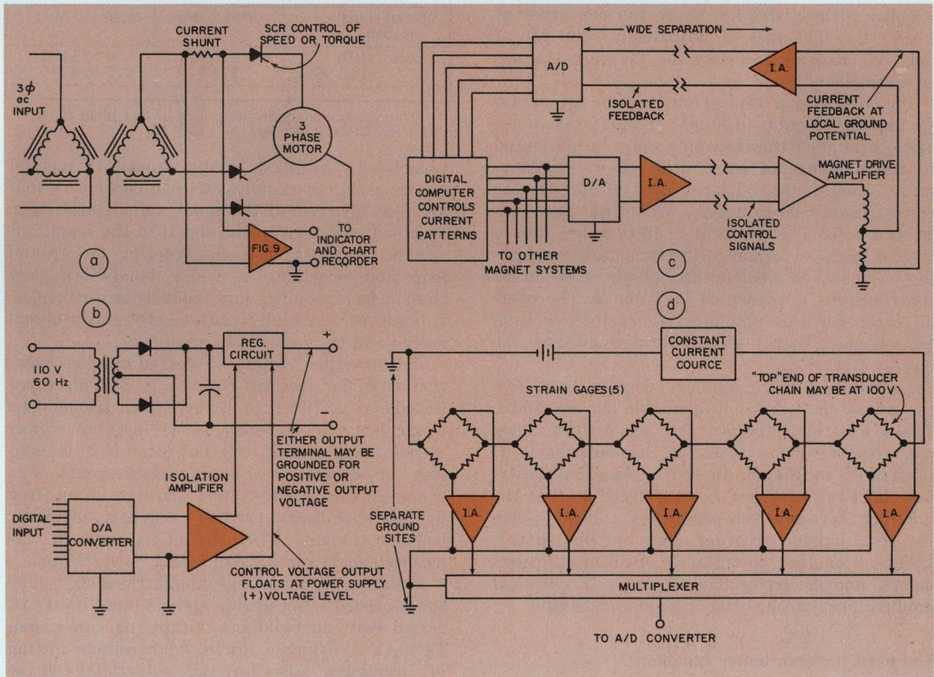
8. Isolation amplifiers can be used to monitor current in motors (a) to control high-voltage regulators digitally (b) to send control signals for a computer-run magnetic
