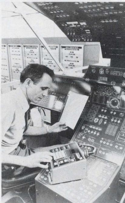
Automatically Controlled Electrical System is being tested in a mockup of the space-shuttle cockpit. The new system moves the power switching location from the cockpit to remote electrical load centers.
