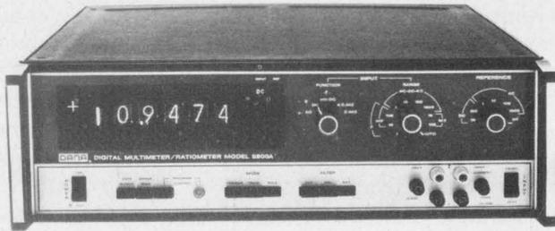
Dana's 5800A is characterized by an rms, distortion-insensitive ac converter, and other systems features.
