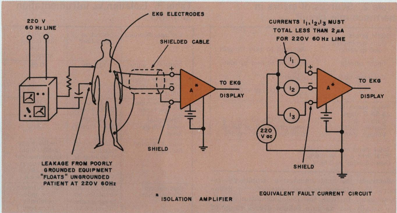
7. Biomedical measurements require extremely small input currents and large isolation resistance values.
