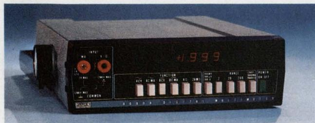
Fluke's 8000A—the first to use both analog and digital LSI chips. Featured are a high-impact case, overload protection and a weight of less than 3 pounds.
