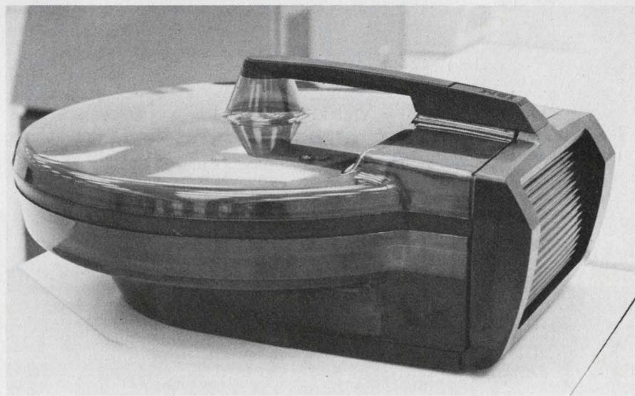
Increased data reliability results from combining disc, access arms and read/write heads into a single removable cartridge.
