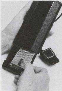
Insert the reference board into the logic comparator.
