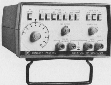
**Brand New Function Generator 3311A** shows what a performance plus you get from this technology in action. Priced at only \$249, it adds sweep capability and a separate high-power pulse output to the usual sine, square and triangular wave outputs. Sweep it over any 10 to 1 span within its 0.1 Hz to 1 MHz range. The pulse output drives up to
