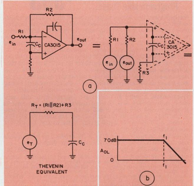
3. The amplifier equivalent circuit (a) shows the effect of the input lag-compensation capacitor,  $C_c$ , on the open-loop gain characteristics, (b). That is,  $C_c$  attenuates the effective open-loop gain of the amplifier at the frequency  $f_1$ .
