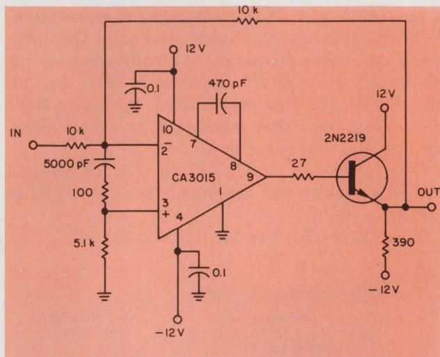
4. The complete unity-gain amplifier demonstrates the simplicity of designing a suitable input lag compensation to meet a given performance criterion, see text for step-by-step design procedure. The power supply is decoupled using a pair of ceramic capacitors. To minimize the effects of capacitive loading, an emitter follower is added.
