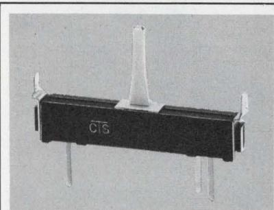
**Big Savings in New CTS Series 470 1 3/4" Linear Motion Composition Slide Control** — Full size performance in space saving 5/16" x 5/8" molded housing. Only 21¢ in quantity. Excellent settability, stability . . . low noise. Varied mountings. 1/2 watt power; 200 Ω - 5 meg Ω CTS of Brownsville Inc., Brownsville, Texas 78520. (512) 546-5184.
