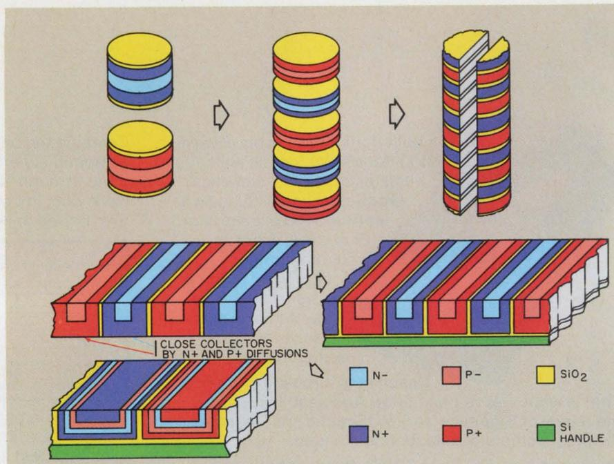
A new approach to power-integrated circuits is being studied by RCA. Stacked wafers of doped semiconductor material, separated by oxide, are sliced longitudinally and the device is completed with standard processing.
