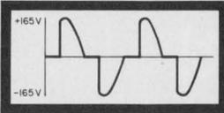
Load voltage using full-wave SCR phase control
