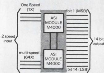
The block diagram shows two ASI modules which form a complete 14-bit 2-speed converter. No external mixing logic or programming is required. For further information contact astrosystems, inc.
