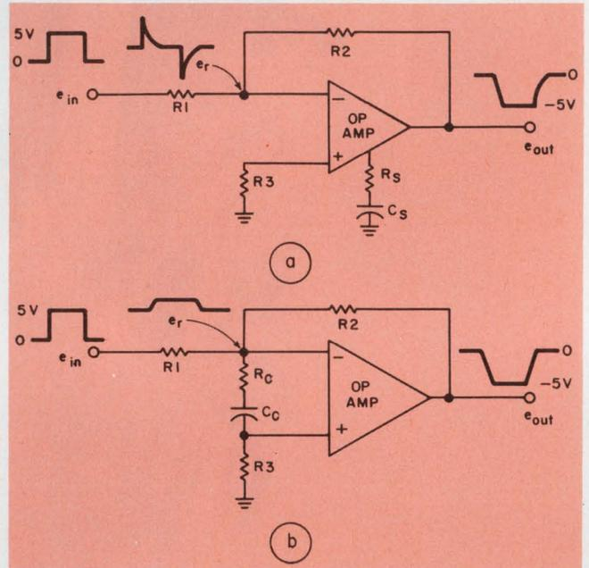
1. Increase in bandwidth and slew rates is obtained by placing the standard lag compensation network,  $R_s C_s$ , (a), across the op amp input or summing points, (b). The error voltage,  $e_r$ , is now averaged by the time constant  $R_c C_c$ , thus preventing first-stage saturation.
