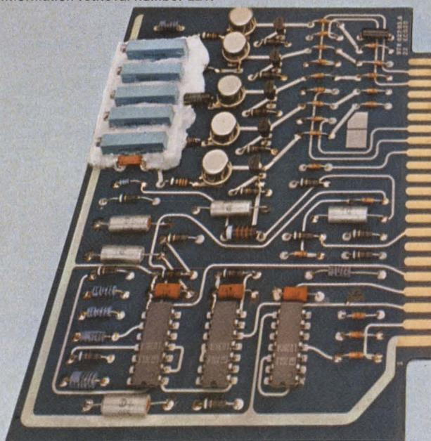
For excellent adhesion to corrosion-prone metals such as copper, use this new noncorrosive, one-part Dow Corning sealant. Cure mechanism produces no exothermic heat or acetic acid. Information retrieval number 223.
