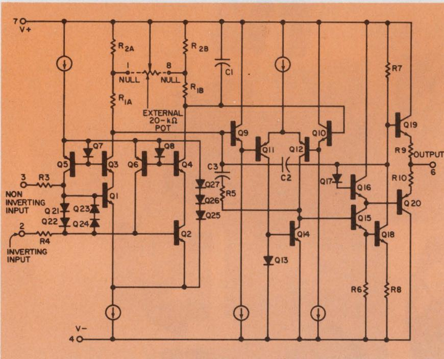
pk-pk noise voltage of  $0.7 \mu\text{V}$  (10-Hz bandwidth), with  $0.38 \mu\text{V}$  typical, and a maximum drift of  $0.6 \mu\text{V}/^\circ\text{C}$  (E versions). By comparison, the  $\mu\text{A} 725$  has a higher typical pk-pk noise voltage of  $1.0 \mu\text{V}$ ; no maximum noise voltage or drift spec is listed.
