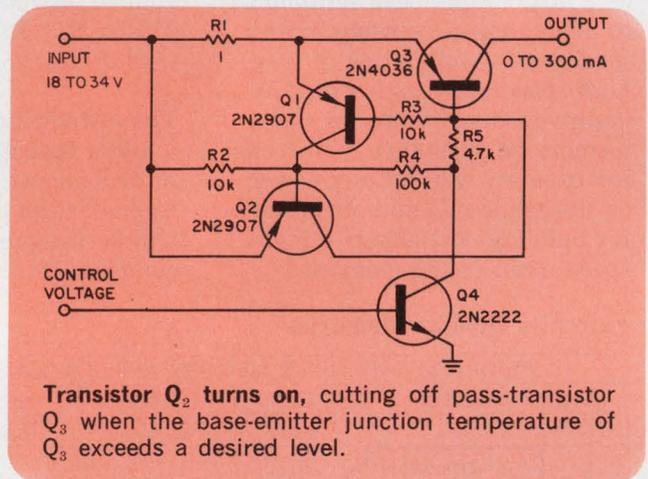
If it's assumed that  $Q_2$  and  $Q_3$  have equal base-emitter voltages at the same current and temperature, the current supplied by  $R_4$  should be adjusted as follows to obtain the desired cut-off temperature differential:
