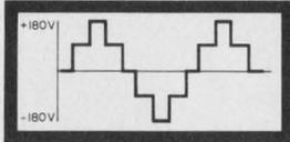
Sine wave synthesis by voltage switching
