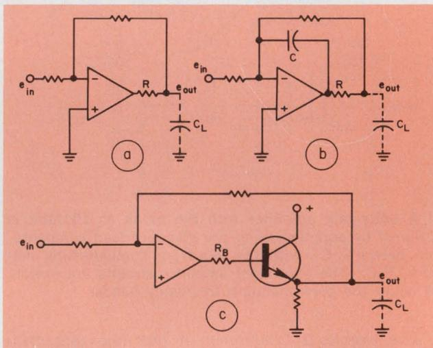
5. To minimize the effects of capacitive loading, a resistor (a), or a resistor-capacitor (b), or an emitter follower (c) can be added to an amplifier as shown. Also see text for several practical tips on layout, grounding, decoupling.
