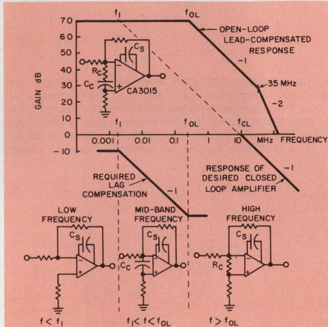
2. A unity-gain amplifier with the break at 10 MHz is obtained by supplementing the standard lead compensation network,  $C_s$ , with the input lag compensating network,  $R_c C_c$ . The equivalent amplifier circuits are sketched below the corresponding frequency bands.
