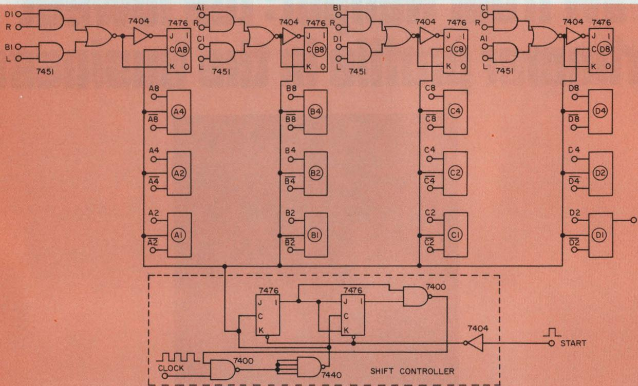
1. Interconnection scheme for digit shifting in a shift register saves gates, interconnecting leads
