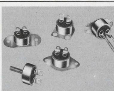
**Prototypes of precision snap-action thermostats** from Elmwood, widely specified for quick, reliable response; proven industrial and military performance record. Environ. expos. -85° to 550°F; narrow or wide diff.; rated to 15 amps. Wide choice of brackets, terminals. Elmwood Sensors, Inc. (401) 781-6500. TWX 710-381-6413.
