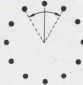
With a bidirectional model, a pulse to one coil gives cw step, to the other, ccw. Standard shelf models move in increments of 10, 15, 20, 30, or 36 degrees.
