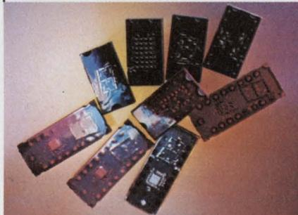
LED display with an internal TTL/MSI logic chip providing latch, decoder and driver. It accepts 8-4-2-1 data and displays 0 through 9 and A through F with both right and left decimal points.
