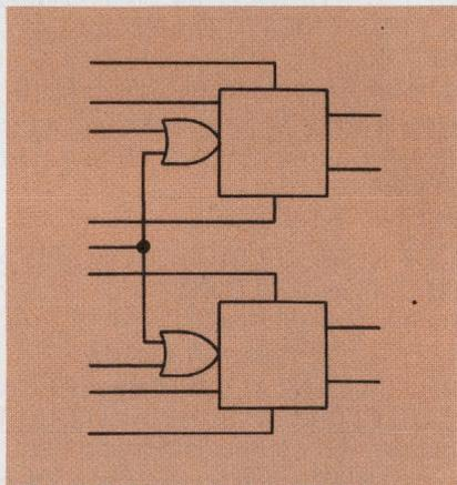
MC10231 High-Speed Dual D Flip-Flop
