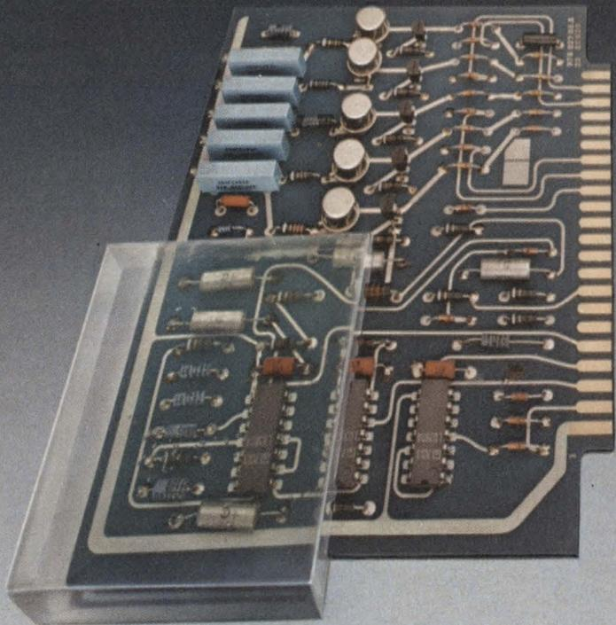
For see-through protection, encapsulate with this clear, resilient silicone resin. Self-extinguishing, it guards against humidity, heat, cold, radiation, thermal shock and vibration. Information retrieval number 221.
