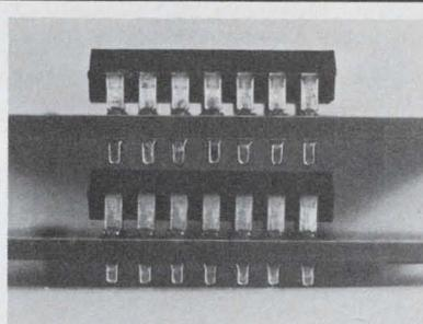
**Minisert® P.C. Socket** for use where space is restricted. Extends just .030" above and .088" below board; allows .400" board-to-board spacing. Accepts up to .023" round or flat leads. Machine insertable at rates up to 3000 per hour. Berg Electronics, Inc., New Cumberland, Pa. 17070. Phone (717) 938-6711.
