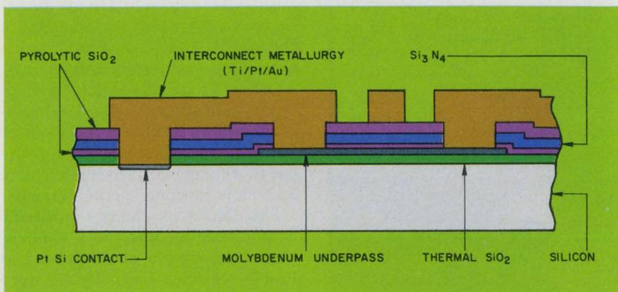
**Molybdenum underpasses**, which appear as light blue rectangles in the photo above, replace the usual diffused silicon ones to minimize parasitic capacitance, lower underpass resistivity and improve device yield. Active devices surround the gold-colored power and ground bus lines. As can be readily seen, half of the area of the beam-lead LSI chip is taken up by interconnection paths. The cross-sectional view (drawing) shows the underpass structure.
