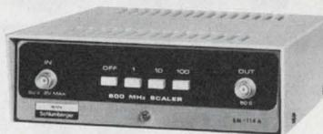
The new Heath/Schlumberger SM-114A Scaler extends the useful range of any counter with more than 100 kHz capability. Three pushbutton-selected ranges allow division of input frequency by 1, 10 and 100. The  $\div 1$  range provides for direct transmission of frequencies from 10 MHz to 100 MHz with a gain of 17 dB;  $\div 10$  and  $\div 100$  ranges will scale frequencies between 40 MHz and 600 MHz.
