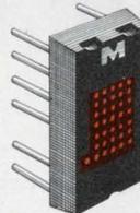
**MAN2** — A 5 x 7 light-emitting-diode matrix, the .35" MAN2 alphanumeric displays the full 64-character ASCII code. Finds application as keyboard verifier, avionics display, in computer peripherals and has 2<sup>36</sup> bits available for film annotation work.
