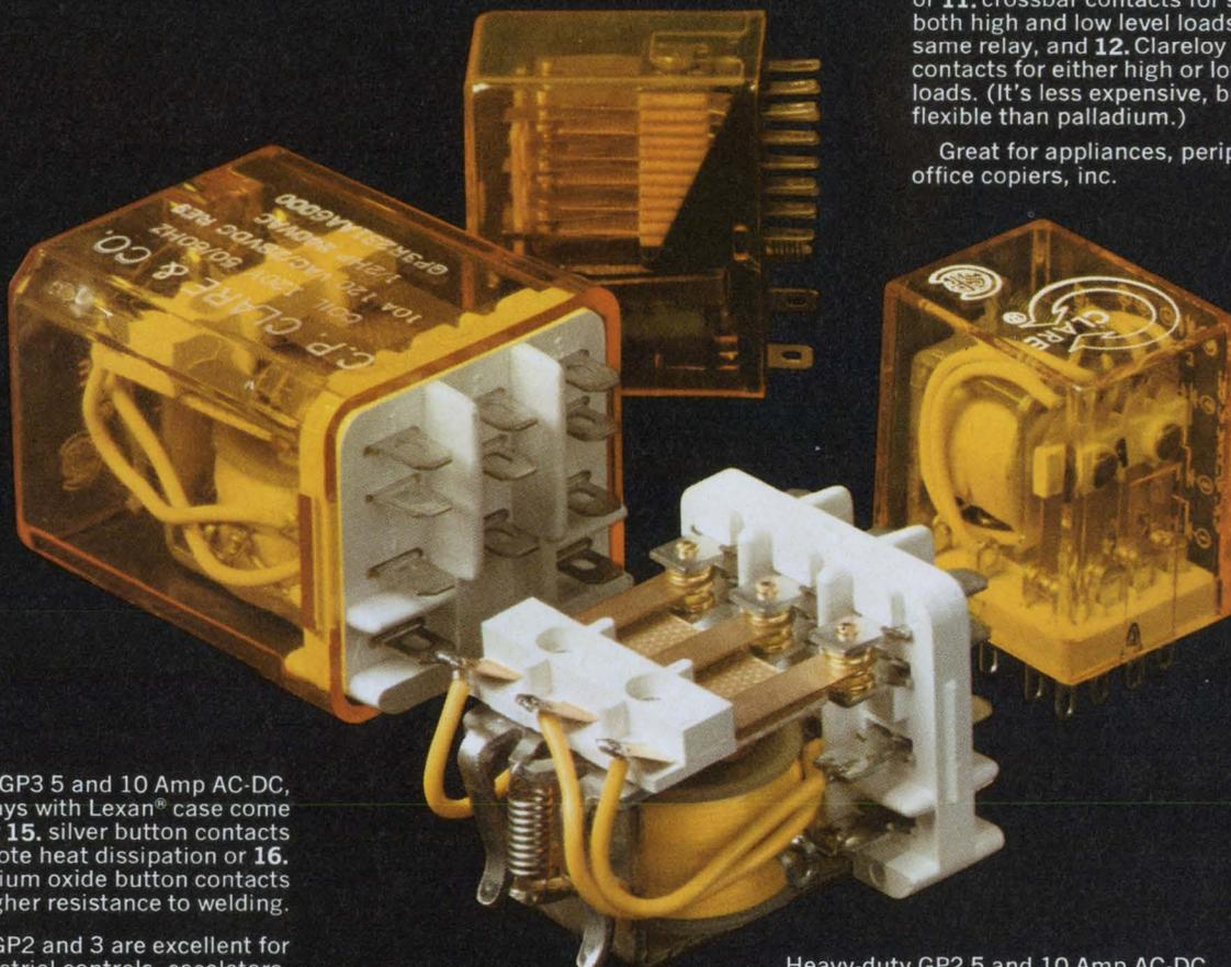
Rugged GP3 5 and 10 Amp AC-DC, 3PDT relays with Lexan® case come with either **15.** silver button contacts that promote heat dissipation or **16.** silver cadmium oxide button contacts with higher resistance to welding.
