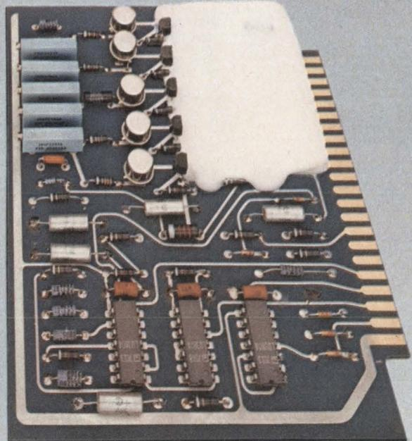
For protection against moisture, dirt, ozone, radiation and many solvents and chemicals, select this conformal coating. It flows on easily and cures at room temperature to a tough silicone rubber with excellent dielectric properties. Information retrieval number 224.
