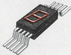
**MAN3A** — Encapsulated in transparent red epoxy, this small (.115") readout is very useful in desk calculator displays, portable instruments, and film annotation sockets. Displays ten digits and nine letters.
