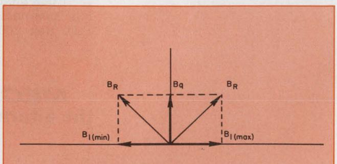
2. The phase-opposing field,  $B_p$ , centers the current-produced vectors about the origin. The resulting field,  $B_r$ , moves from second quadrant to the first as the current changes from  $I$  (min) to  $I$  (max).
