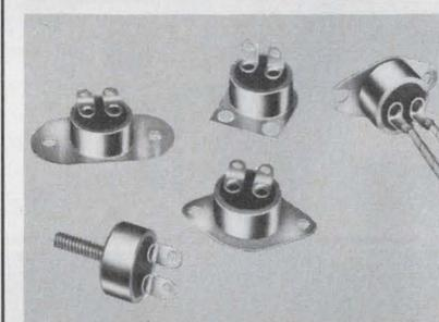
**Prototypes of precision snap-action thermostats** from Elmwood, widely specified for quick, reliable response; proven industrial and military performance record. Environ. expos.  $-85^{\circ}$  to  $550^{\circ}\text{F}$ ; narrow or wide diff.; rated to 15 amps. Wide choice of brackets, terminals. Elmwood Sensors, Inc. (401) 781-6500. TWX 710-381-6413.
