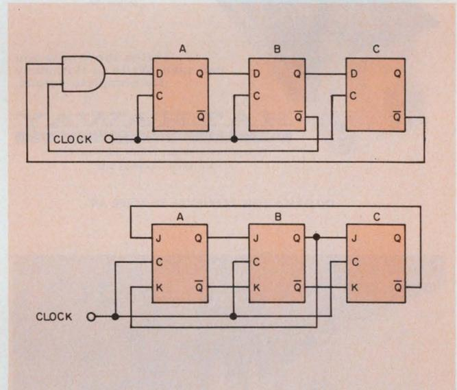
8. A divide-by-seven shift counter designed with the sequence-tree method. Both flip-flop types are shown.
