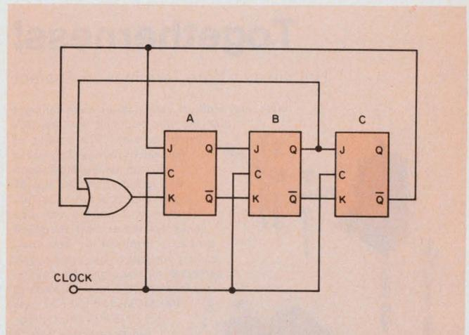
7. The final three-stage, seven-state counter using J-Ks. Only one OR gate is required.
