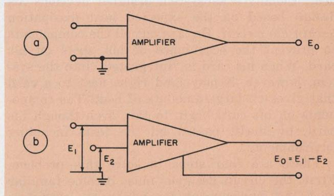
3. Input-signal noise is often a problem in a single-ended amplifier (a). Thus, while a subsystem test may show that a single-ended amplifier is adequate, a differential amplifier should be considered in anticipation of possible high-level noise in the system (b).
