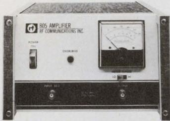
Model RF-805 is a solid-state amplifier with -30 db harmonic and intermodulation distortion. Gain is 47 db minimum, constant within 1 db for full output with less than 0.1 volt at 50 ohm input.
