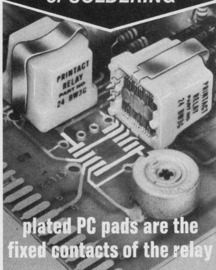
**plated PC pads are the fixed contacts of the relay**
