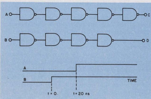
4. A simple example requiring a guaranteed timing relation of  $t_d \geq t_c$ , the basic network consists of NAND gates. Gate delays are 10 ns to 20 ns; delay lines have  $\pm 10\%$  tolerances. The minimum delay to be added to D, neglecting tolerances, is 80 ns.
