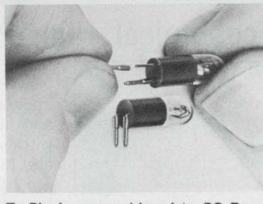
**Tu-Pin Lamps soldered to PC Board Unplug for Replacement.** When the lamp must be replaced, it is simply unplugged, leaving the gold plated pin sockets behind firmly soldered to the PC board and ready to receive a replacement. Hudson Lamp Co., Kearny, N. J. (201) 997-1850.
