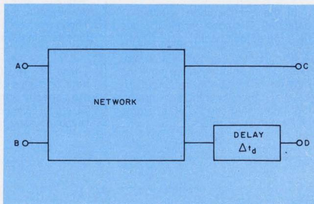
2. Introducing a delay in one path is the easiest way to obtain the  $t_d \geq t_c$  criteria. The delay can be determined by assuming a worst-case delay, tuning one path or tuning both paths. The last option provides the least delay to signal D.
