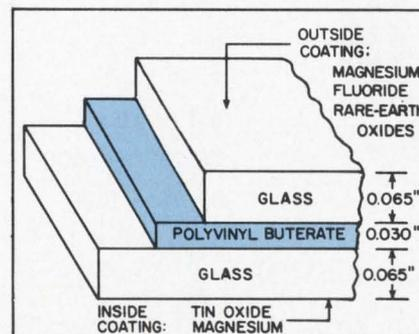
CRT faceplate is a sandwich of blue-green polyvinyl buterate between two pieces of coated glass.
