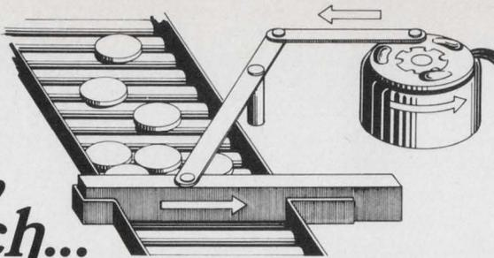
To move a load in an arc or a straight line
