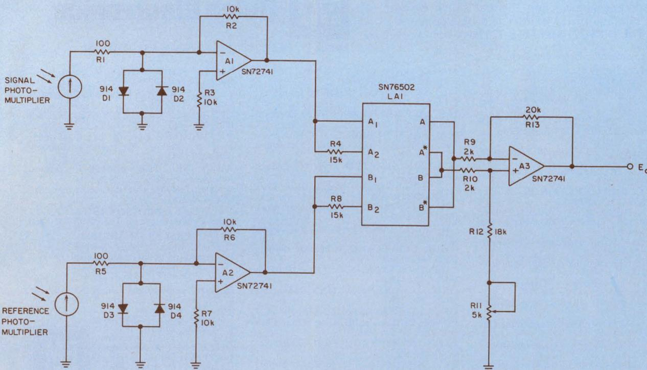
A low-cost, wideband (40 MHz) log amp (LAI) enables the circuit to achieve a faster and more accurate response than the usual design employing
