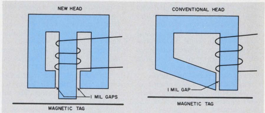
**Double-gap magnetic recording head** gives an accurate recording with up to 45° angular displacement or tilt from the data line. Present recording heads work only with about 15° of angular displacement and about 10° of tilt.
