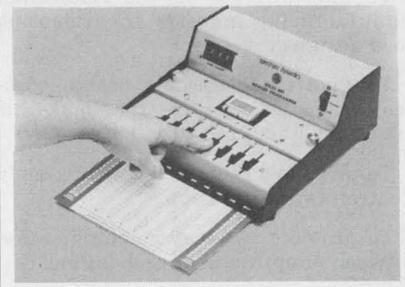
**Program all fusible-link programmable ROMs** manually with the Model 300. Designed with a 4096 bit (512 words x 8 bits) capacity. Both 115 VAC and 220 VAC versions available. Spectrum Dynamics, Inc., 2300 East Oakland Park Boulevard, Ft. Lauderdale, Florida. Phone (305) 566-4467 or 566-2547.
