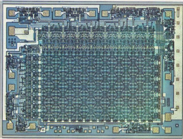
**Bipolar RAM** with 256 one-bit words, the 93410, is the first product to use Fairchild's Isoplanar oxide-isolation process to boost on-chip bit density.
