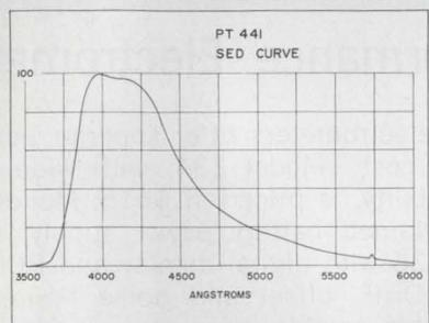
**New fast decay CRT screen.** A new long life phosphor screen is available with a decay time of 80 nano-seconds and with an efficiency substantially higher than standard P-16. Available in a wide variety of CRTs for scanners and readers. Thomas Electronics, Inc., 100 Riverview Drive, Wayne, N. J. Phone: (201) 696-5200.
