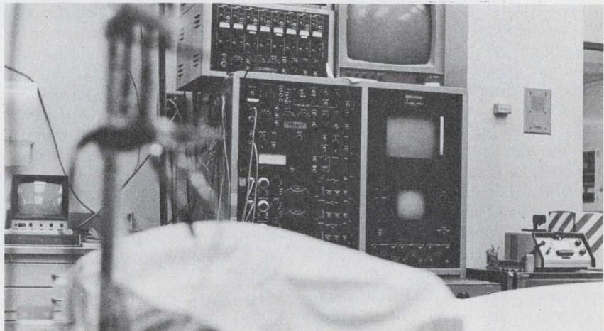
locations in the patient's cardiovascular system. For example, programs can perform a complete pattern recognition on left or right ventricular pressures, right atrial pressure, and aortic pressure. These programs take the raw pressure wave from the appropriate heart chamber, analyze it, pick out its important points and present the results to the cardiologist on the keyboard display shown at left.
