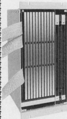
Now heading your way—a brand new breed of memory system hot on the computer market. It's Toko's high-speed, woven plated-wire memory system, HS 150. Dual-designed to operate on the non-destructive readout mode, it can be used partly for random access, read-write memory and partly for read-only memory.
