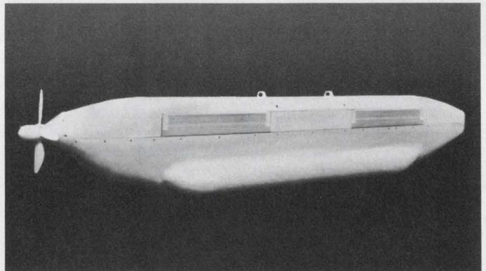
Garrett AiResearch enclosures are also cooling the pod mounted ALQ-76 and ALQ-99 electronic countermeasures systems. The enclosure in the ALQ-99 pod (shown above) for the EA-6B utilizes surface heat exchangers as the ultimate heat sink.
