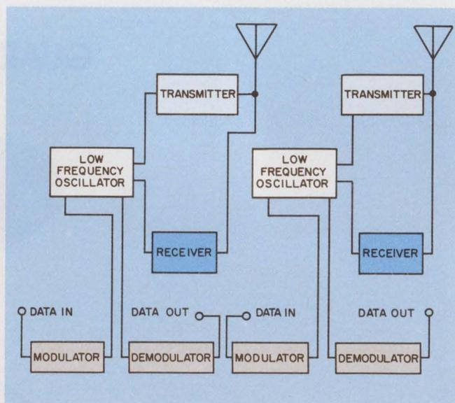
2. Adding a modulator and a demodulator to the basic repeater allows each station to originate and receive data as well as relay it. Data can be sent between any and all of the stations in the network.
