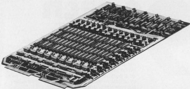
**The Compleat MOS Memory Card. 73,728 Bits. With Address, Data, Refresh and Timing Logic. Single Unit Just \$1859.**
