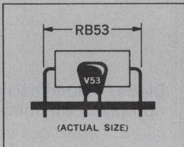
Size comparison between V-53 and RB-53 type wirewound. Vishay V-53 requires only 1/8 the space needed by the RB-53.
