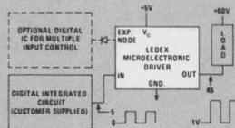
With the LMD-5 you can switch up to 325 watts. It has an expander node terminal, so you can add multiple inputs. An internal diode protects the circuit from damage when driving inductive loads.
