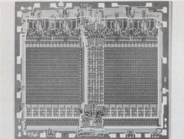
The first erasable field-programmable ROM, Intel's 1601 on a 147 X 161-mil chip, can be erased by exposure to ultraviolet light, then reprogrammed.
