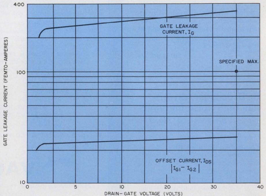
A new family of monolithic JFET duals features devices with ultra-low leakage and offset currents down in the femto-amperes region. These new JFETs can handle drain-gate voltages as high as 35 V with no input current degradation. Drain current for the above curves was set at 100  $\mu\text{A}$ .
