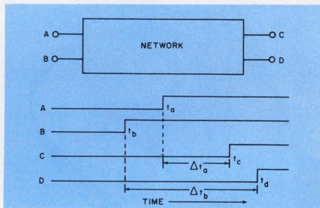
1. Obtaining  $t_d \geq t_c$  while minimizing time delays at the output is the objective in guaranteeing signal timing relationships. The required timing relationships are defined for output signals C and D, which are responses to inputs A and B, respectively.
