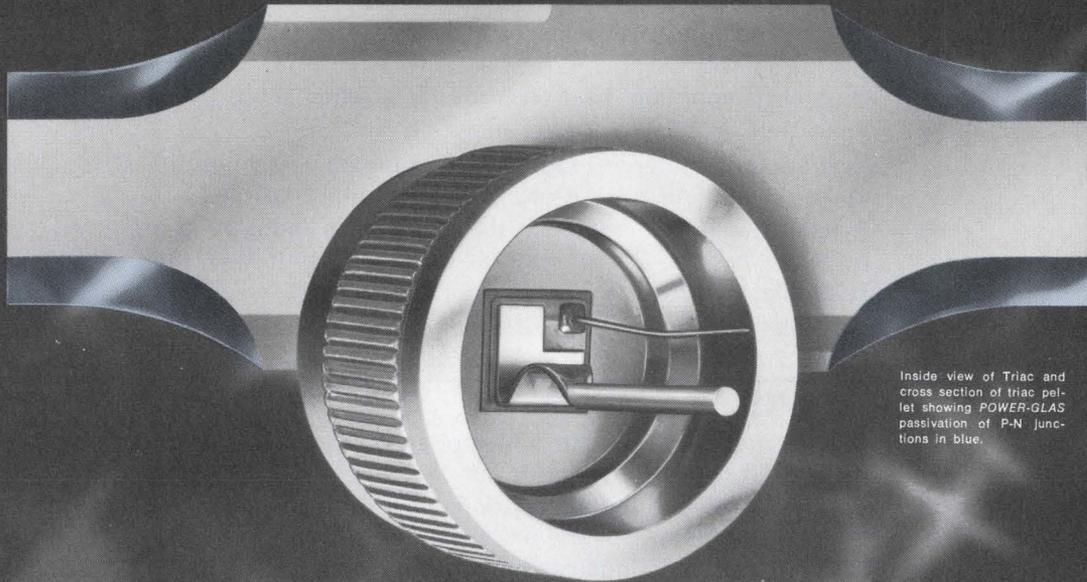
Inside view of Triac and cross section of triac pellet showing **POWER-GLAS** passivation of P-N junctions in blue.
