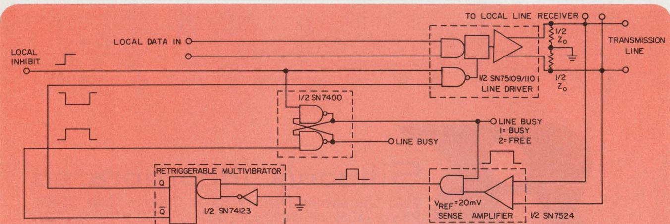
The local driver is prevented from transmitting in this party-line control until the line is free. The
