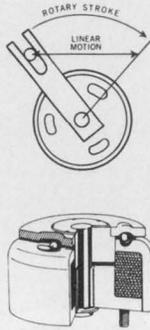
The Ledex rotary solenoid starts off working where the force is really at, about .030" between the pole faces. Then the armature rides a helical ramp, to distribute the force over the stroke you need. It gives you efficient, direct rotary action and uniform linear movement.
