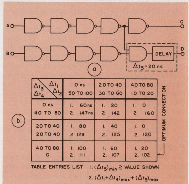
6. The hybrid technique of method 3 results in the optimum connection shown (a). A table giving all possible connections (b) lists each in terms of the criteria of method 3. The delay  $\Delta t_5$  is a variable used to solve the inequality  $[(\Delta t_4 + \Delta t_5)_{\min} \geq (\Delta t_2)_{\max}]$ . The optimum connection has least over-all time delay.
