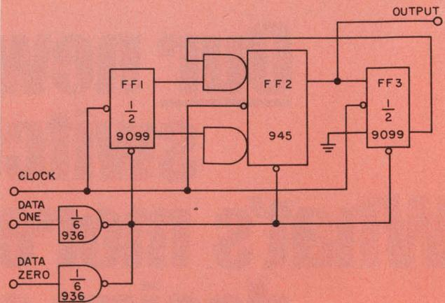
**Three flip-flops form the basis of a blank detector.** The circuit requires additional flip-flops when the external clock rate is significantly different from that of the internal clock.
