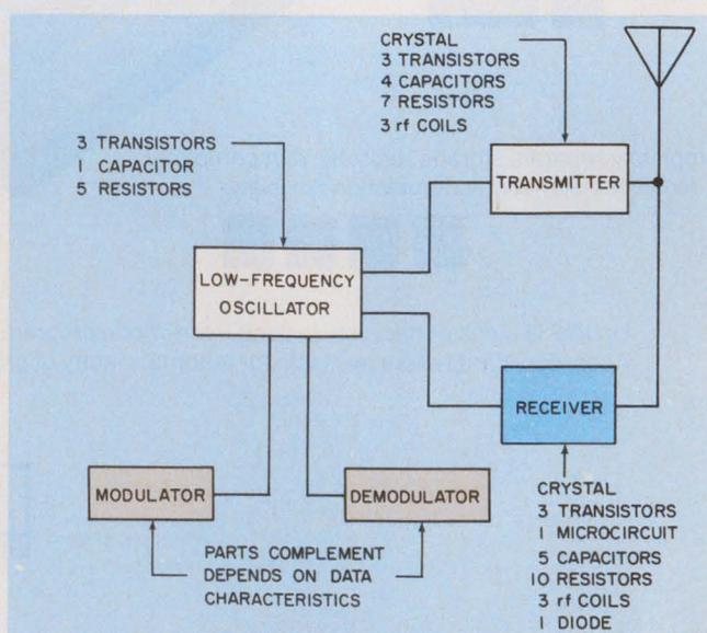
4. Station design is uncomplicated and inexpensive. The design details will vary with the system designer, but the parts complement should be approximately as indicated in this typical-system example.
