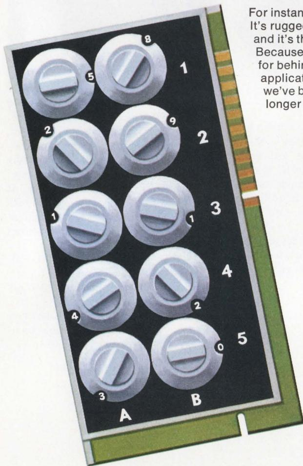
For instance, take our Rotary Matrix Switch. It's functional. It's rugged, easy to operate, positions with positive detent action, and it's the smallest available programming device of its kind. Because it's out of sight, beauty is not our intent. It's designed for behind-panel installations in semi-permanent programming applications. And because it's changed so infrequently, we've built in a life span that's as long as you'll need, probably longer than the equipment for which it is intended.
