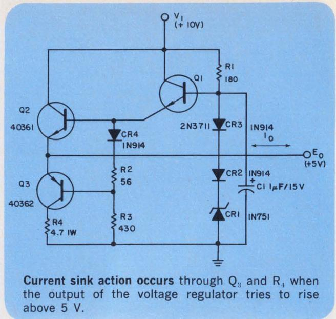
current through  $R_1$ . For the circuit values shown, the output voltage is 5 V, and the supply can sink up to 100 mA of current.
