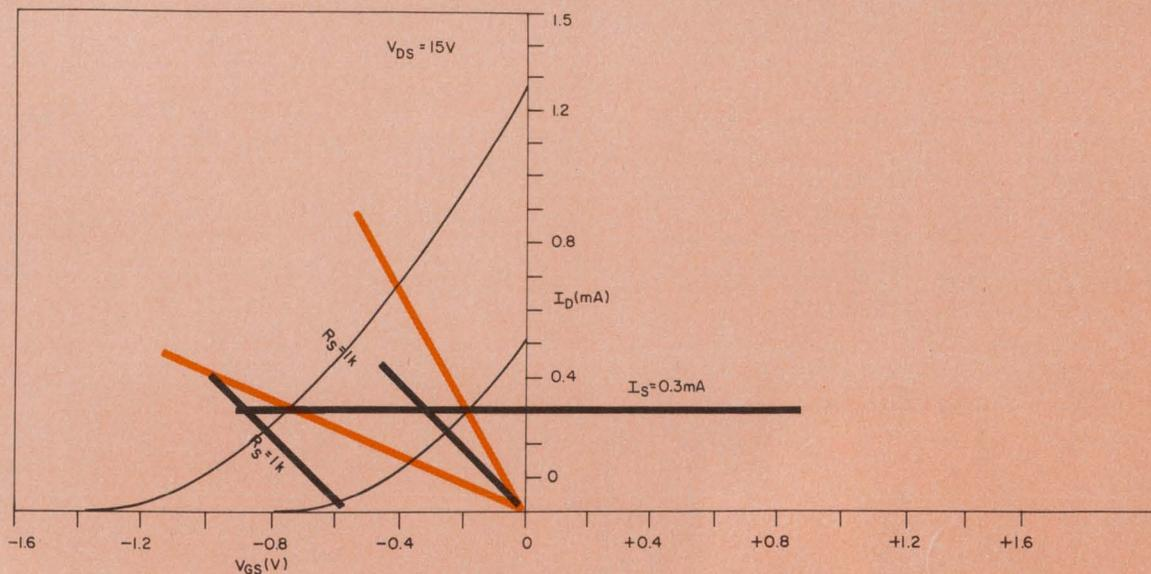
8. If  $R_s$  isn't trimmed so that the load line passes through the origin, a voltage will appear at the gate
