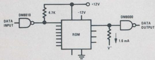
Application briefs have been written to describe a character generator system or a delay line application that mixes the two worlds. By using a ROM for micro-programming, code conversion, character generation, table lookup and so forth, a system becomes fewer and fewer components. In fact, any random logic function that can be expressed in a truth table can be programmed into a ROM. Just try it.
