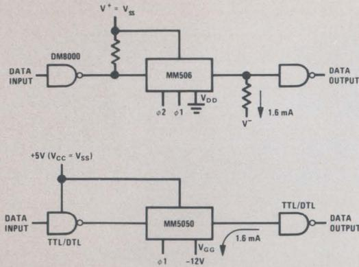
This form of interface can even be used to improve the operating frequency of MOS devices. When the MOS shift register is driving TTL, the total signal swing from a logic "0" to a logic "1" is reduced, hence the delay time is minimized. A long serial delay line, consisting of 1 MHz operating frequency shift registers, can be made to operate at 2.0 MHz by this method.
