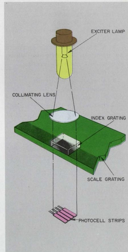
**Moiré fringe systems** convert small linear motion into greatly magnified optical signals. This system can detect 0.0001-inch imperfections.
