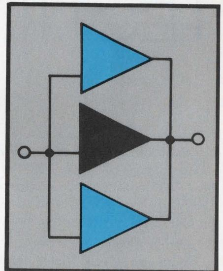
When good op-amp reliability is not enough—when you need ultra-high reliability—special summing circuits can be the answer. A redundant amplifier (RAMP) connection of several op amps can continue to operate satisfactorily, even after one or more of the amplifiers fails.
