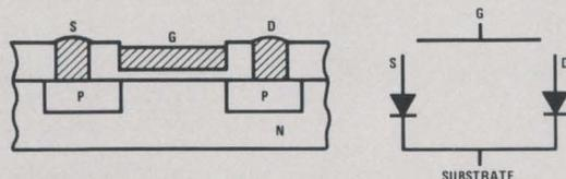
induced between these two junctions to cause operation. The electrical symbol shows the device to be no more than two diodes with a common cathode. The junctions are used merely as contact points for the Source and Drain. If forward biasing occurred without current limiting, the junctions would be destroyed. As long as the substrate remains more positive, the diodes never become forward biased. The gate is electrically isolated by a thin oxide layer.
