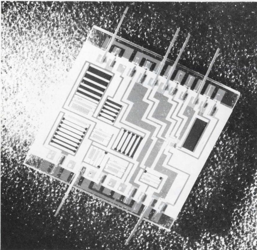
**All-purpose second-order filter building block** uses thin film components. Scribe points on the circuit allow the selection of any filter function.
