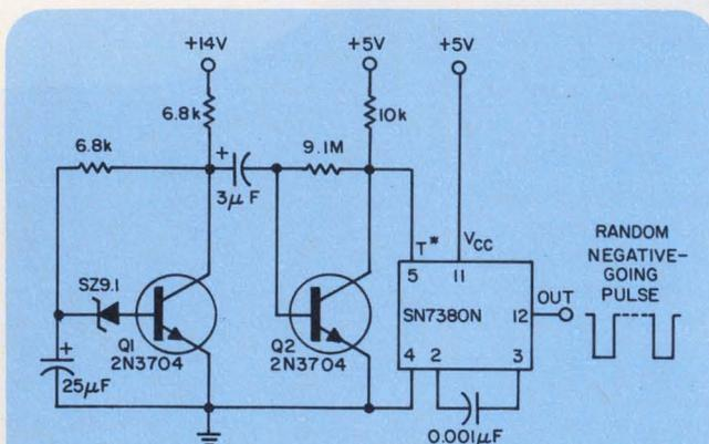
Random negative pulses from the monostable multivibrator are triggered from a combination noise generator/amplitude discriminator.
