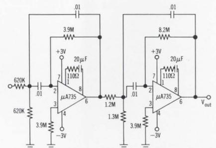
This circuit has a center frequency at 10 Hz, 12 dB rolloff with -3 dB points at 6.5 Hz and 14 Hz. The  $\mu A735$  lets you use small capacitor values and large resistors for frequency shaping at a few Hz, due to the  $\mu A735$ 's low input offset current.
