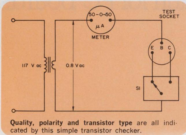
under test is considered defective; that is, it is either open or shorted. If the junction is good, the meter will immediately deflect to one side or the other of zero, depending on whether the device under test is an npn or a pnp.
