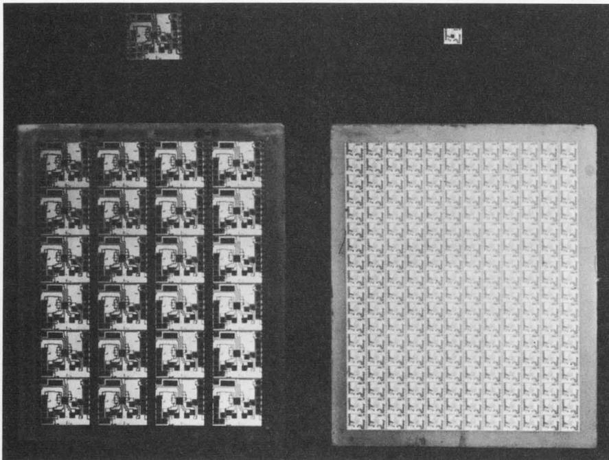
**Using present technology**, tone generator (left) has 24 circuits on a standard substrate. With future technology, the same substrate (right) has 216 of the same circuits based on predicted component miniaturization.
