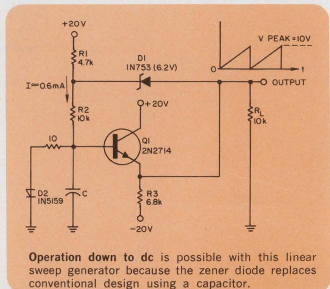
Operation down to dc is possible with this linear sweep generator because the zener diode replaces conventional design using a capacitor.
