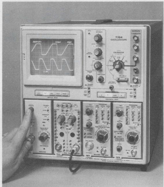
The Readout System presently displays up to 49 symbols and responds to various functional instructions. Less than half of the symbols are needed for today's plug-ins.
