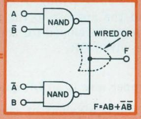
5. An exclusive-OR function at a one-gate saving (a), and a two-input coincidence detector, also at a one-gate saving (b), from NAND/wire-OR.
