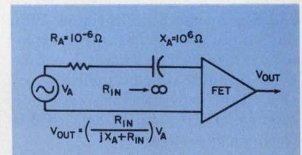
2. Equivalent circuit of the mini-antenna for a 1-meter stub at 20 kHz.
