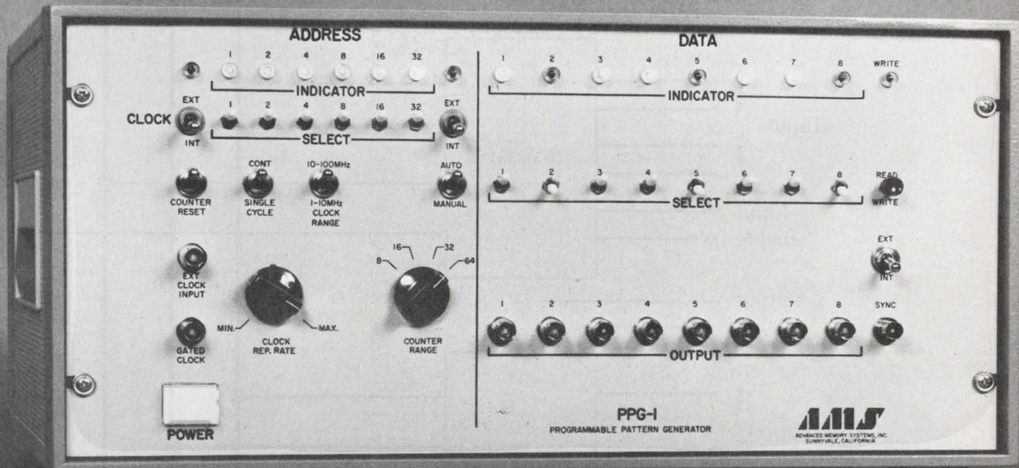
Program pulse position and pulse width from your computer *or* from the front panel. Once the program is set, the PPG-1 can provide data outputs in 10 nanosecond increments. Eight channels, sixty-four bits per channel. DC to 100 MHz clock rate. 1.5 nS rise and fall time. *That's a Pattern Generator:* Advanced Memory System's PPG-1
