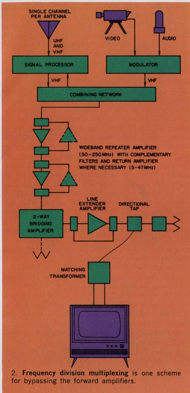
2. Frequency division multiplexing is one scheme for bypassing the forward amplifiers.
