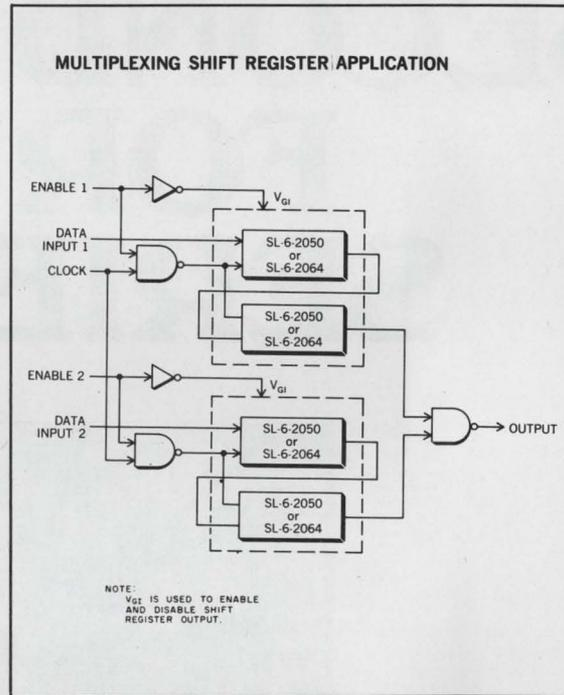
Among their various and marked advantages over bipolar and delay line serial storage systems, General Instrument's GIANT Dual 50-bit and Dual 64-bit DC shift registers operate with the lowest power dissipation available for static registers . . . a mere 7 milliamps typical.
