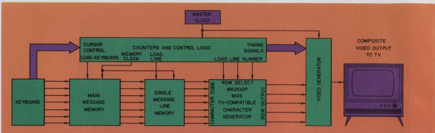
**3. Mostek technique** for connecting a standard keyboard to a TV set. An MOS 2240-bit, read-only memory func-
