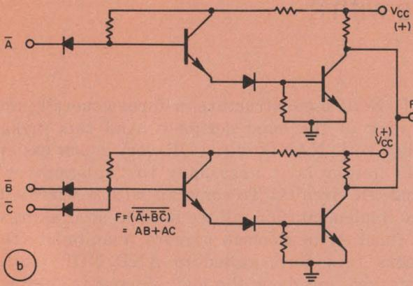
2. The basic 930 DTL NAND gate (a) gives a LOW output only if all inputs are HIGH. A simple connection of the output leads of two of these gates (b) results in an additional OR function; the combined outputs is LOW if either output is LOW.
