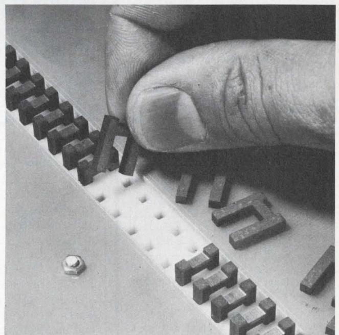
able U cores and I bars. The retainers for these components are plastic so that the retainers, instead of the components, are wrapped with the sense winding.
