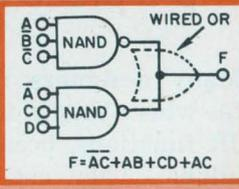
4. Significant savings in gate count result for some logic functions (a). In this case a simple NAND circuit requires five gates (b), but a simplified AND/NOR circuit uses three gates and a NAND/wired-OR equivalent uses only two gates.
