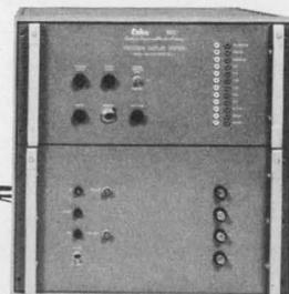
CELCO Precision Display Systems are completely self-contained X-Y monitors with wide bandwidth to 1.0 MHz, linearity to 0.1% and fast slew rates. These flexible
