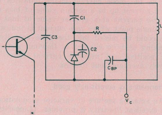
1. The modulation sensitivity of this fm oscillator tank circuit is most easily adjusted by changing the size of capacitor  $C_1$ .  $R$  should present an impedance many times larger than that of the varactor ( $C_2$ ) if it is to be omitted from the rf analysis of the circuit.
