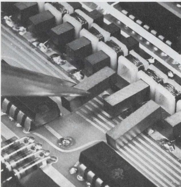
**Mechanically alterable read-only memory** puts its fixed-program format on plug-in PC boards. In addition, memory downtime is minimized because of easily replace-
