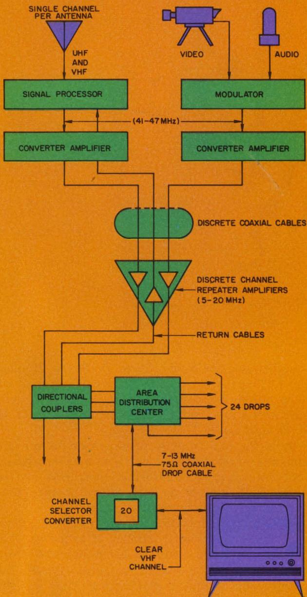
1. In the Discade system each channel is carried on a separate cable at reduced frequency.
