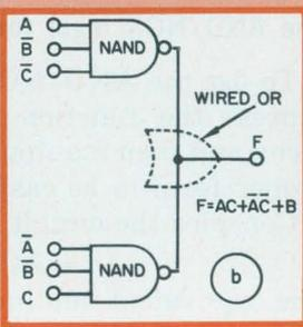
3. AND/NOR (a) and NAND/wired-OR (b) gates perform equivalent functions if connected in similar patterns. The designer performs Boolean calculations to minimize the gates in an AND/NOR system; then he replaces AND gates with NAND gates, NOR gates with the wired-OR connection.
