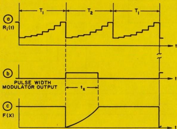
24. Simulated arc-tangent derivative (a) is switched to integrating counter by pulse-width modulator signal (b). Counter content (c) approximates arc-tangent function over period  $t_x$ .
