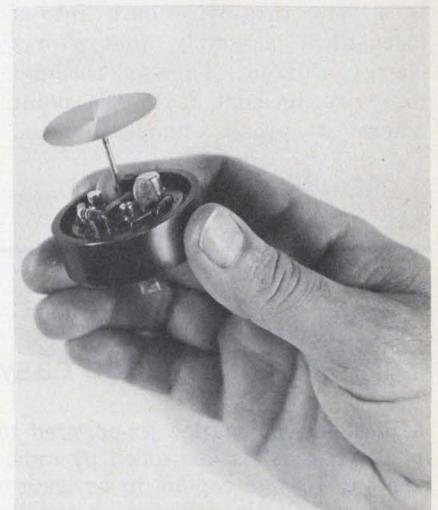
A disc-topped rod plus electronics make up the Voltage Probe Antenna
