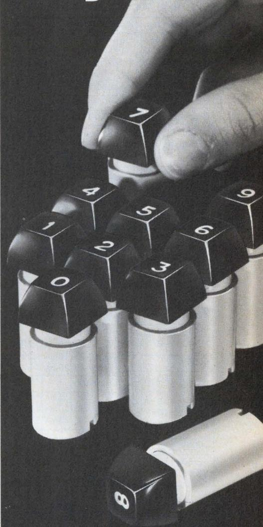
Build your own keyboard by using new ALCOSWITCH Keyswitch Modules. A highly reliable reed and magnet combination is employed to provide extremely long life and a low operating force simulating the action of a fine electric typewriter. Modular switches fit into standard 3/4" centers and have a 10° slanted base for "step up" key formation.
