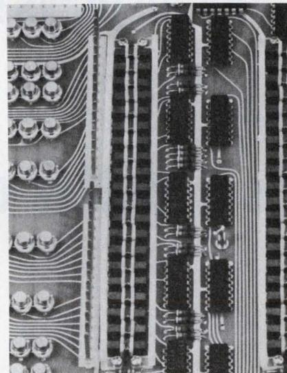
A new read-only core memory, which can have its program altered without being returned to its manufacturer, offers capacities to 20,480 bits at a cost of only 2.5¢ per bit. Called the VROM, it has a mechanically interchangeable braid and diode board, thus permitting users to maintain a library of plug-in fixed-program tables.
