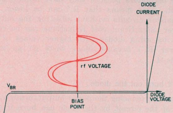
4. Both forward and reverse currents can flow concurrently if the p-p rf voltage swing exceeds  $V_{BR}$ .
