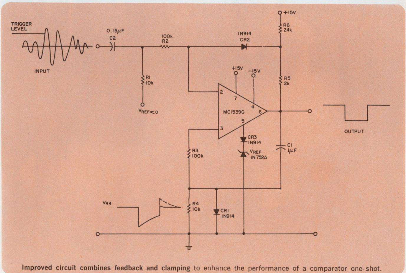
Improved circuit combines feedback and clamping to enhance the performance of a comparator one-shot.
