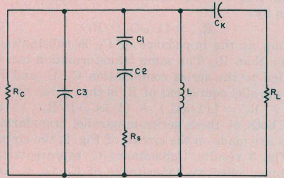
2. The effective series resistance,  $R_s$ , of the diode should not be neglected when analyzing the loaded tank circuit.  $R_C$  is the effective shunt resistance of the transistor,  $R_L$  is the load and  $C_K$  couples the load to the oscillator. Only rf components are shown.
