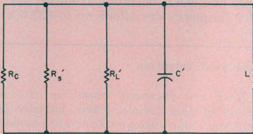
3. Power output suffers as  $R_s'$  is decreased. The primes indicate parallel-equivalent transformation.
