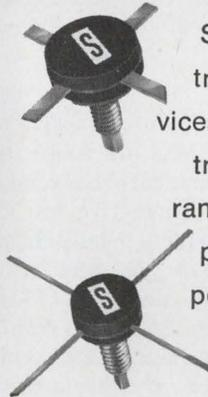
Solitron's wide range of RF power transistors can provide the right devices for your required applications. These transistors cover a useful frequency range from 40 to 1000 MHz and output power levels of 1 to 30 Watts. All popular package types are available. Take your pick from Solitron's power frequency spectrum and contact us today.
