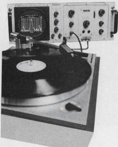
The spectrum analyzer with an **AL-2** module is often used in audio distortion measurements. Amplitudes of all frequency components in the scanned spectrum are simultaneously displayed for rapid analysis. Typical of its applications are measurement of IM distortion in transducers such as phonograph cartridges. IM products are displayed as side bands on a recorded carrier.
