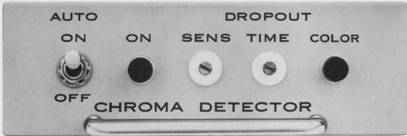
What KTTV, Los Angeles, says about Cohu's new chroma detector . . . "The Cohu chroma detector enables us to run the highest quality monochrome film on a color chain, eliminating the need for duplicate equipment. This means color and monochrome film can be interspliced without concern."
