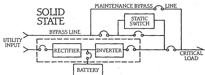
to 600 KVA. Six or more modules can be paralleled to increase ratings to 3600 KVA and beyond, building in fail-safe redundancy.
