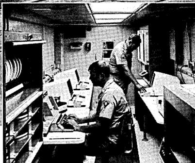
GE provides the Army with low-cost, reliable mobile data processing facilities for its Decentralized Automated Service Support System (DAS3) program. DAS3 utilizes standard commercial computers and programming, ruggedized and environmentalized to meet military needs for transportability. DAS3 units are operated and maintained by Army field personnel with minimal training.
