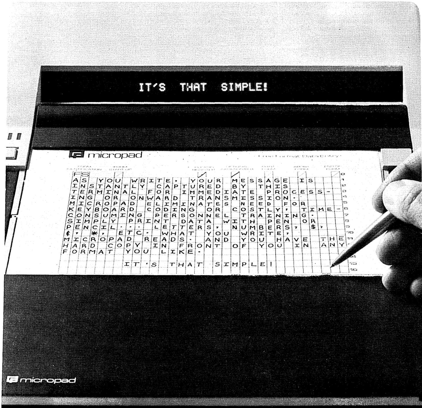
Brokers, bankers, accountants—from a factory foreman entering work in process to the chairman of the board accessing financial data—anyone can become a computer user with Micropad. Immediate feedback and data recall are provided in the integral display. Corrections are simple—just write over the character to be changed.
