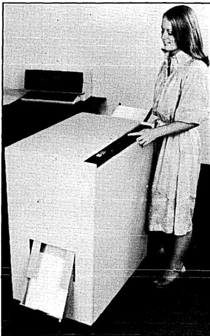
paper path and a stationary scanning head. Instead of moving the head across the page, a drum containing focusing lenses rotates at 1,800rpm, directing a light source onto the page, and redirecting the reflected character image from the page to a light-detecting sensor fixed at the central axis of the rotating drum.
