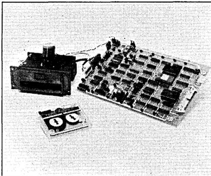
that uses the 3M DC100A minicartridge. The drive records up to 168KB on each of two tracks and transfers data at a rate of 1.8Kbps.
