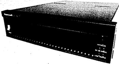
Just announced in February, the new entry-level member of the Honeywell Level 6 family, the Model 23, is designed for end user applications. Shown here in rack-mountable form, it is also available in prepackaged "minimount" and workstation crt versions.
