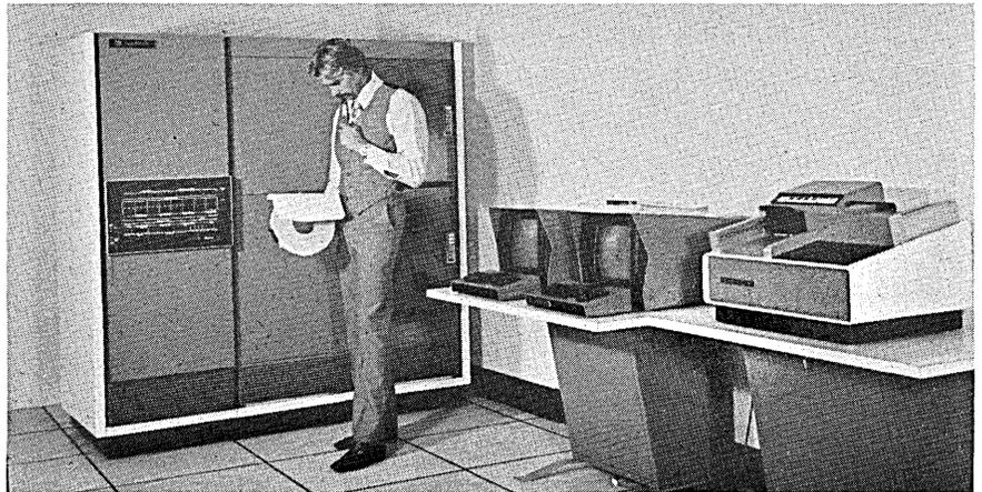
Harris Computer System's line of midicomputers began life as Datacraft models. Shown here is the S220 cpu. The Harris line is unusual in that it uses a 24-bit word rather than one of 32 bits, and that it is optimized for double-precision floating point arithmetic (in fact, single-precision results are obtained by discarding the least significant 24 bits from double-precision results).
