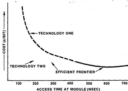
Fig. 5. Some 37 inputs to the model are non-scalar, including the relation of memory cost to performance (which is fed to the model as a function, and which assumes the use of the most efficient technology).
