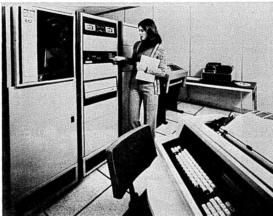
The Interdata 8/32 is the only computer in this class which currently supports user-programmable writeable control store. The machine also has four specialized instructions which allow the user to set up any number of circular lists in memory for stack or queuing operations.
