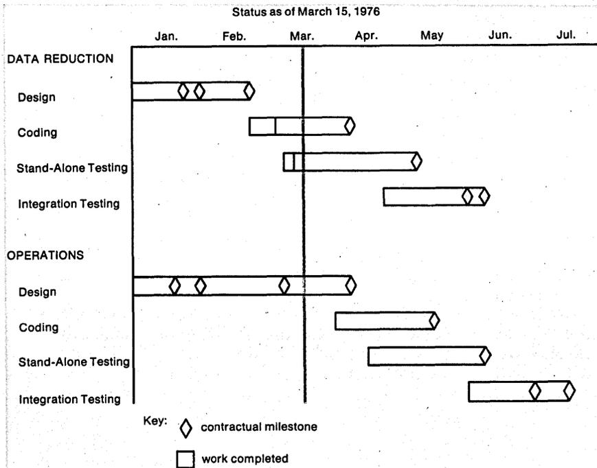
Fig. 1. A Gantt chart is useful for assigning production schedules, but a drawback is that on any particular day it is unclear whether a specific task, which may proceed at a nonlinear rate, is on schedule or falling behind. Such bar charts are then of little use for warning managers of potential problems.
