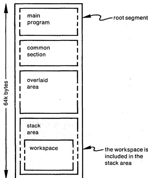
Fig. 1. The basic problem in converting to a mini is space, of course. It drives the designer to walk a tightrope between excessive disc accesses and core overflow. The above shows how a typical SPSS job was laid out.
