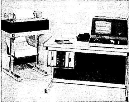
DynaTermDisk, 8K of random access memory expandable to 64K, a virtual memory editor, and two RS-232C ports for interfacing a terminal and line printer. The standard software includes
