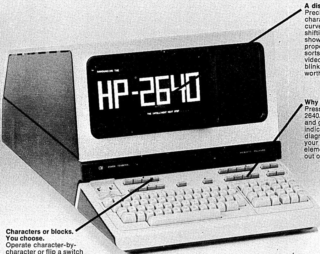
**A display that people like.** Precise. Crisp, with 9 x 15 dot character cell. Character curves are smoothed by dot shifting. The 5" x 10" screen shows characters in their proper 2x1 aspect ratio. All sorts of options, such as inverse video, underlining, half bright, blinking, because a picture's worth a thousand words.
