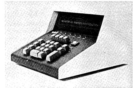
even Correspondence codes optionally available. Other options include formatting and interfaces to cassettes, printers, floppy discs, or other similar devices. Delivery is quoted as 30 days, depending on specific functions required. The TR-10 is also available without the gas discharge display feature. VMF INDUSTRIES, INC., Bay Shore, N.Y.
