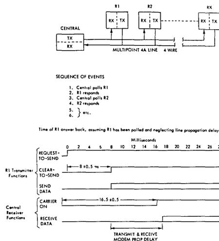
Fig. 4. Many of the Los Angeles County modems had to operate in a polled environment. This plot shows the timing sequence of a polled four-wire multipoint system. The remote site starts the sequence by raising Ready To Send signal. The central site master responds 8.5 msec later with a Clear To Send.
