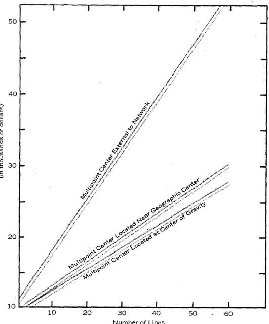
Fig. 1. A \$25/run network optimization program written in GPSS/360 was used to compare the operating costs resulting from various node placements in this 60-terminal network.
