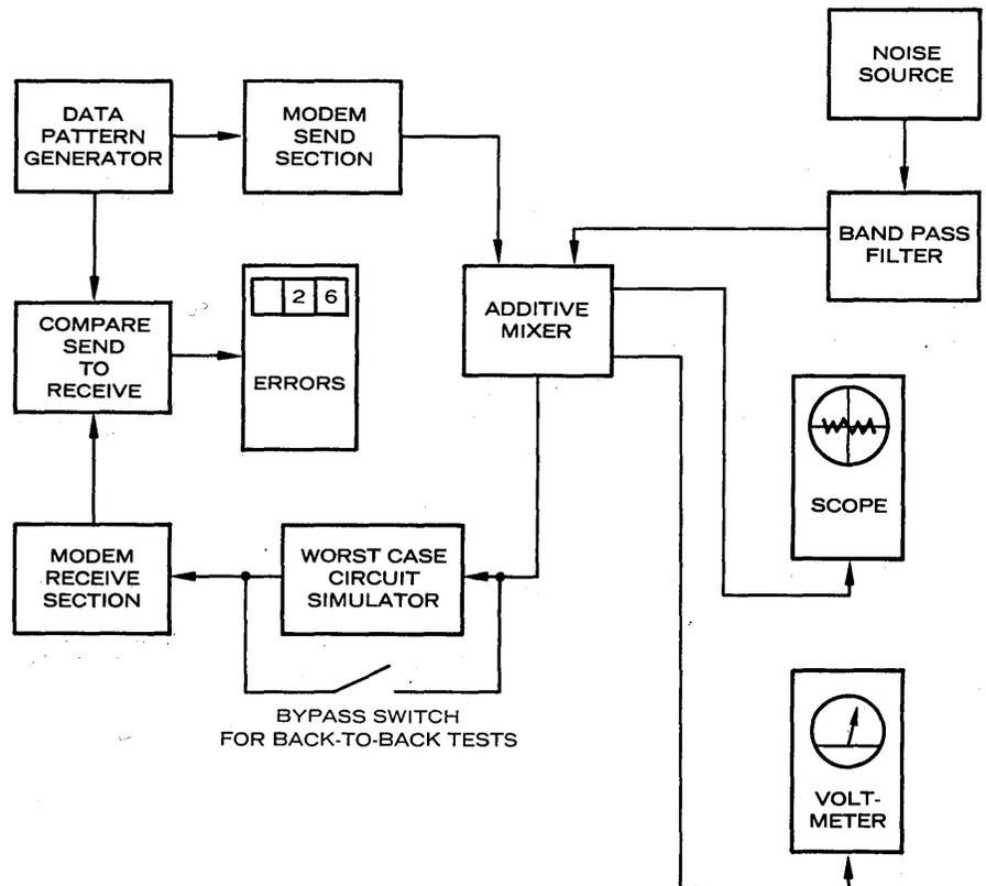
Fig. 1. This test setup was used to determine operating characteristics under various signal-to-noise conditions.
