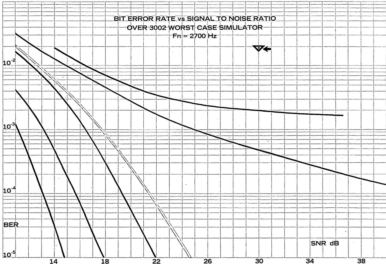
Fig. 2. Tests conducted with the worst case line simulator separated the modems by how well their line equalizers worked. The best curve is on the left. The Bell 201B equivalent is the
