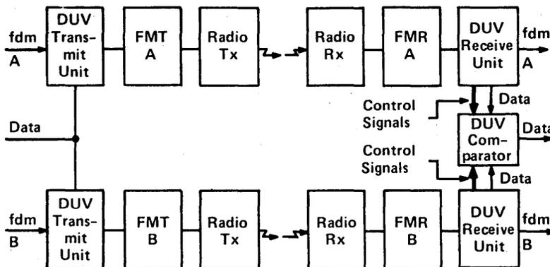
**PARALLEL DUV:** In this one-for-one protection configuration, two frequency division multiplexed signals and one 1.544 Mbps data signal are transmitted over two working radio channels. The comparator equipment then selects from the two decoded bit streams the one that has no bits in error.
