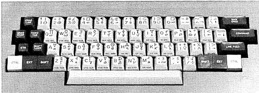
Fig. 1. An eight-bit code makes a 256-character set possible, but a keyboard for that many characters is intimidating.
