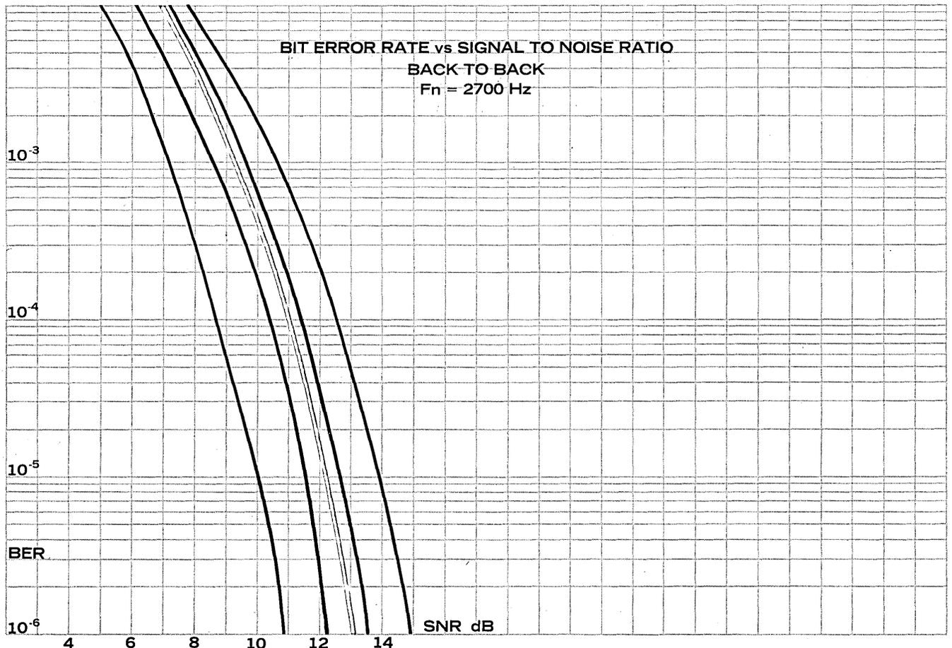
Fig. 3. The five brands of modems not eliminated by previous tests were then run in pairs, back-to-back. Although the curves look fairly close, the 201B modem, the middle line, is shown
