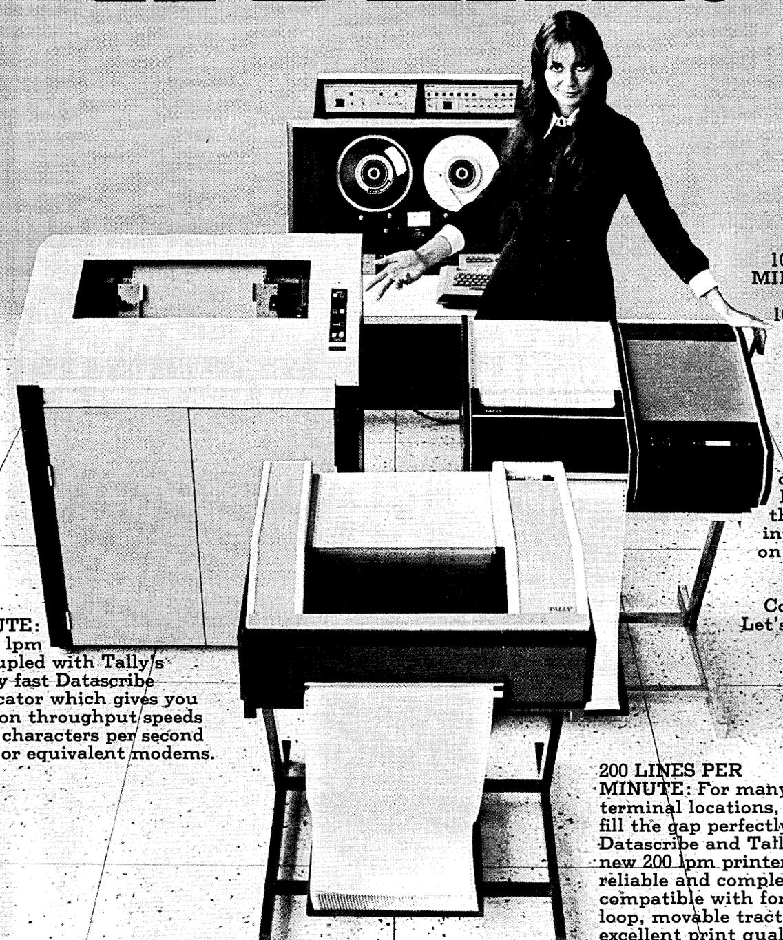
**600 LINES PER MINUTE:** Tally's 600 lpm printer coupled with Tally's exceedingly fast Datascribe Communicator which gives you transmission throughput speeds up to 1200 characters per second using Bell or equivalent modems.
