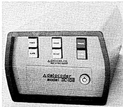
trillion unique code formats are possible in this version, which can operate over dial-up and dedicated phone lines, and even microwave links. The speed of the DC-110 is given as 100,000 baud through tty or RS-232 interface. Prices for the DC-108 and DC-110 are \$2950 each—and don't forget that you need at least two of them. For information:
