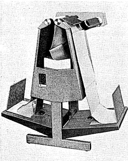
the open front design has been restyled to permit easier threading of form webs. Magnetic backstop plates allow location of form depths. Tines of carbon rewind forks have been connected into "U" sections to prevent operator injury. Speed of the decollator is variable, from 50-350 feet per minute; handling paper of 10-110 lb. substance. MOORE BUSINESS FORMS, Niagara Falls, New York. For information:
