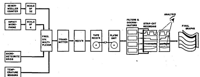
age of the micrometeoroid grids. This very simple system employed very little on-board data processing and very little machine processing on the ground, and was used in the first satellites to give a high probability of success at a time when instrumentation on satellites was still an undeveloped science, and when large volume data processing techniques on the ground were relatively unknown for this application.
