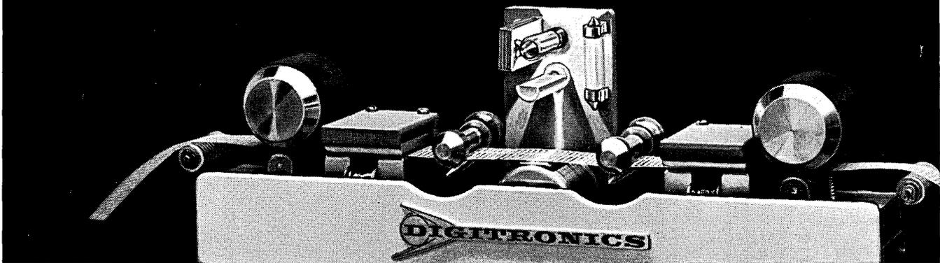
But even the light source in a Digitronics photo-electric perforated tape reader has extra-ordinary life. A source under test is still burning after 18 months. All's to say that you'll need very few replacement parts ever in a Digitronics reader. High derating factors on all parts and careful design insure continuous use.
