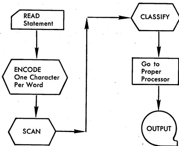
example of such a processor is the routine which processes COMMON, DIMENSION, and EQUIVALENCE statements. This processor records the name and order in COMMON of every COMMON variable; the name and length of every array, and all of the EQUIVALENCE information. All of this information is stored in tables for use during step two. Finally, the statement is written onto the intermediate tape.
