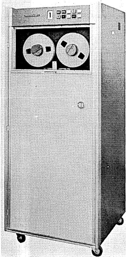
inches per second, and dual densities of 200 or 555.5 bits per inch. Start/stop times for the BC 422 are less than three milliseconds. BURROUGHS CORP., 460 Sierra Madre Villa, Pasadena, Calif. For information: **CIRCLE 204 ON READER CARD**
