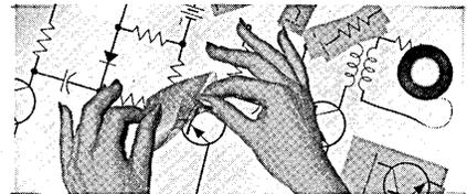
for displays and technical presentations. The product consists of all A.S.A. and I.R.E. electrical symbols, individually printed on self-adhesive transparent plastic. Select-a-circuit preprinted symbols are available in 2½" or 4½" lengths, and vary in
