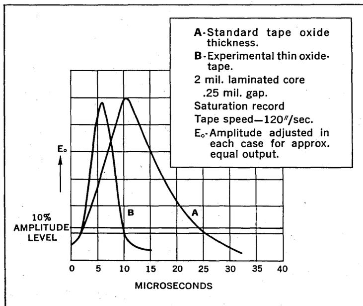
Pulse width comparison—standard and thin oxide tape.
