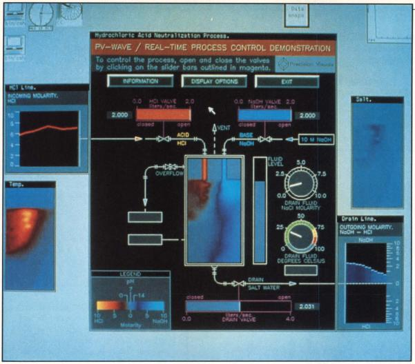
An external process used to neutralize acid outflow is monitored and controlled using **Precision Visuals' PV-Wave interactive** data analysis and display system. Input and output pH levels and flow rates can be controlled by interaction with the display. Other critical parameters of the process can be monitored in
