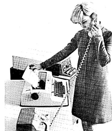
Controls on the telephone data set permit operators to hold telephone conversations, exchanging instructions or other information. They also allow documents to be communicated automatically when there is no operator in attendance.
