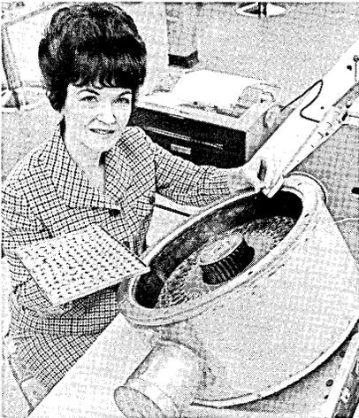
— Here, Dottie Henry begins to load a batch of dime-sized thermostats that control the heat level in computers, into an air heated "testing pot"
