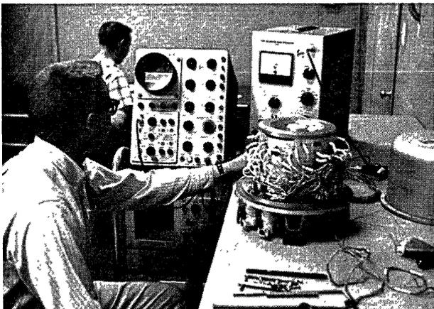
Conducting an acceptance test on a 6", 80 Track, 6000 RPM drum at Wheeler-Fairchild. Tests showed less than 5% modulation on all tracks. Made for U. S. Navy's "ASROC" project. Some other customers include .... Ramo-Wooldridge, General Precision Laboratories, Aeronutronics, Div. of Ford Motor Co.
