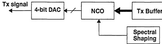
Figure 3. Modulator Block Diagram
