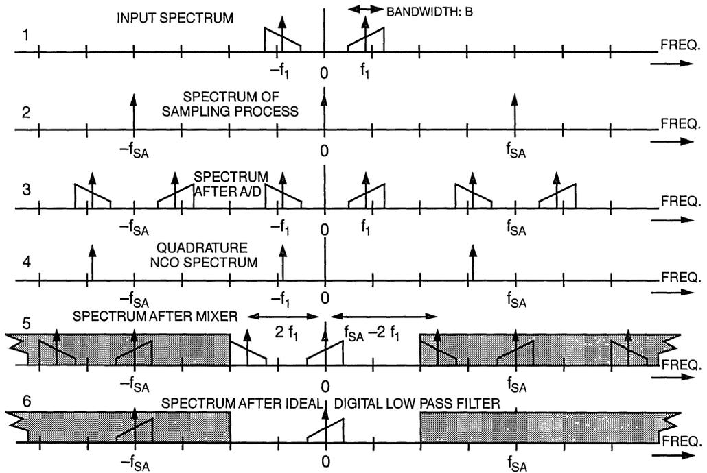
Figure 15. Spectra of Signals in Quadrature Sampling Mode
