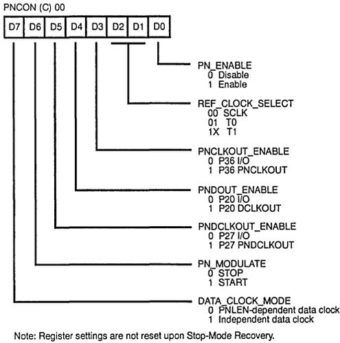
Figure 35. PN Modulator Control Register ((C) 00H: Read/Write)
