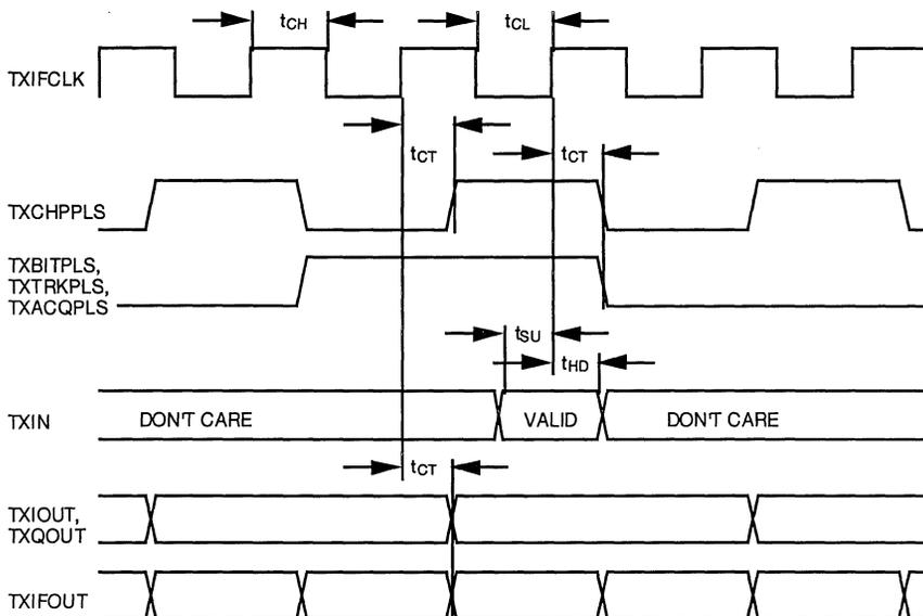
Figure 4. Transmitter Input/Output Timing
