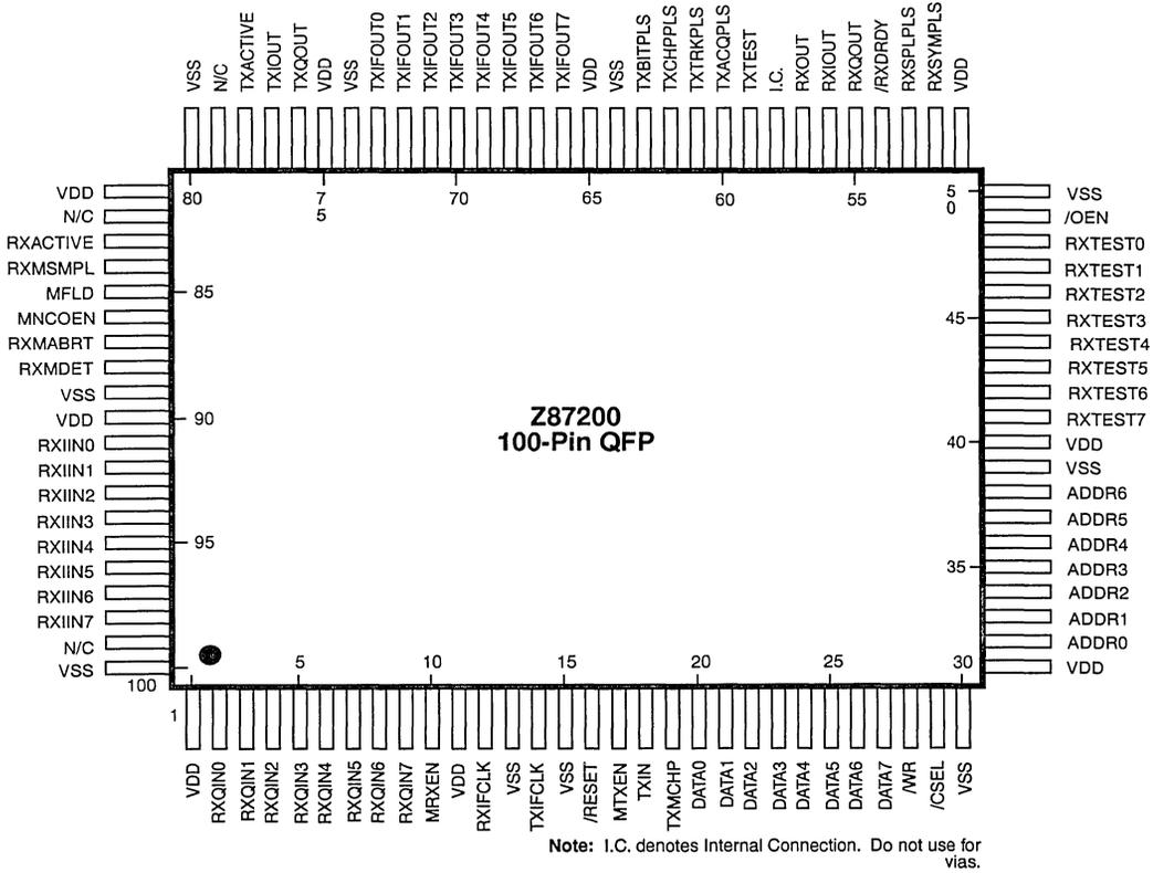
Figure 2. Z87200 100-Pin PQFP Pin Description
