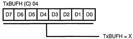
Figure 39. PN Modulator High-Byte Data Hold Register ((C) 04H: Write Only)
