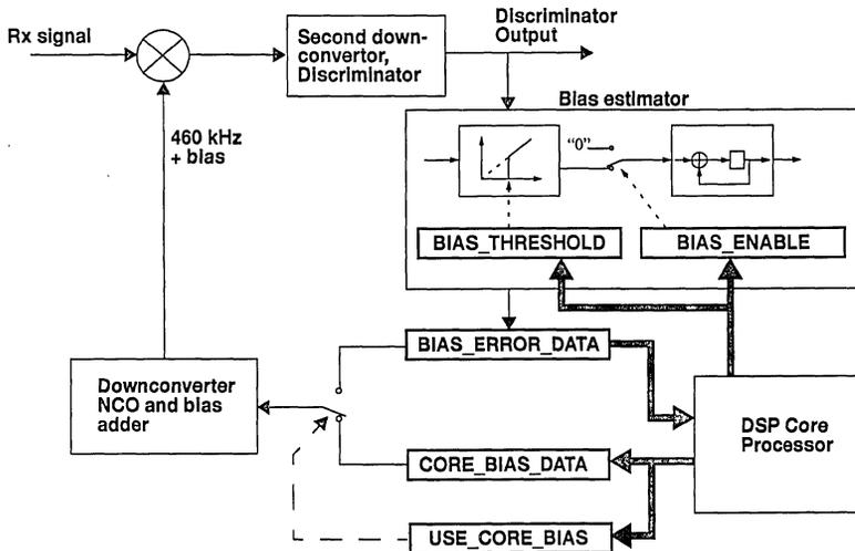
Figure 5. AFC Loop and Processor Control
