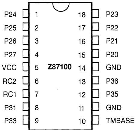
Figure 2. 18-Pin DIP/SOIC Pin Configuration
