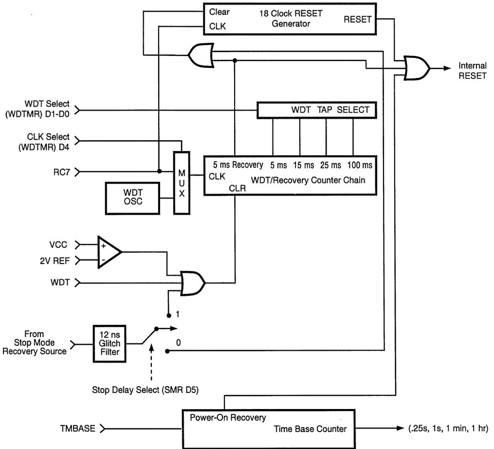
**Figure 24. Timing Recovery Circuit (POR, WDT)**
