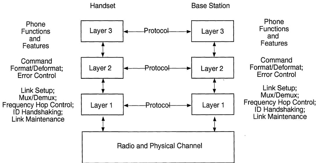
Figure 6. Signaling Architecture
