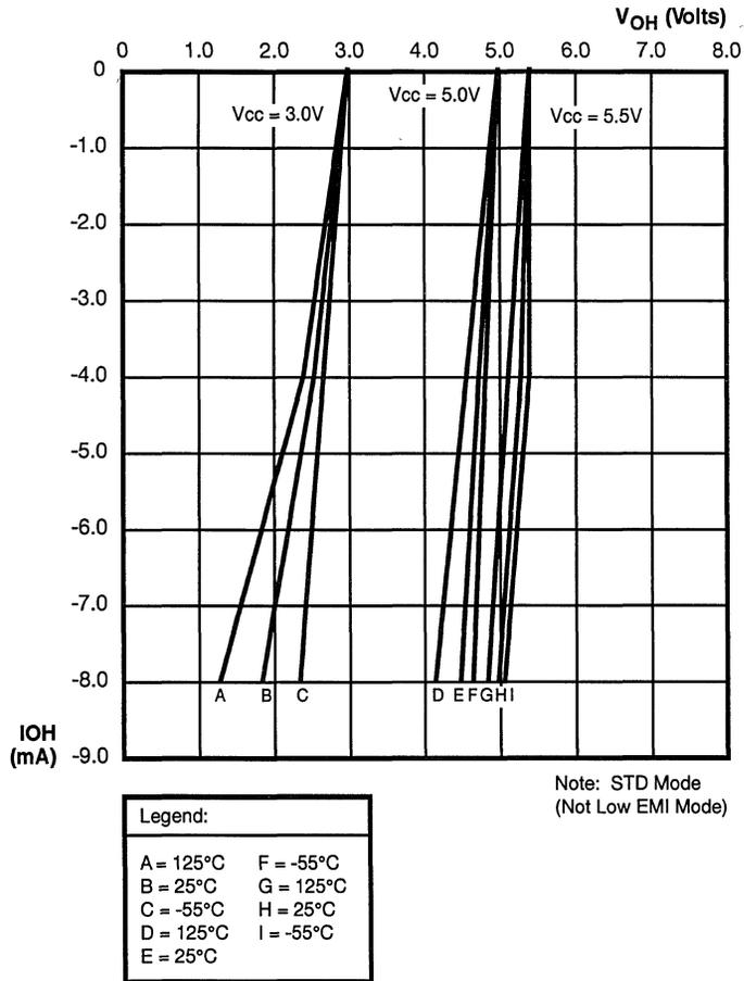
Figure 55. Typical  $V_{OH}$  vs  $I_{OH}$  Over Temperature
