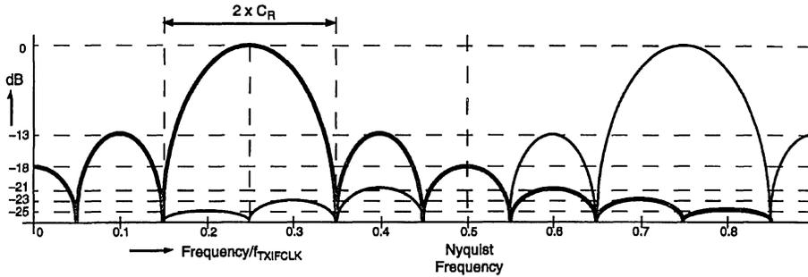
Figure 17. Spectrum of DDS modulated at  $0.1 \times f_{RXIFCLK}$  when carrier frequency is set to  $0.25 \times f_{RXIFCLK}$
