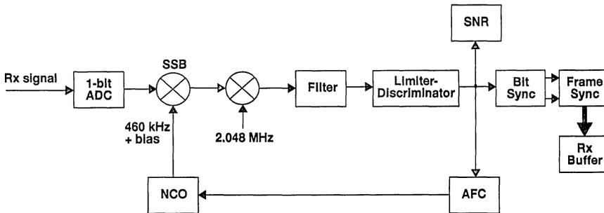
Figure 2. Demodulator Block Diagram
