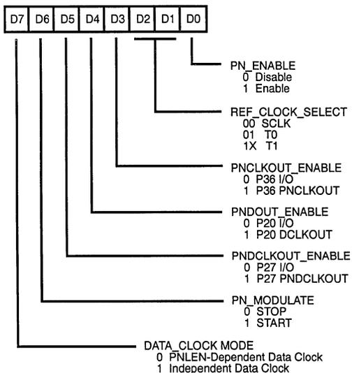
**Figure 18. PN Modulator Control Register (PNCON)**
