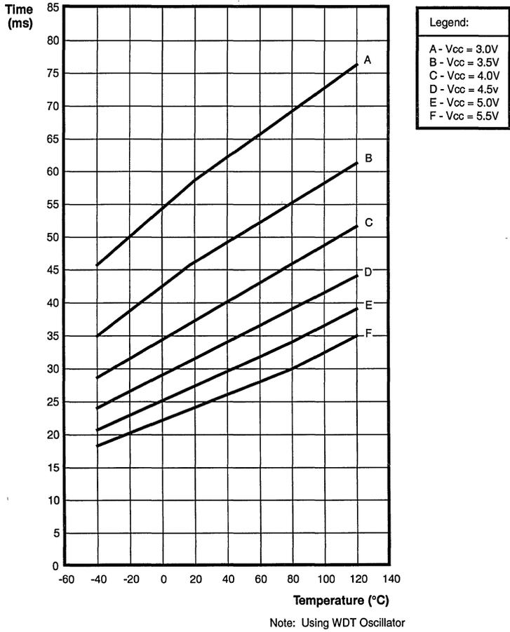
Figure 59. Typical 15 ms WDT Setting vs Temperature
