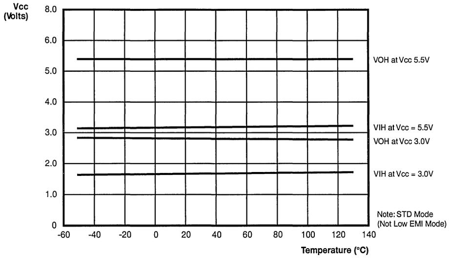
Figure 54. Typical  $V_{OH}$ ,  $V_{IH}$  vs Temperature
