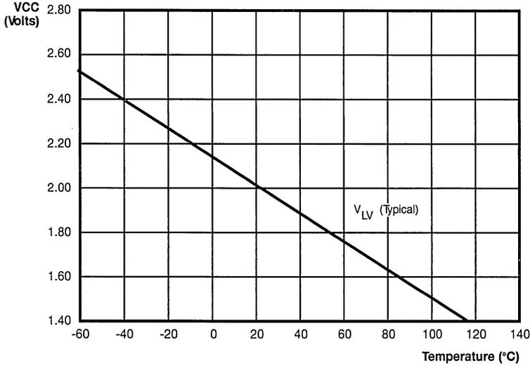
Figure 25. Typical Z87100 V<sub>LV</sub> Voltage vs Temperature
