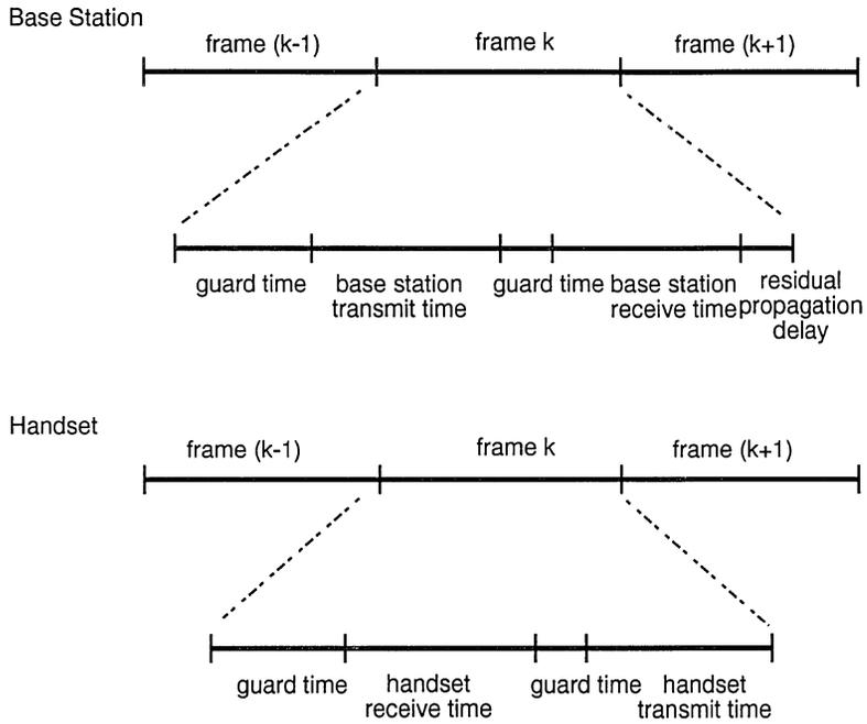
Figure 1. TDD Frame Structure
