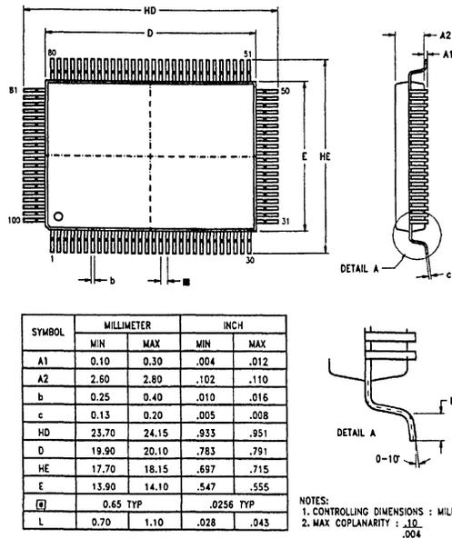
Figure 6. 100-Pin PQFP Package Diagram
