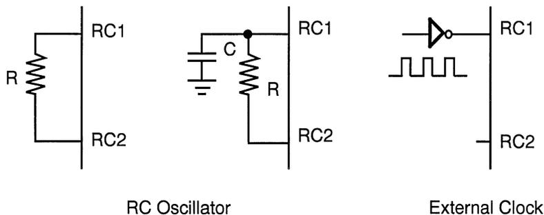
Figure 16. RC Oscillator Configuration
