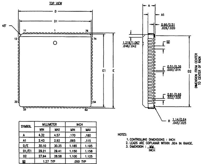
Figure 5. 84-Pin PLCC Package Diagram
