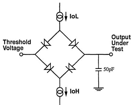
Figure 4. Test Load Diagram
