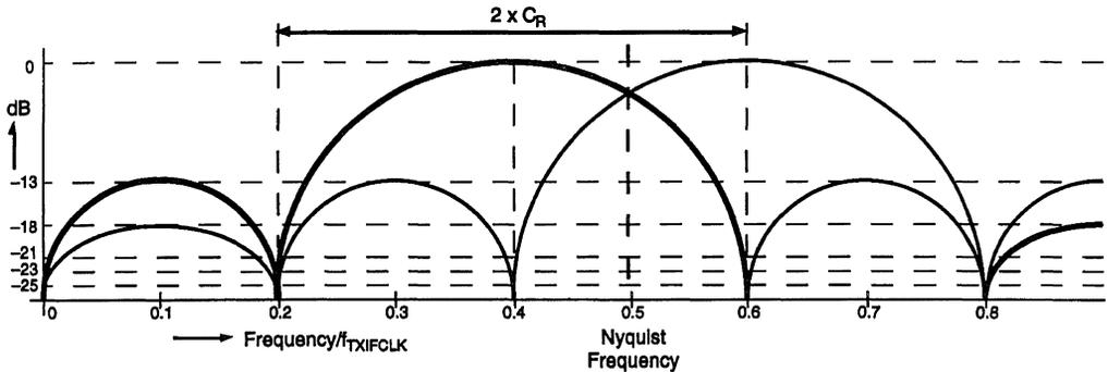
**Figure 18. Spectrum of DDS Modulated at  $0.4 \times f_{RXIFCLK}$
