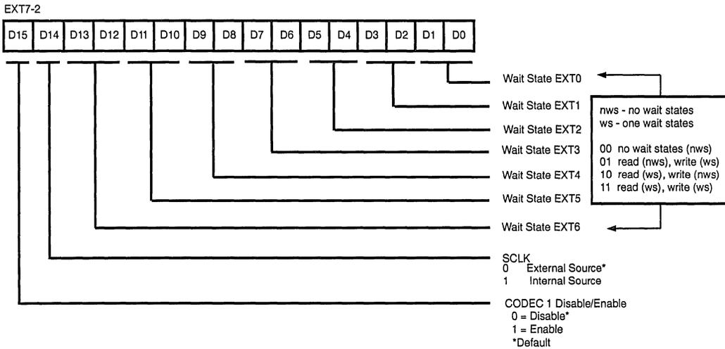
Figure 14. Wait/State/CODEC Interface Control Register
