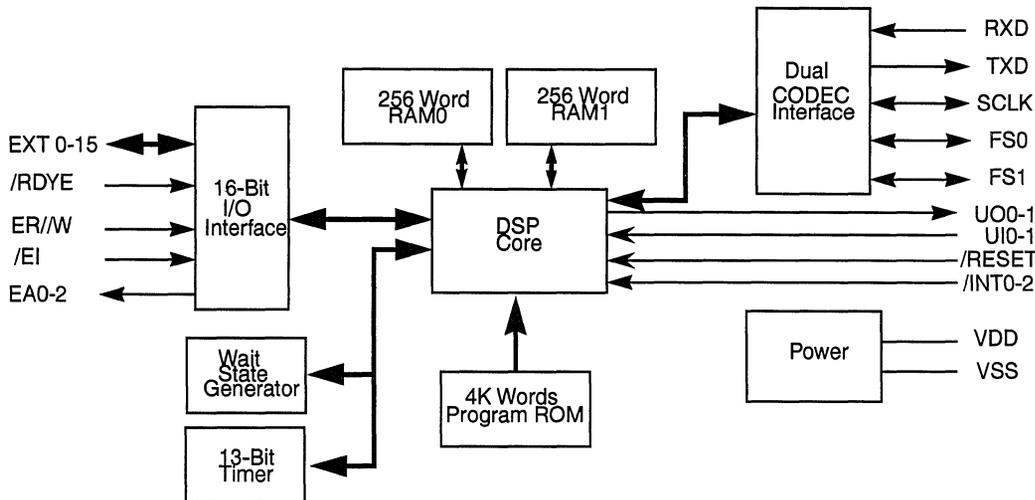
**Figure 1. Z87010 Functional Block Diagram**
