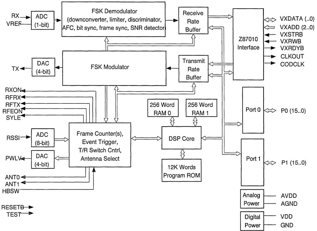
Figure 5. Z87000 Functional Block Diagram
