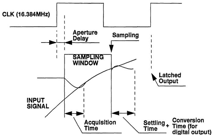
Figure 6. 1-Bit ADC Definition of Terms
