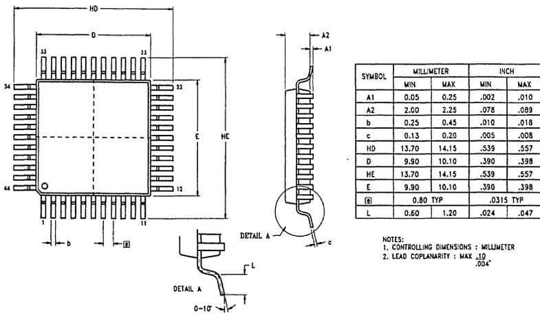
Figure 4. 44-Pin QFP Package Diagram
