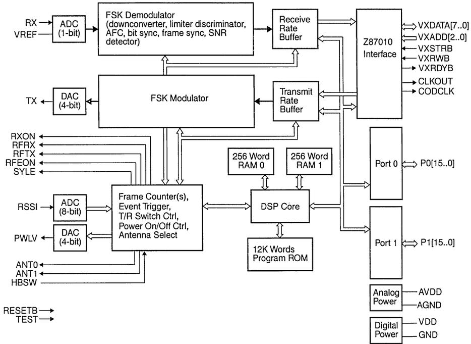
Figure 2. Z87000 Functional Block Diagram
