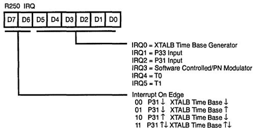
Figure 46. Interrupt Request Register (FAH: Read/Write)
