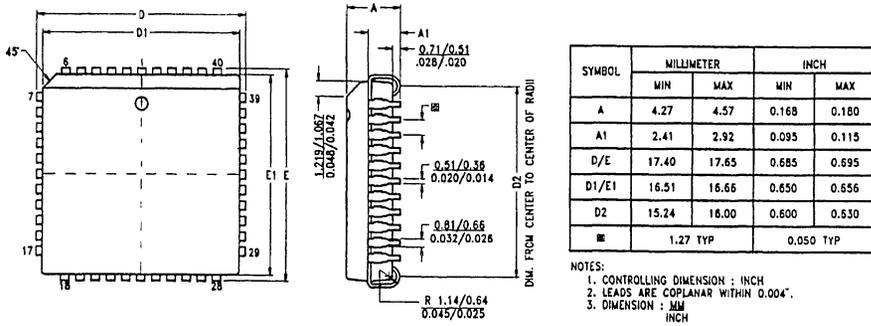
Figure 3. 44-Pin Lead PLCC Package Diagram
