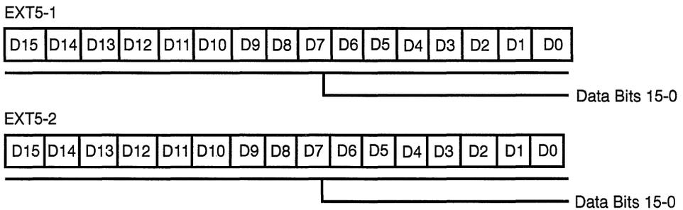
**Figure 11. CODEC Interface Data Registers (Channel 0)**
