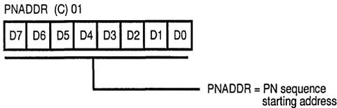
Figure 36. PN ROM Relative Address Register ((C) 01H: Read/Write)
