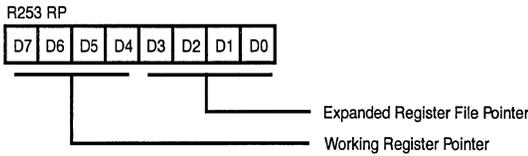
Figure 12. Register Pointer
