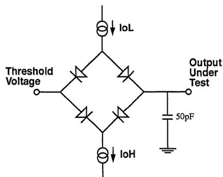
Figure 5. Test Load Diagram
