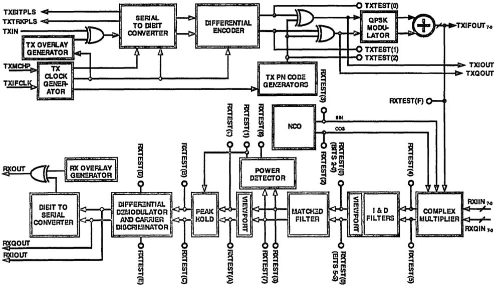
Figure 10. Transmitter and Receiver Test Points
