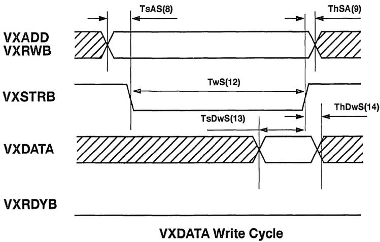
Figure 8. Read/Write Cycle Timings
