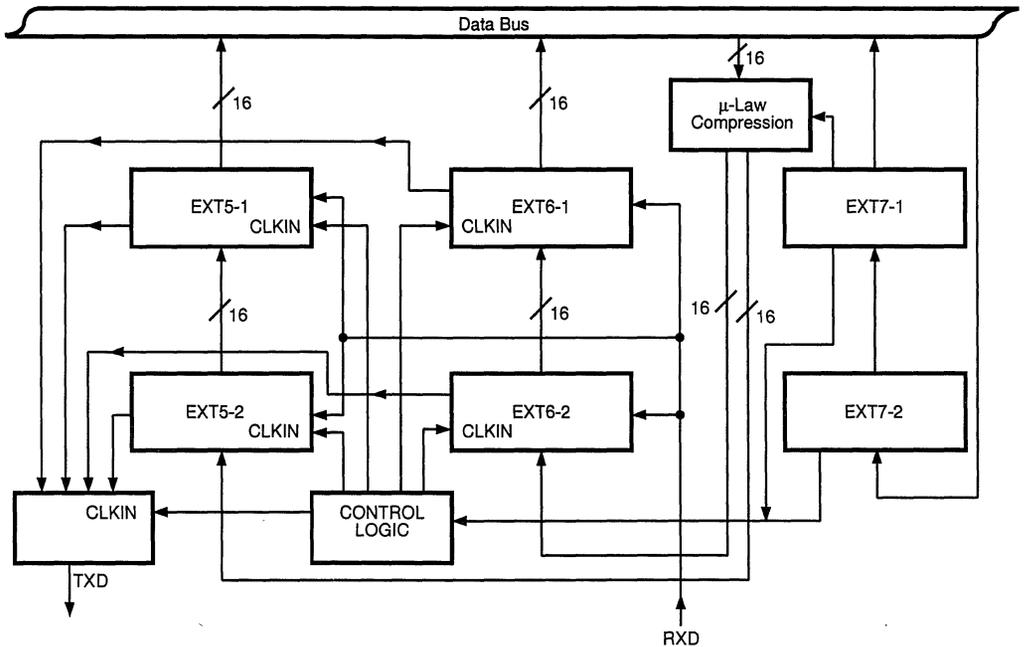
Figure 9. CODEC Interface Block Diagram
