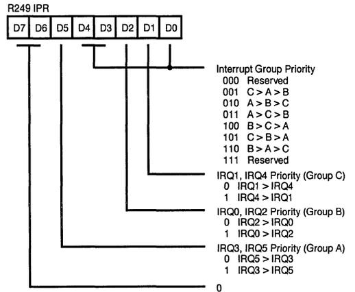
Figure 45. Interrupt Priority Register (F9H: Write Only)
