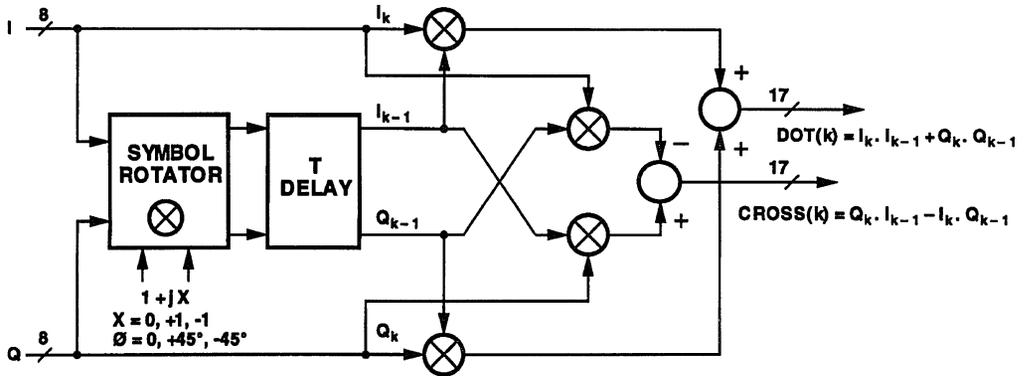
**Figure 8. DPSK Demodulator I and Q Channel Processing**
