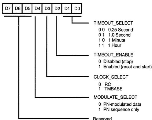
**Figure 20. Time Base Generator Control Register**
