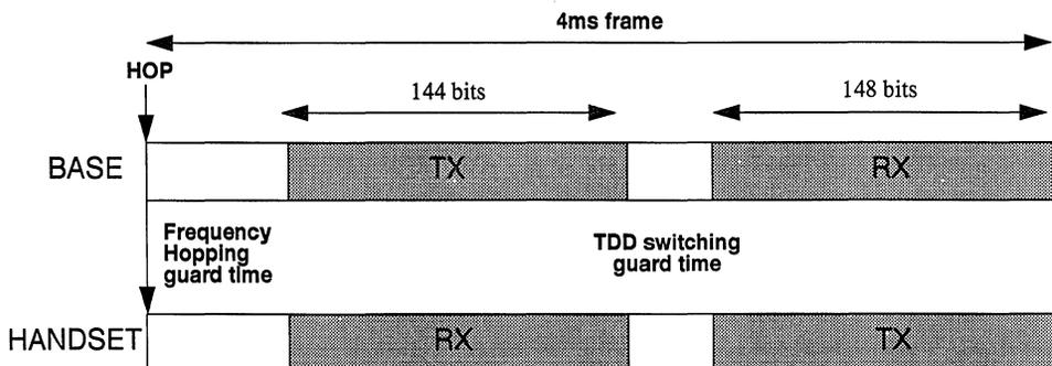
Figure 1. Basic Time Duplex Timing
