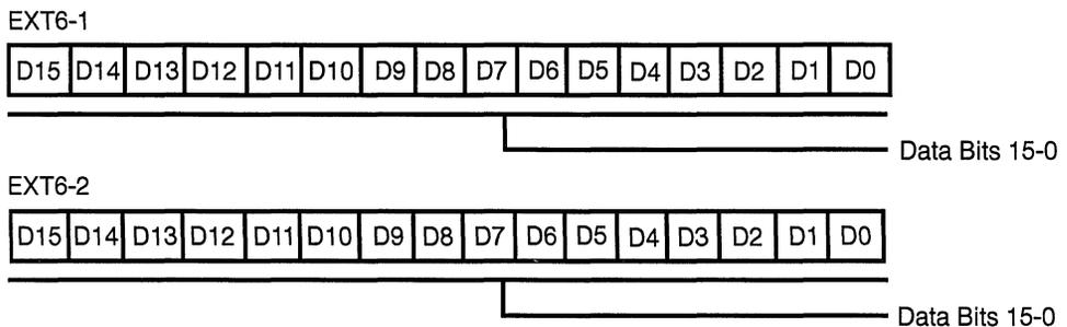
**Figure 12. CODEC Interface Data Registers (Channel 1)**
