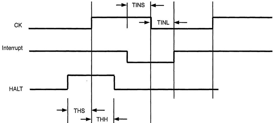
Figure 7. Interrupt/HALT Timing
