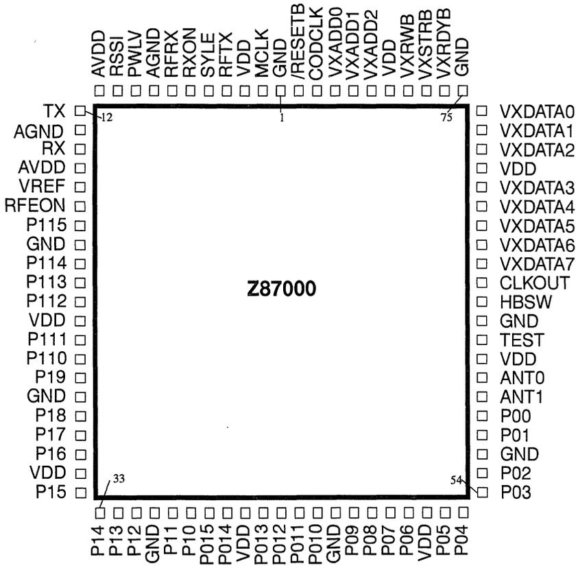
Figure 3. 84-Pin PLCC ROM Pin Configuration (Z87000 only)
