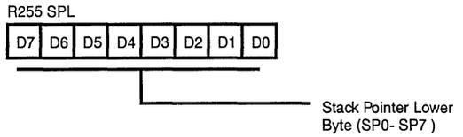
Figure 51. Stack Pointer
