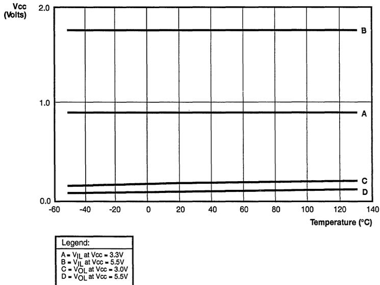
Figure 53. Typical  $V_{OL}$ ,  $V_{IL}$  vs Temperature
