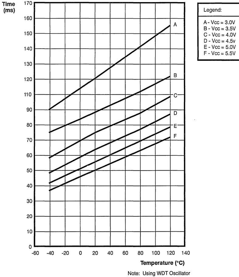
Figure 60. Typical 25 ms WDT Setting vs Temperature
