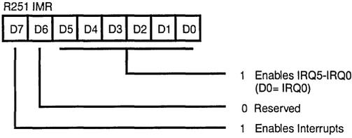
Figure 47. Interrupt Mask Register
