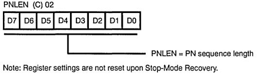
Figure 37. PN Code Length Register ((C) 02H: Read/Write)
