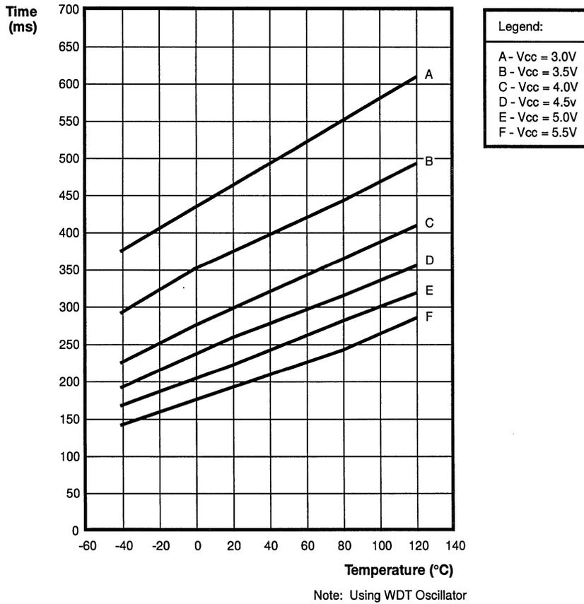
Figure 61. Typical 100 ms WDT Setting vs Temperature
