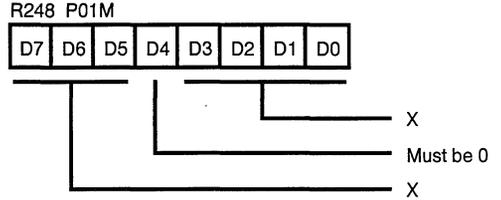
Figure 44. Port 0 and 1 Mode Register (F8H: Write Only)
