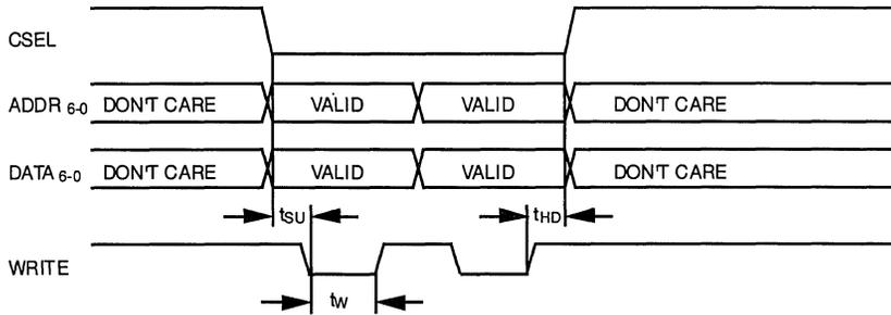
**Figure 3. Microprocessor Interface Timing**
