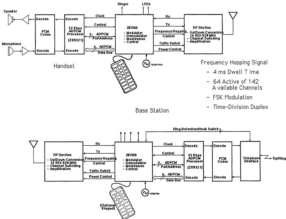
Figure 4. Z87000 Cordless Phone Transceiver/Controller
