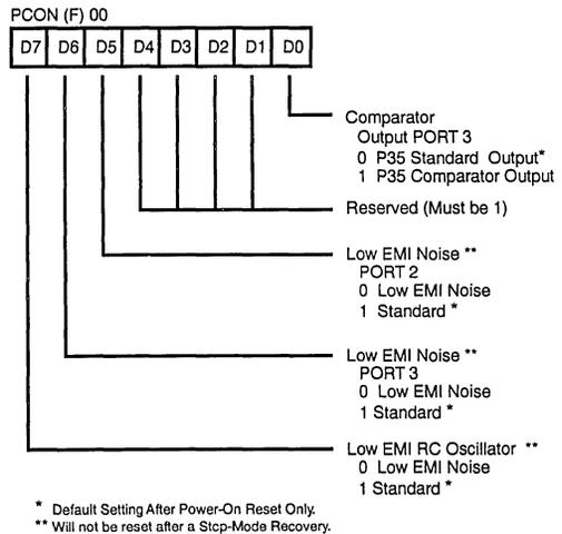
**Figure 9. PORT Configuration Register (PCON)**
