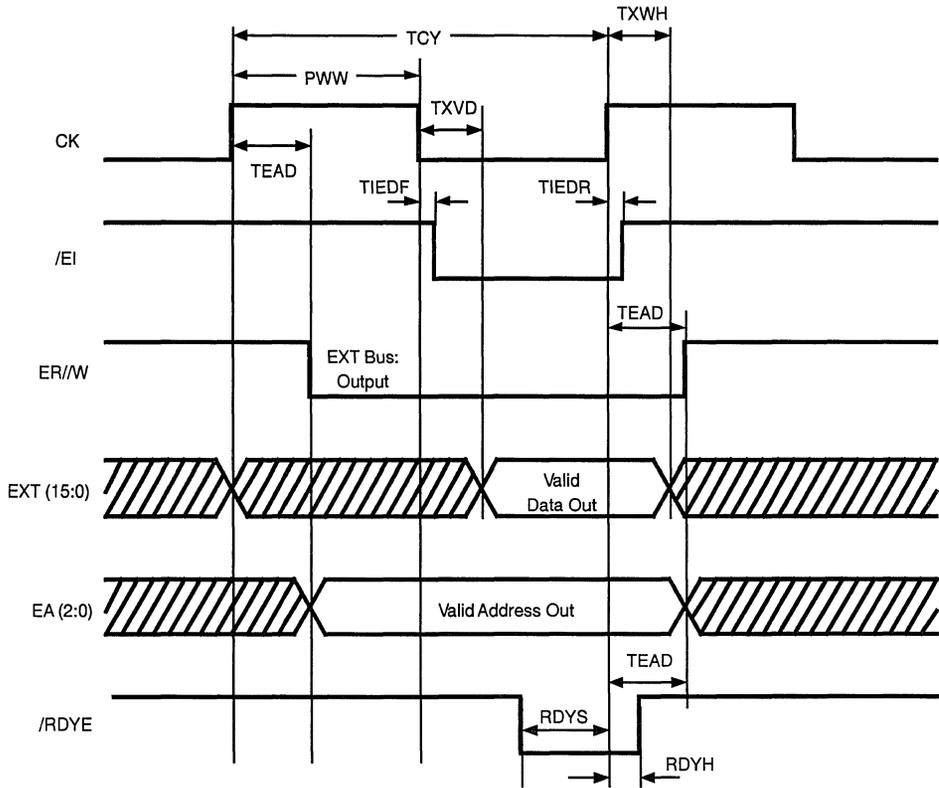
Figure 5. Write to External Device Timing
