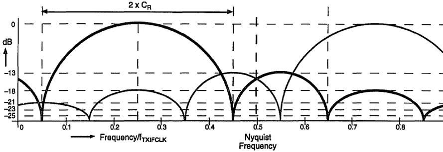
Figure 19. Spectrum of DDS Modulated at  $0.4 \times f_{RXIFCLK}$
