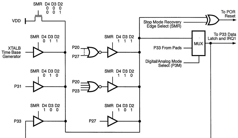
**Figure 22. Stop-Mode Recovery Source**
