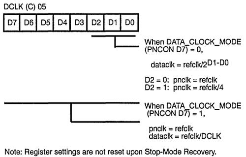
Figure 40. Data Clock Control Register ((C) 05H: Read/Write)
