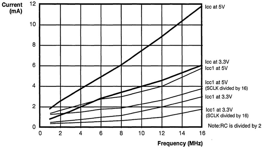
Figure 52. Typical  $I_{CC}$  vs Frequency
