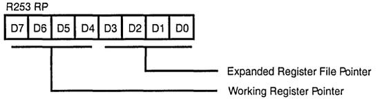
Figure 49. Register Pointer
