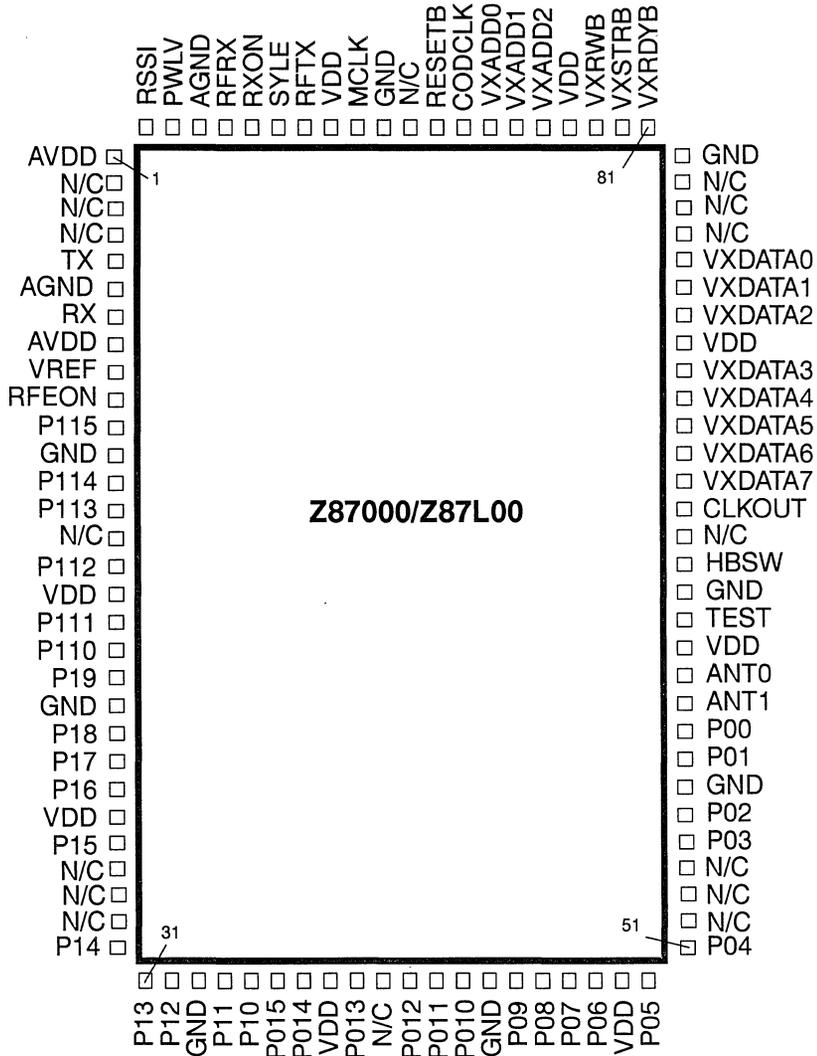
Figure 4. 100-Pin QFP Pin Configuration
