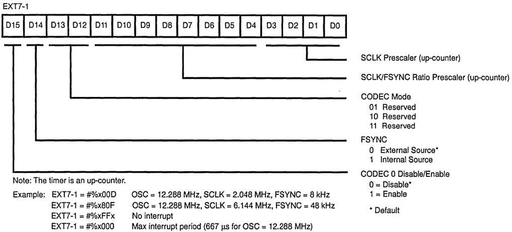
Figure 13. CODEC Interface Control Register
