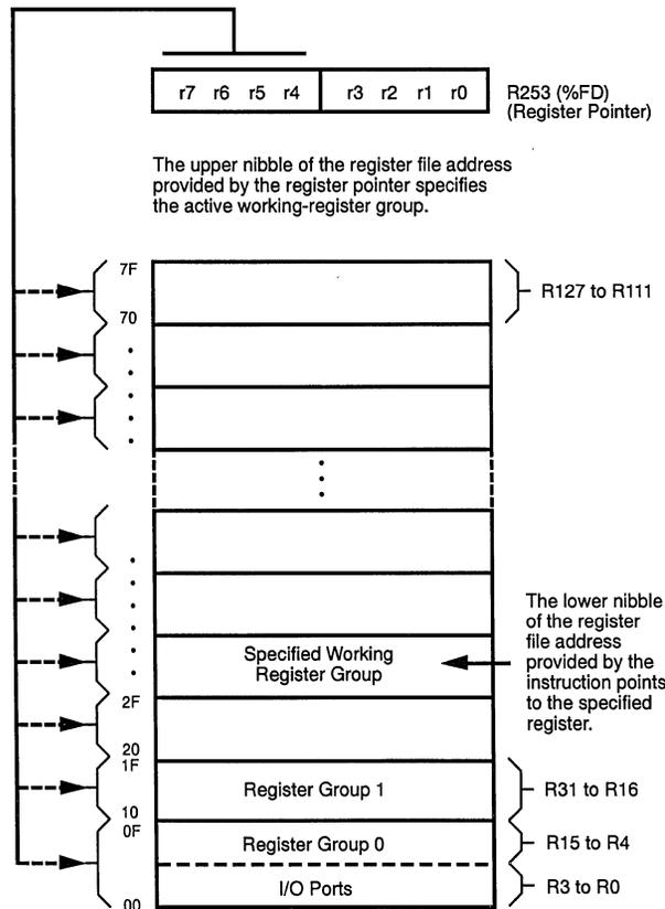
Figure 13. Register Pointer
