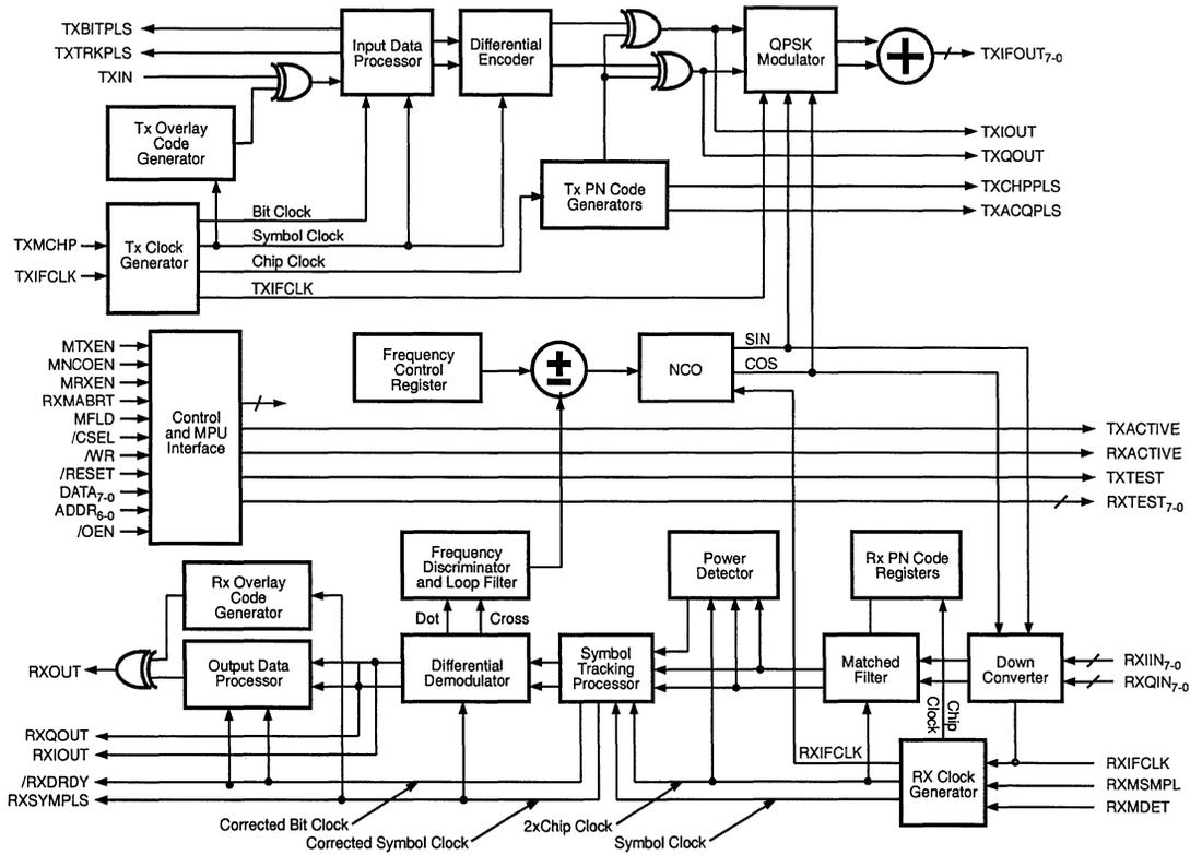
Figure 1. Z87200 Block Diagram
