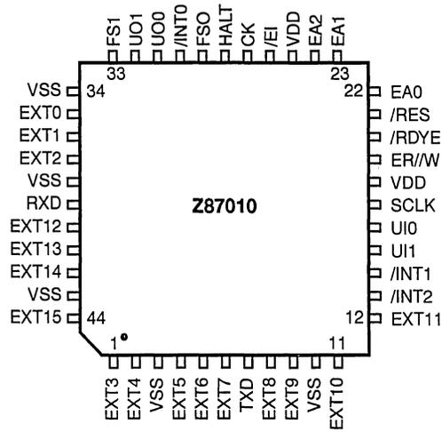
Figure 3. 44-Pin QFP Pin Assignments
