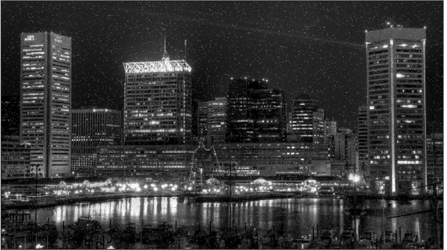
Figure 1 – Input image affected by impulsive noise. Only 2 percent of the pixels are corrupted, but that’s enough to severely degrade the image quality.
