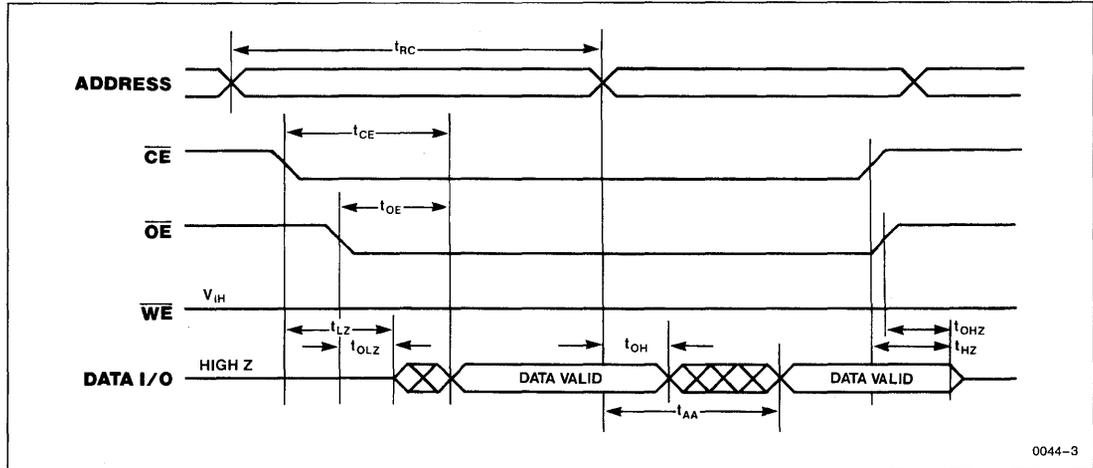
Note: (2)  $t_{HZ}$  and  $t_{OHZ}$  are measured from the point when  $\overline{CE}$  or  $\overline{OE}$  return high (whichever occurs first) to the time when the outputs are no longer driven.
