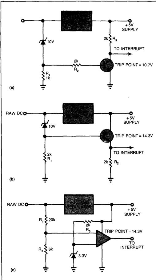
**Fig 7**—Using zener diodes you can configure a power-supply detector circuit to produce either a negative (a) or a positive (b) interrupt pulse when the trigger point is reached. You can configure the op amp shown in c to produce either a positive or a negative output pulse polarity.
