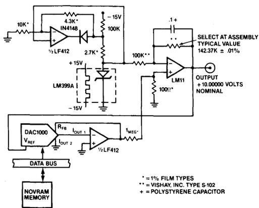
Figure 12) Software programmable voltage reference.
