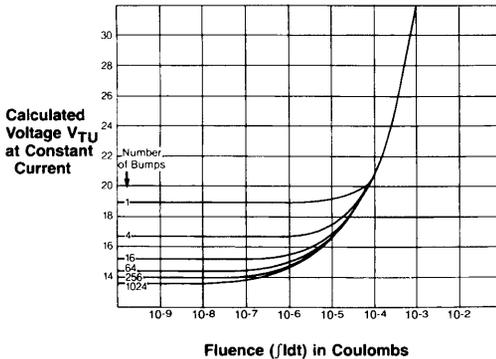
Figure 3: Effect of Number of Samples  $k$  on Calculated Tunnel Voltage
