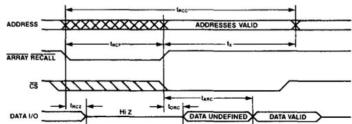
Figure 7) Timing diagram for the RECALL operation.
