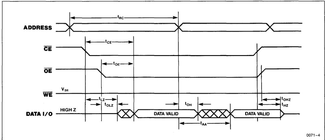
Note: (3)  $t_{HZ}$  and  $t_{OHZ}$  are measured from the point when  $\overline{CE}$  or  $\overline{OE}$  return high (whichever occurs first) to the time when the outputs are no longer driven.
