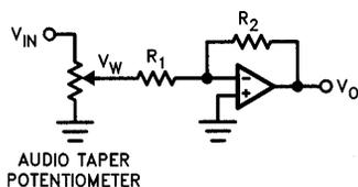
Figure 1: Conventional Potentiometer Volume Control
