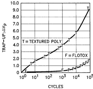
Figure 2: Trap-up vs. cycles for Textured Poly (2864) and FLOTOX (2816A). Trap-up is measured in terms of the increase in programming voltage  $\Delta V_p$  necessary to program the cell. 0024-2
