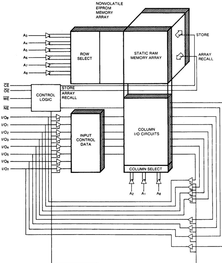
Figure 2: X2004 functional block diagram.
