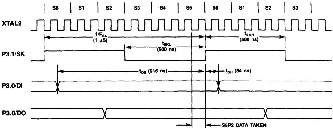
Figure 1. 12 MHz 8051 Serial Port Mode 0 and X2444 Timing
