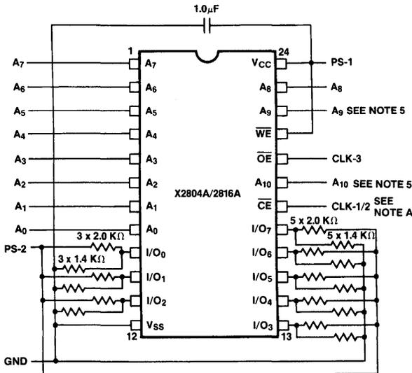
Figure 8a: X2804A/2816A (DIP) Burn-In Circuit
