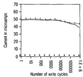
Figure 5: E<sup>2</sup>PROM cell test endurance data.
