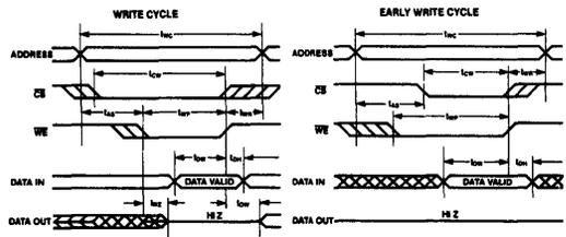
Figure 4) Timing diagram for Writing to the RAM.
