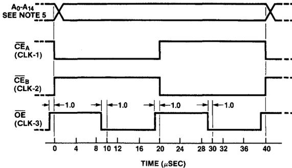
Figure 9b: X2864A/2864B/2864H/28256 (DIP) Burn-In Timing
