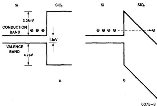
Figure 7: Energy band diagrams of the Si/SiO<sub>2</sub> system in the neutral state (a), and during the store operation (b).
