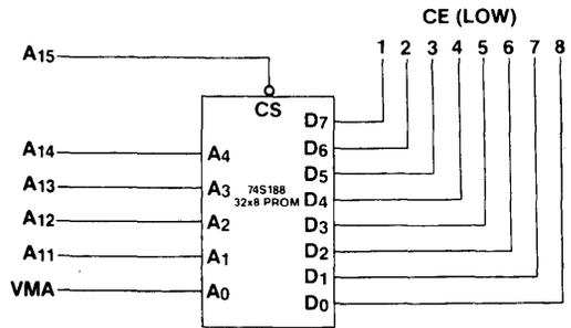
Figure 5. Bipolar PROM Mapping
