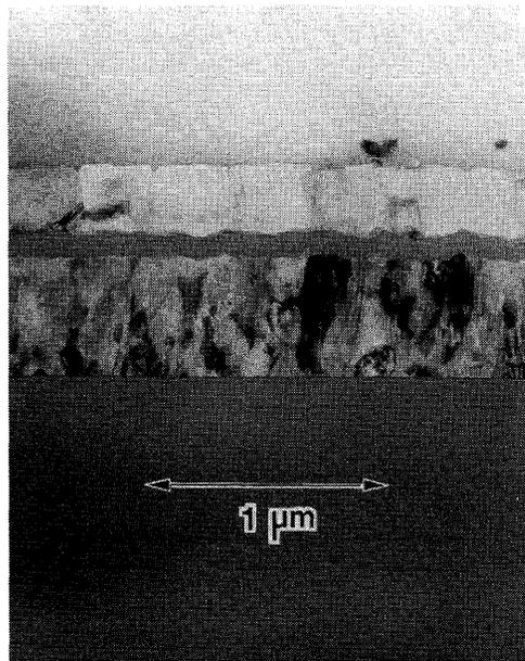
Figure 10: Transmission electron microscope (TEM) photograph of a cross-section through a textured tunneling structure. The one micron-long arrow shows the scale.
