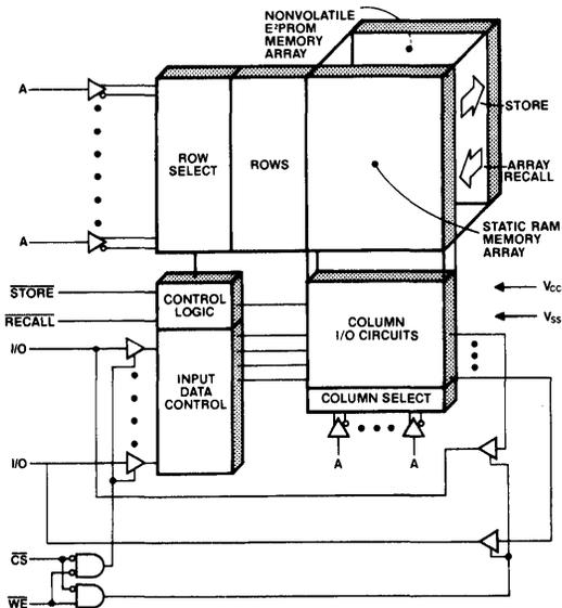
Figure 1) NOVRAM memory block diagram.
