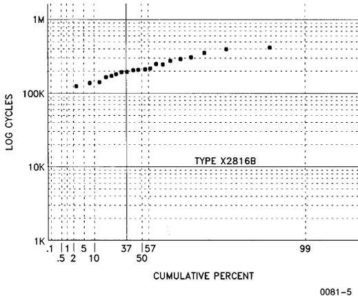
Figure 5: An extreme value distribution of endurance monitor on units cycled in mass mode.
