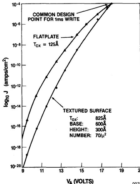
Figure 14: Comparison of calculated tunneling J-V curves for emission from a planar and a textured structure. The devices were designed to have the same emission in the high current regime where programming takes place.
