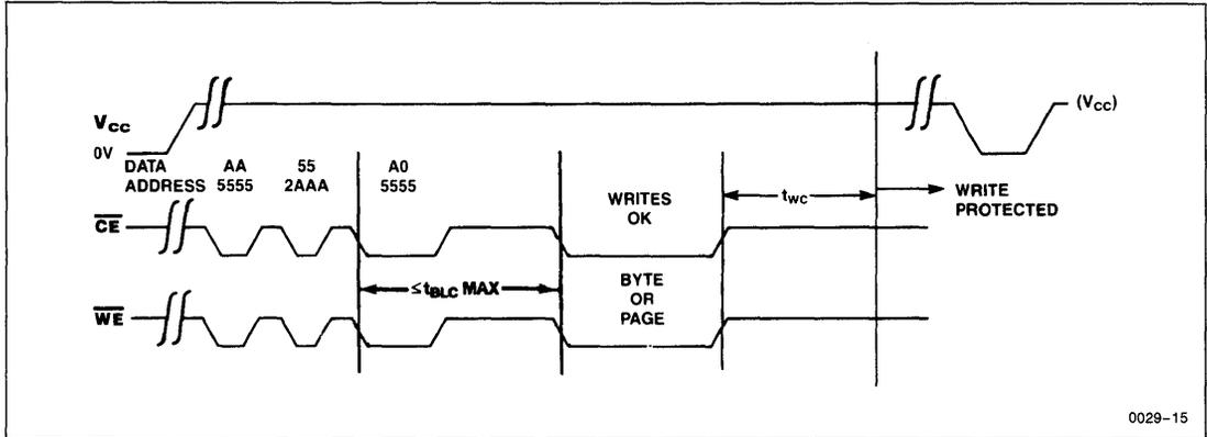
Figure 4b: Write Sequence for Software Data Protection
