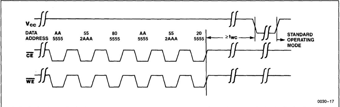
Figure 5b: Software Sequence to Deactivate Software Data Protection
