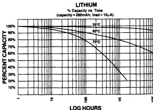
Figure 1: Lithium-Capacity vs. Time with Varying Temperatures
