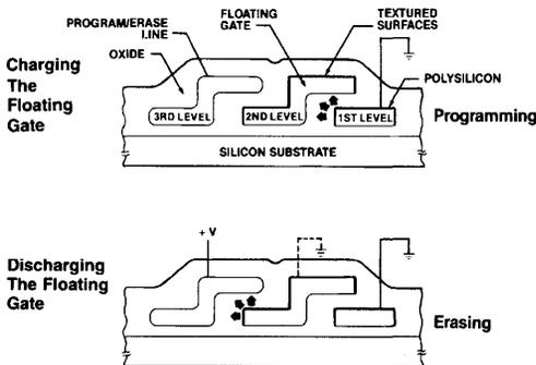
Figure 1: TPFG Cell Operation
