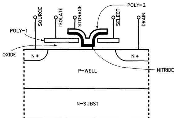
Figure 1c: Cross sectional structure of a MNOS memory cell.<sup>8</sup>
