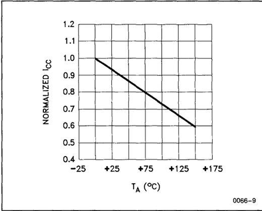
**Normalized Standby Supply Current vs. Ambient Temperature**
