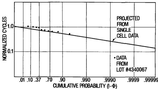
Figure 6: This is a Log Extreme Value probability plot of the endurance of a lot of X2212 NOVRAMs. The points are measured values, the straight line represents endurances predicted from the single cell data shown in Figure 5.
