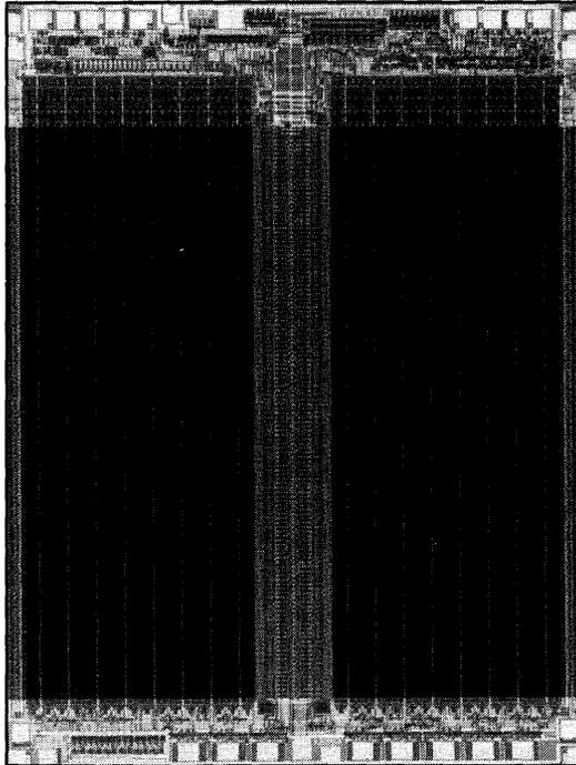
**1. SMALL DIE.** Equivalent in size to many thin-oxide 64-K parts, Xicor's 256-K EEPROM die measures about 64,000 mils<sup>2</sup>.
