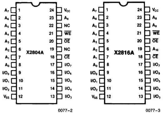
Figure 1: X2804A and X2816A Pin configurations.
