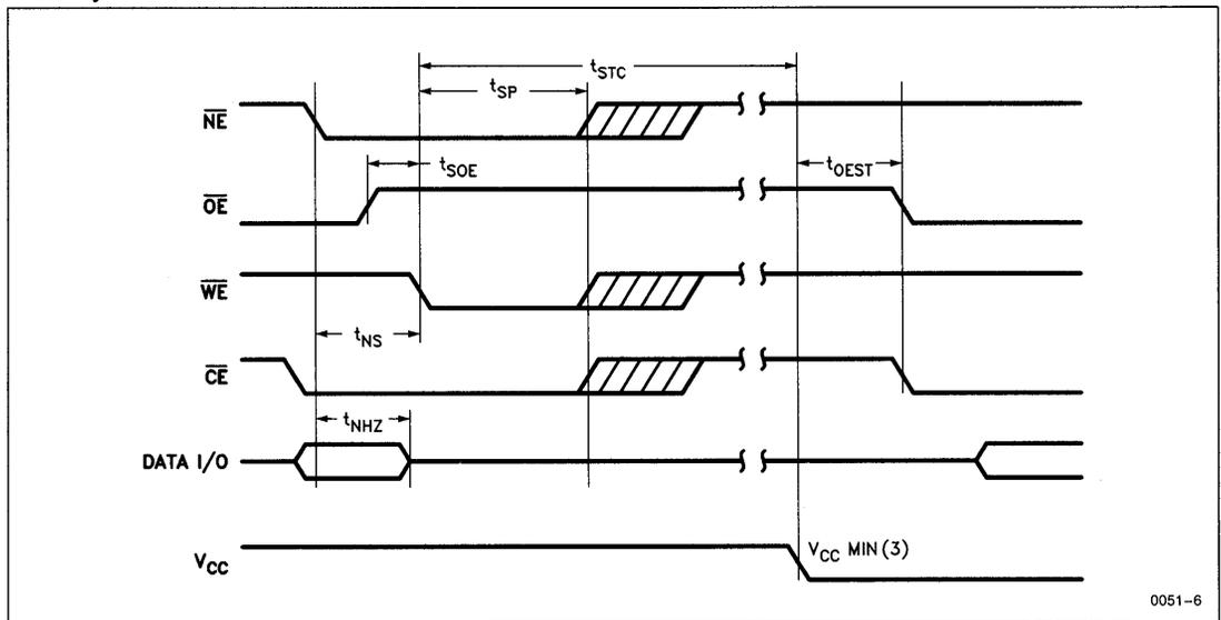
Note: (3) X2001  $V_{CC}$  Min. = 4.75V
