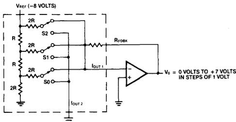
Figure 7) A simplified 3-switch CMOS DAC.
