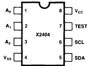
Figure 1: X2404 Pin configuration.
