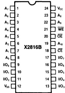
Figure 1: X2816B pin configuration.
