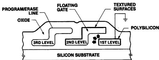
Figure 4: Cross sectional structure of a textured poly memory cell. 0079-2
