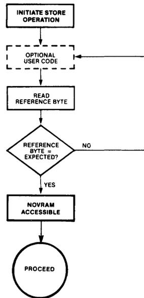
Figure 2: Early Write Completion Flowchart
