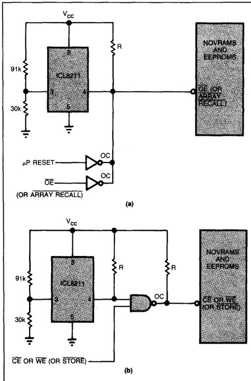
**Fig 10**—In a hold-low protection scheme (a), a nonvolatile memory's array-recall pin is pulled to logical zero when the supply voltage falls below 5V. In hold-high protection (b), when power is lost, either the WE or CE pins are held high.
