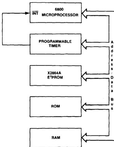
Figure 1: Hardware Configuration of a Typical System with the E<sup>2</sup>PROM and the Programmable Timer on the Bus
