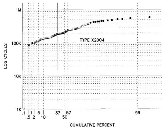
Figure 8: Extreme value distribution plot for X2004.
