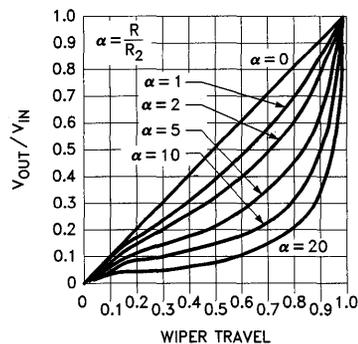
Figure 9: Utilizing External Resistors to Vary Potentiometers Trim (EDN Nov. 13)
