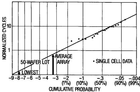
Figure 5: This shows the Log Normal probability plot of individual single cell endurance data. The right half of the plot is quite standard, as marked by typical cumulative percentages. The left half represents an extension of the standard chart to much lower probabilities, in order to permit predictions for specific members of a much larger population.
