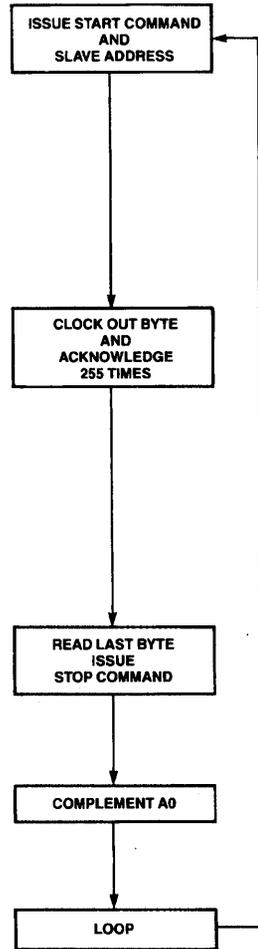
X2404 Burn-in timing diagram and program flow.
