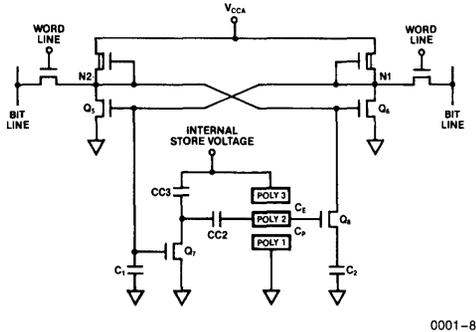
Figure 2) Circuit diagram of a NOVRAM cell.
