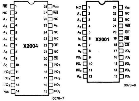
Figure 1: X2004 and X2001 pin configurations.
