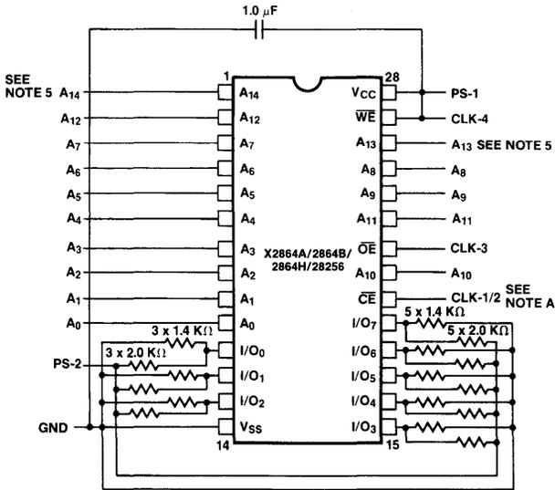
Figure 9a: X2864A/2864B/2864H/28256 (DIP) Burn-In Circuit
