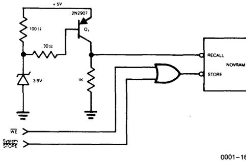
Figure 11) Another form of power supply status detector to drive the RECALL pin LOW when the supply drops below 4.5Volts.
