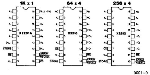
Figure 3) Pin configuration of the XICOR NOVRAM family.
