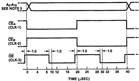
Figure 8b: X2804A/2816A (DIP) Burn-In Timing
