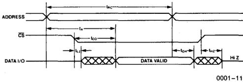
Figure 5) Timing diagram for Reading from the RAM.
