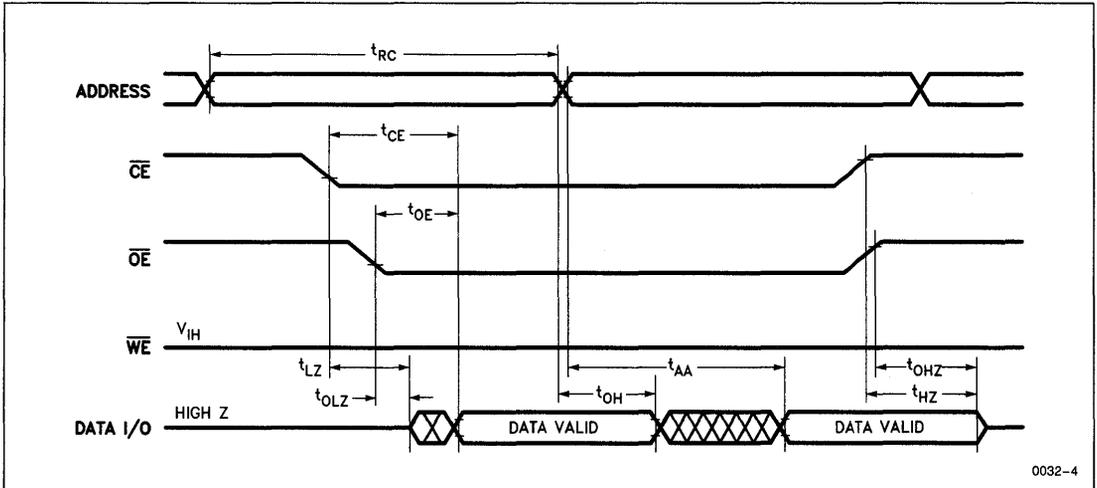
**Note:** (3)  $t_{HZ}$  and  $t_{OHZ}$  are measured from the point when  $\overline{CE}$  or  $\overline{OE}$  return high (whichever occurs first) to the time when the outputs are no longer driven.
