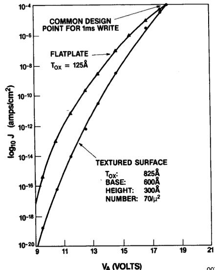
Figure 5: Comparison of calculated tunneling J-V curves for emission from a planar and a textured structure. The devices were designed to have the same emission in the high current regime where programming takes place. 0079-3
