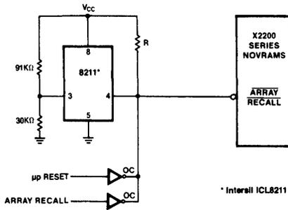
Figure 3: Power-up/Power-down Write Protection Circuit
