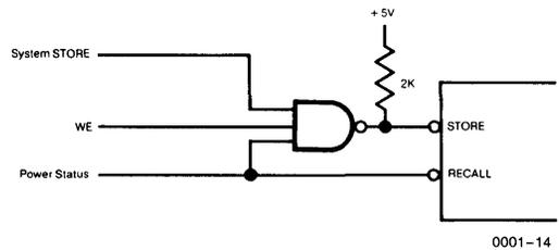
Figure 9) A power supply status line held LOW can insure that both the RECALL pin is held LOW and the STORE pin is held HIGH.
