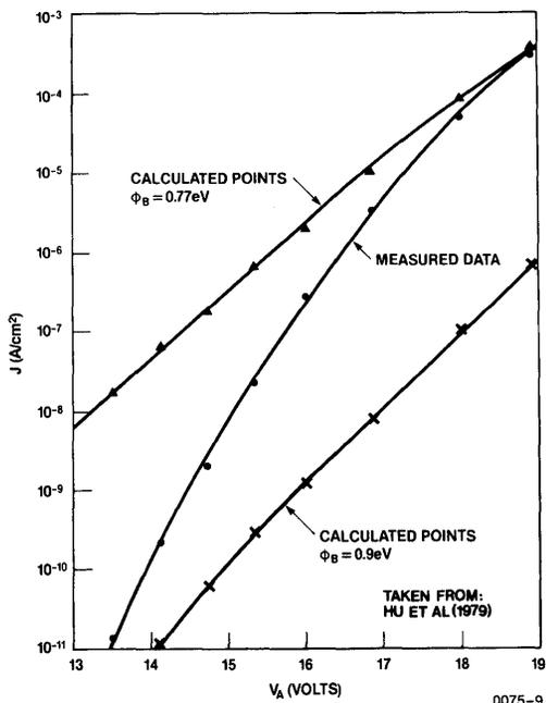
Figure 8: Current vs. applied voltage for current from textured poly surface emitted through 1760Å of thermal SiO<sub>2</sub> compared with calculations based on previously available theory.
