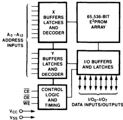
Figure 2: X2864A Functional block diagram.
