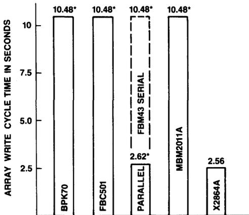
Figure 2: Array Write Cycle Times
