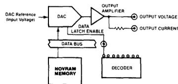
Figure 9) A NOVRAM memory DAC combination provides a voltage or a current to correct analog circuits.
