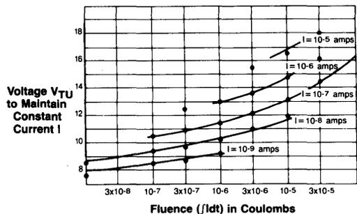
Figure 2: Tunnel Voltage vs. Fluence at Constant Current. Lines are experimental data, solid circles are calculated from eq (8).
