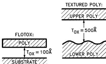
Figure 3: FLOTOX and Textured Poly structures. 0024-3
