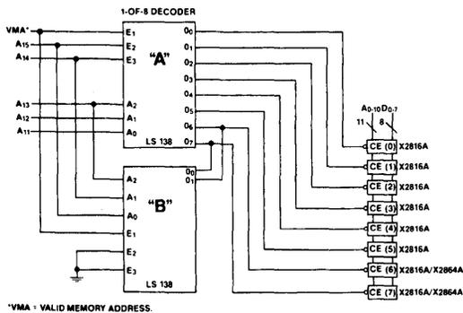
Figure 4. 74LS138 Decode Wiring Option
