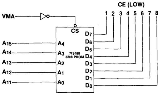
Figure 6. Bipolar PROM Mapping for Memory Expansion
