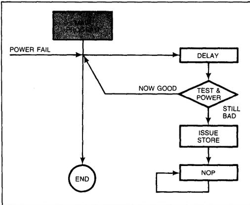
**Fig 3**—In a typical  $\mu P$  system that tests for power loss, once the processor receives an interrupt indicating a power loss, the system initiates a subroutine that tests for a true power loss. The subroutine first produces a delay of about 2 msec; then the system looks again at the power detector's output. If that output is still asserted, the system decides that the power loss is real and sends a store pulse to the nonvolatile RAM.
