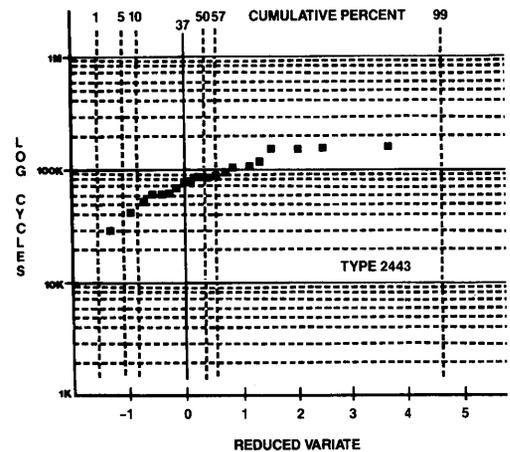
Figure 7: Endurance data from a lot of Xicor X2443 Serial NOVRAMs. 0076-7
