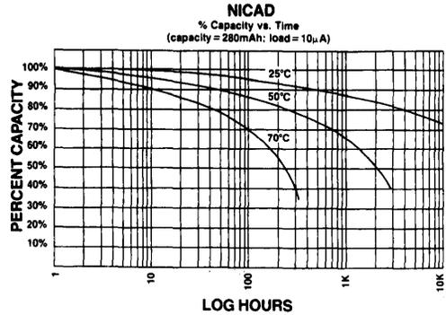
Figure 2: Nicaid-Capacity vs. Time with Varying Temperatures
