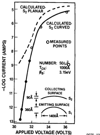
Figure 13: Reverse tunneling characteristic comparing the measured data with curves calculated for a concave and planar emitting surface.
