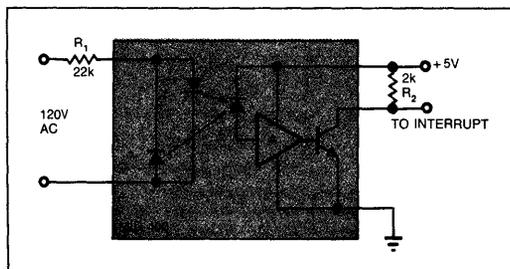
**Fig 5**—To incorporate the MID 400 detector in your sensing subsystem, you need to add only two external resistors that you connect directly to the ac line. You can control the on and off delays at the output by connecting a capacitor across  $R_2$ .
