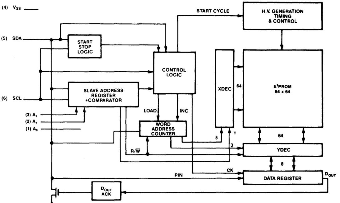
Figure 2: X2404 Functional block diagram.
