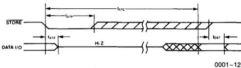
Figure 6) Timing diagram for the STORE operation where data is transferred from the RAM to the EEPROM.
