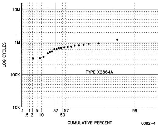
Figure 3: Mass mode cycling data for X2864A.
