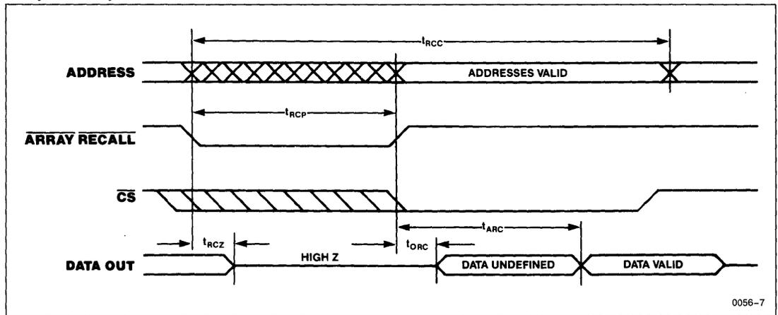
**Note:** (4) Array Recall rise time must be less than 1  $\mu$ s.
