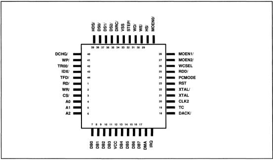
FIGURE 5. WD57C65 44-PIN PLCC
