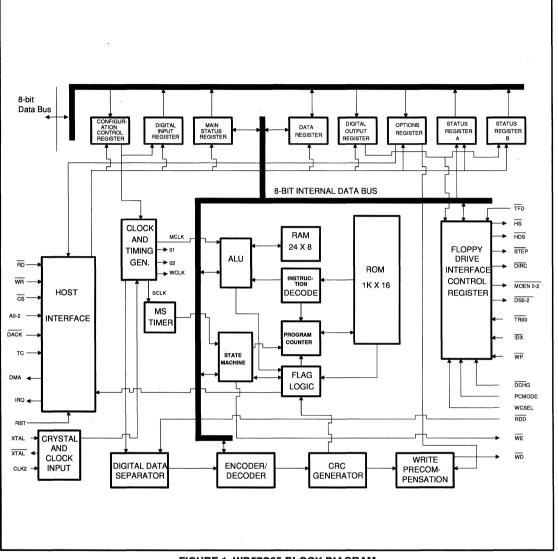
FIGURE 1. WD57C65 BLOCK DIAGRAM
