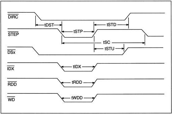
FIGURE 12. DISK DRIVE TIMING
