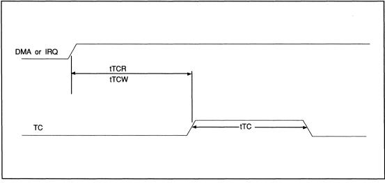
FIGURE 10. TERMINAL COUNT TIMING
