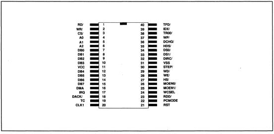
FIGURE 4. WD57C65 40-PIN DIP
