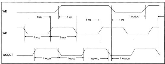
FIGURE 25. WRITE DATA TIMING (NRZ MODE)
