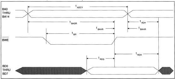
FIGURE 17. BUFFER READ TIMING (INTERNAL OSCILLATOR)
