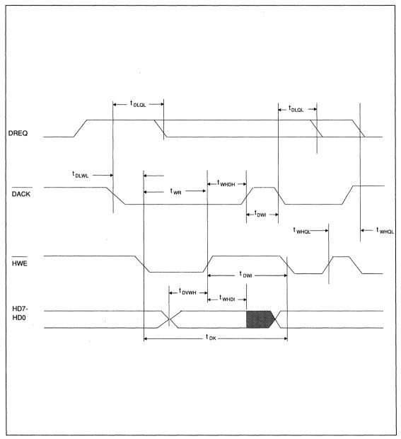
FIGURE 10. AT/XT HOST DMA WRITE TIMING
