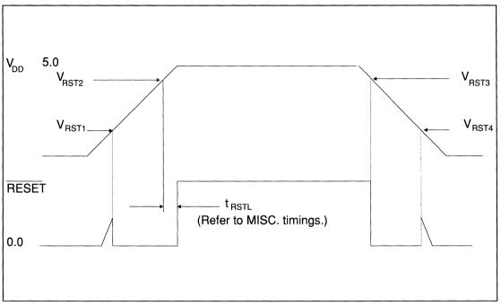
FIGURE 6. POWER QUALIFIED RESET VOLTAGE THRESHOLD
