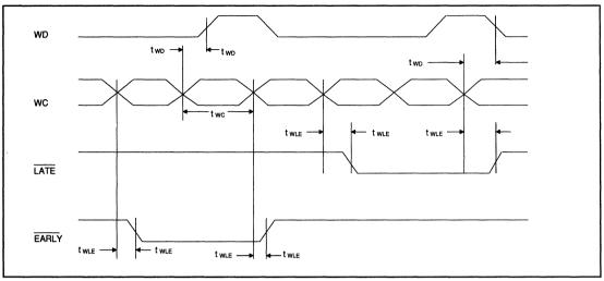
FIGURE 24. WRITE DATA TIMING (MFM/RLL MODE)
