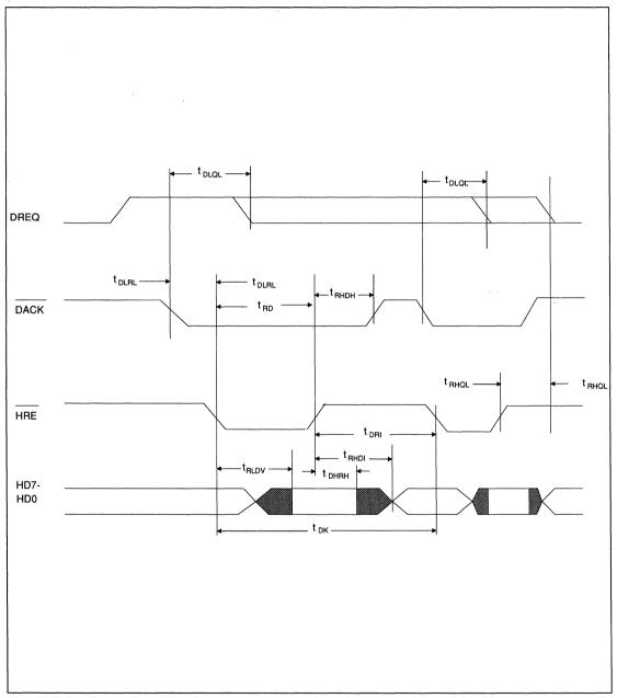
FIGURE 11. AT/XT HOST DMA READ TIMING
