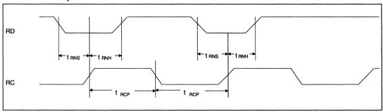
FIGURE 27. READ DATA TIMING (NRZ MODE)
