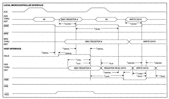
FIGURE 12. SLAVE HOST WRITE TIMING
