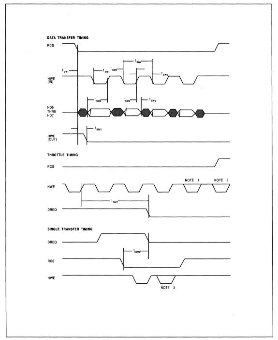
FIGURE 14. SLAVE HOST DMA WRITE TIMING
