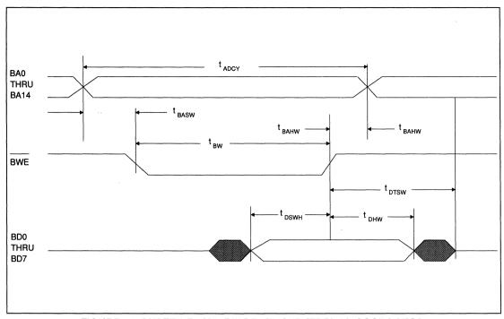
FIGURE 18. BUFFER RAM WRITE TIMING (EXTERNAL OSCILLATOR)
