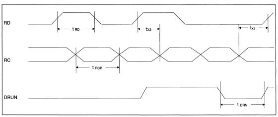
FIGURE 26. READ DATA TIMING (MFM/RLL)
