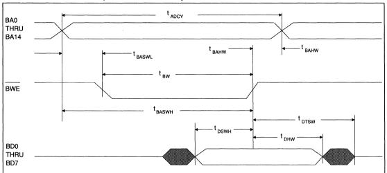
FIGURE 16. BUFFER RAM WRITE TIMING (INTERNAL OSCILLATOR)
