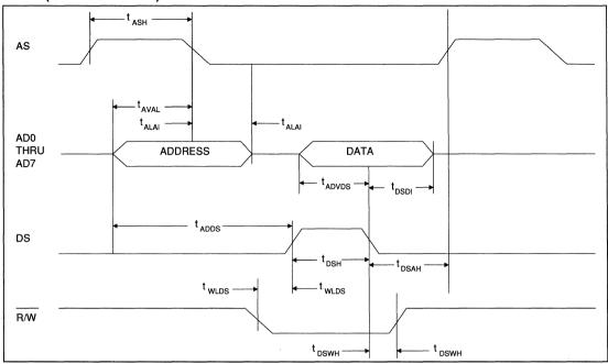
FIGURE 21. MICROPROCESSOR WRITE TIMING (MOTOROLA BUS)
