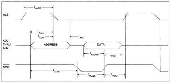
FIGURE 20. MICROPROCESSOR WRITE TIMING (INTEL BUS)
