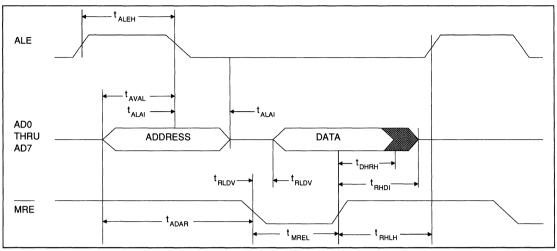
FIGURE 22. MICROPROCESSOR READ TIMING (INTEL BUS)
