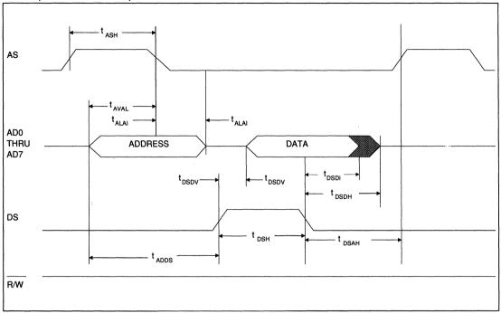
FIGURE 23. MICROPROCESSOR READ TIMING (MOTOROLA BUS)
