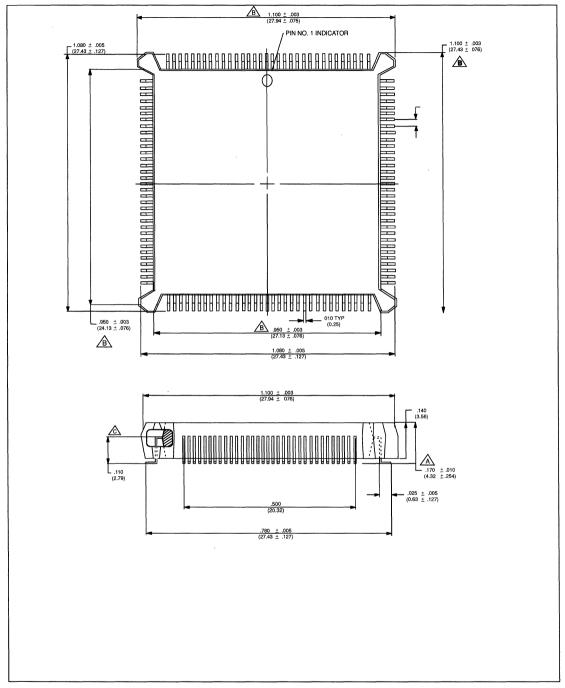
FIGURE 36. 84-LEAD PQFP
