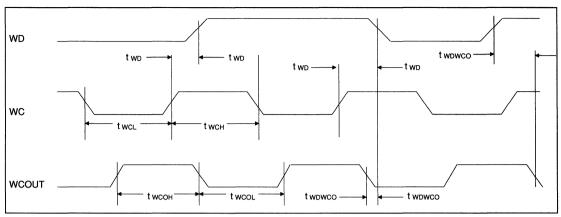
FIGURE 24. WRITE DATA TIMING (NRZ MODE)
