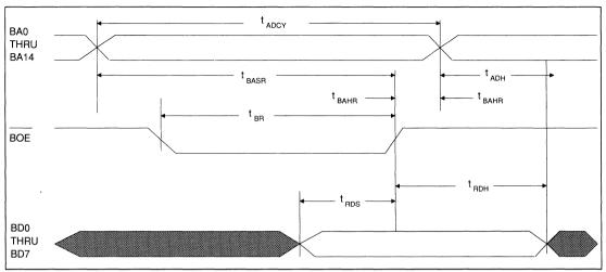
FIGURE 18. BUFFER RAM READ TIMING (EXTERNAL OSCILLATOR)
