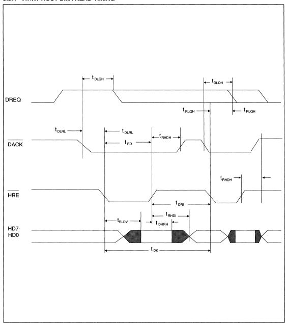
FIGURE 12. AT/XT HOST DMA READ TIMING
