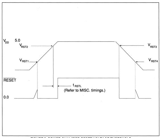
FIGURE 7. POWER QUALIFIED RESET VOLTAGE THRESHOLD
