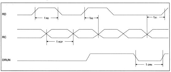
FIGURE 25. READ DATA TIMING (MFM/RLL)
