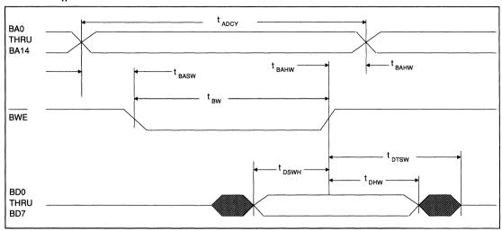
FIGURE 15. BUFFER RAM WRITE TIMING (INTERNAL OSCILLATOR)
