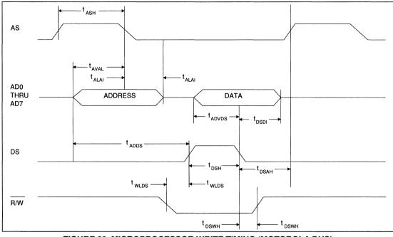
FIGURE 20. MICROPROCESSOR WRITE TIMING (MOTOROLA BUS)
