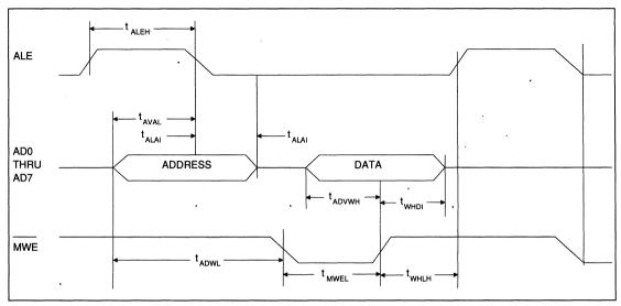
FIGURE 19. MICROPROCESSOR WRITE TIMING (INTEL BUS)
