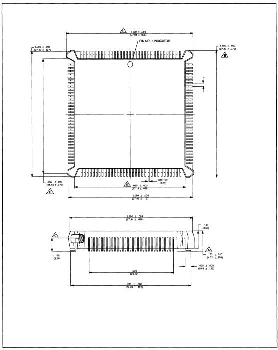
FIGURE 35. 84-LEAD PQFP
