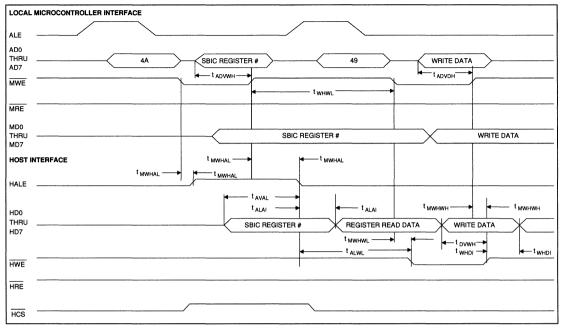
FIGURE 13. SLAVE HOST WRITE TIMING
