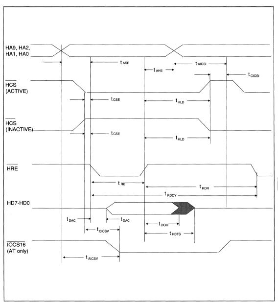
FIGURE 10. AT/XT HOST PROGRAMMED I/O READ TIMING
