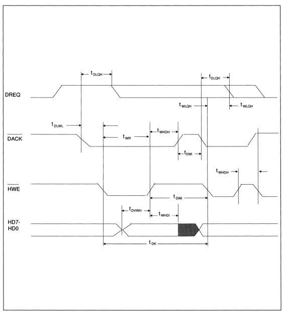
FIGURE 11. AT/XT HOST DMA WRITE TIMING
