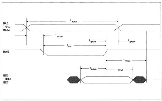
FIGURE 17. BUFFER RAM WRITE TIMING (EXTERNAL OSCILLATOR)
