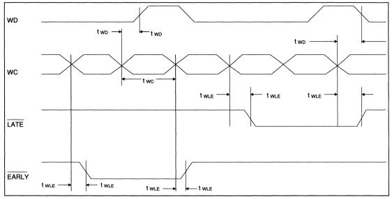
FIGURE 23. WRITE DATA TIMING (MFM/RLL MODE)
