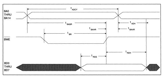
FIGURE 16. BUFFER RAM READ TIMING (INTERNAL OSCILLATOR)
