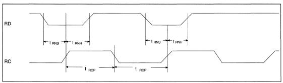
FIGURE 26. READ DATA TIMING (NRZ MODE)
