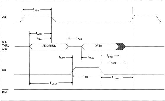
FIGURE 22. MICROPROCESSOR READ TIMING (MOTOROLA BUS)
