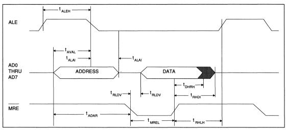
FIGURE 21. MICROPROCESSOR READ TIMING (INTEL BUS)
