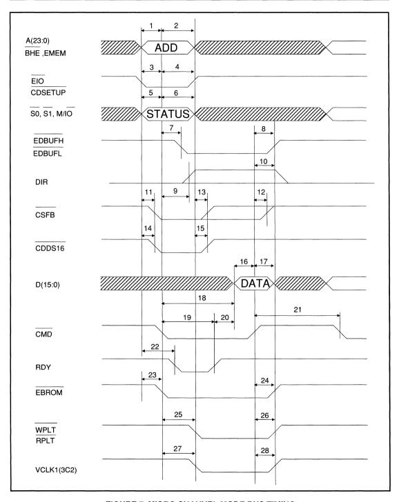
FIGURE 7. MICRO CHANNEL MODE BUS TIMING
