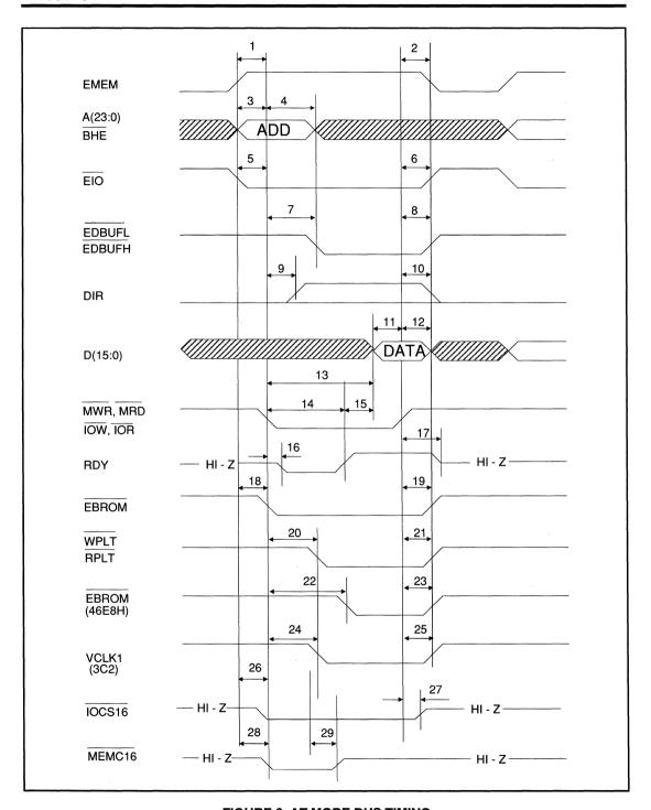
FIGURE 6. AT MODE BUS TIMING
