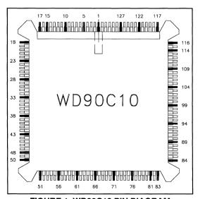
FIGURE 1. WD90C10 PIN DIAGRAM
