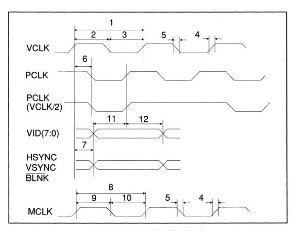
FIGURE 5. CLOCK AND VIDEO TIMING
