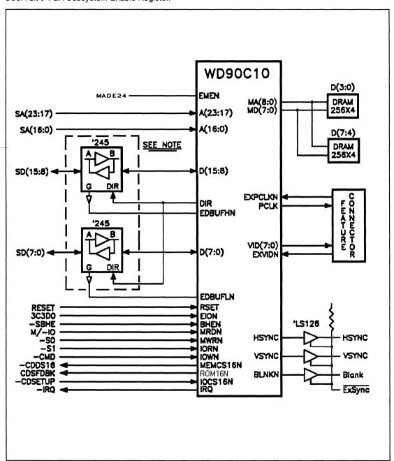
FIGURE 14. 16-BIT MICRO CHANNEL INTERFACE
