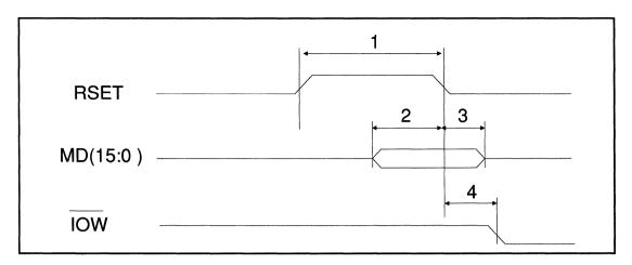
**FIGURE 4. RESET TIMING**
