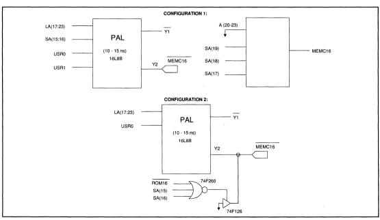
FIGURE 12. WD90C10 INTERFACE FOR 286 OR 386-BASED SYSTEMS
