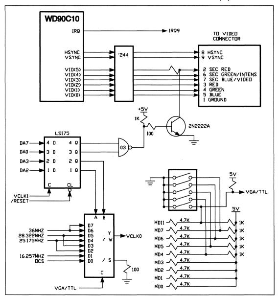
FIGURE 16. WD90C10 AND TTL MONITOR CONNECTIONS
