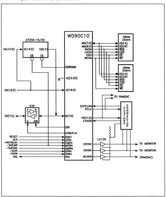
FIGURE 10. 8-BIT PC AT INTERFACE WITH 8-BIT BIOS
