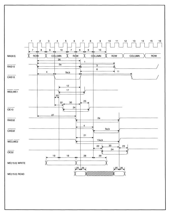
FIGURE 8. CPU READ/WRITE DRAM TIMING
