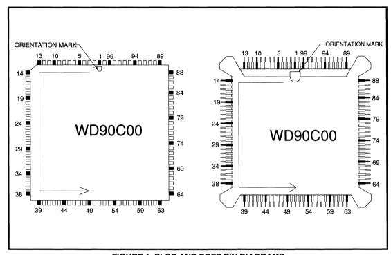
FIGURE 1. PLCC AND PQFP PIN DIAGRAMS
