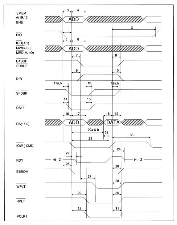
FIGURE 7. MICRO CHANNEL I/O & MEMORY READ & WRITE TIMING
