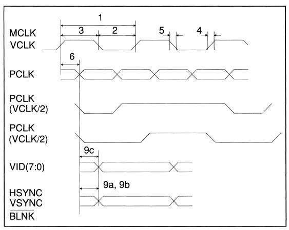
FIGURE 5. CLOCK AND VIDEO TIMING
