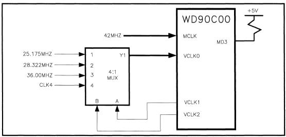
FIGURE 20. EXTERNAL MULTIPLEXING OF THE VIDEO CLOCKS
