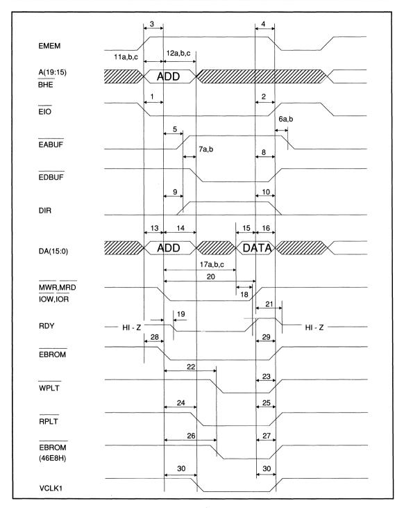
FIGURE 6. AT MODE I/O & MEMORY READ/WRITE TIMING
