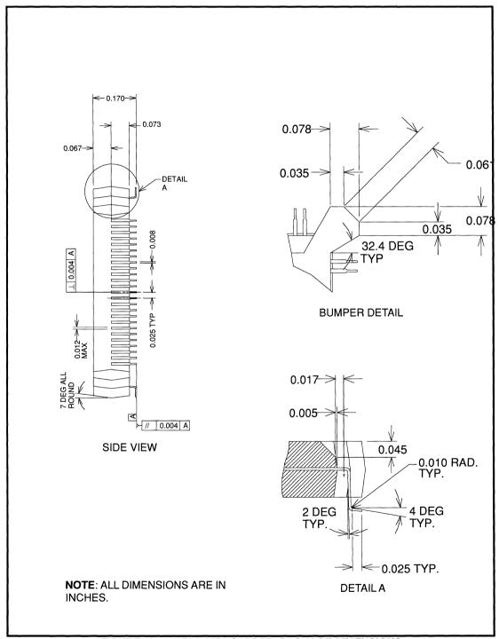
FIGURE 23. 100-PIN JEDEC (PQFP) PACKAGE DIMENSIONS
