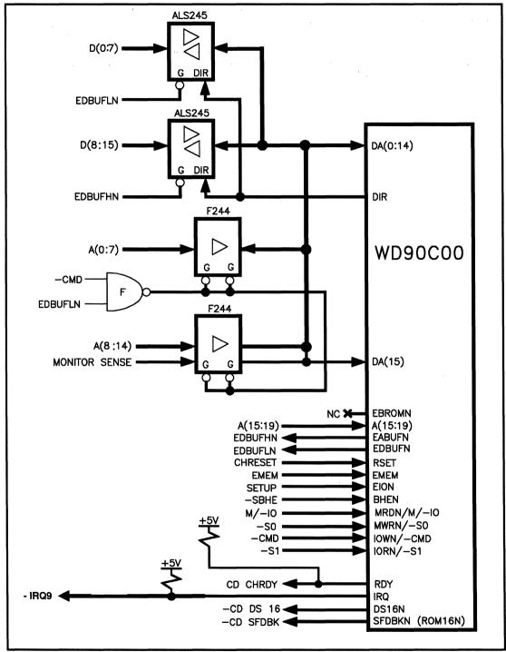
FIGURE 15. 16-BIT MICRO CHANNEL INTERFACE
