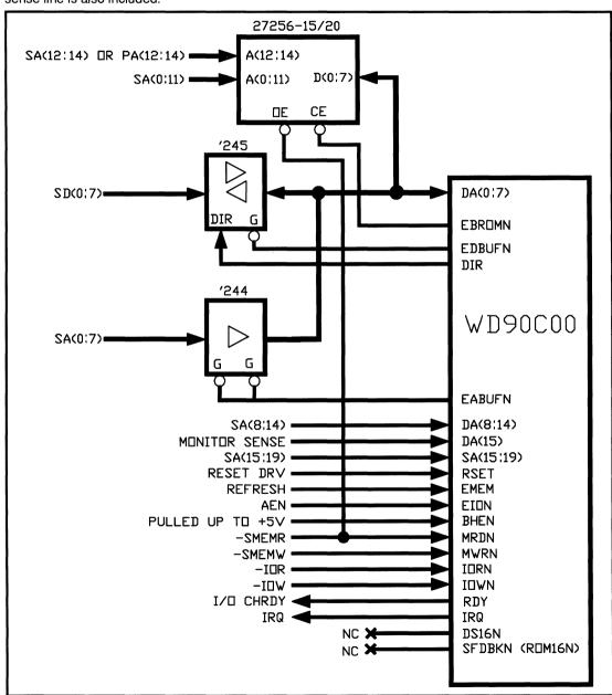
FIGURE 12, 8-BIT PC/AT INTERFACE WITH 8-BIT BIOS
