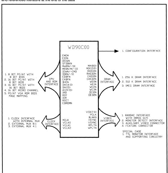
FIGURE 11. WD90C00 PROCESSOR, MEMORY, AND I/O INTERFACES
