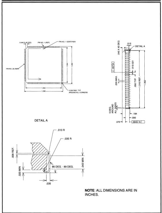
FIGURE 21. 100-PIN PLCC PACKAGE DIMENSIONS
