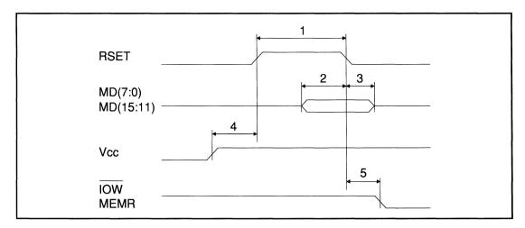
FIGURE 4. RESET TIMING
