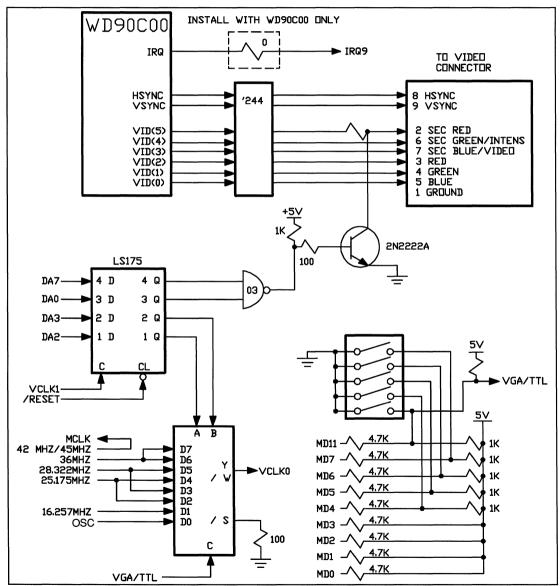
FIGURE 18. WD90C00 TTL MONITOR CONNECTIONS
