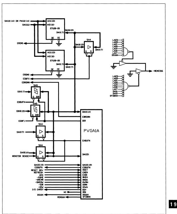
Figure 19. 16-Bit PC/AT Interface With 16-Bit BIOS
