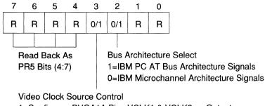
1=Configures PVGA1A Pins VCLK1 & VCLK2 as Outputs 0=Configures PVGA1A Pins VCLK1 & VCLK2 as Inputs
