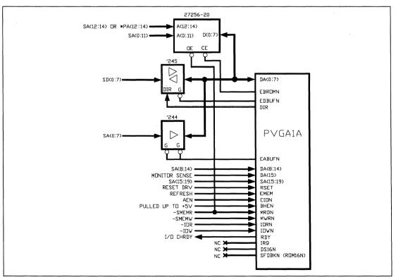
Figure 17. 8-Bit PC/XT Interface With 8-Bit BIOS
