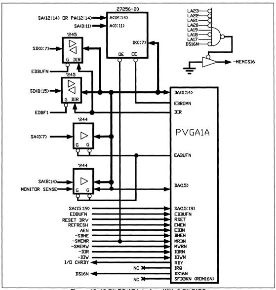
Figure 19 describes 16-bit PC/AT interface with 16-bit BIOS ROM implementation using PVGA1A. The system data bus SD(0:15), address bus SA(0:19), address and data bus buffers, and auto monitor sense input is presented. The (16KX8) upper and lower byte EPROMS, output enable lines (EROM0 / EROM1), and EPROM buffer (Gated by EDBFX) are shown. Note that
