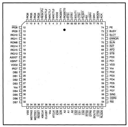
FIGURE 1-1. 84-PIN PLCC - SIGNAL/PIN ASSIGNMENT
