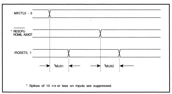
FIGURE 6-11. INTERRUPT MUX TIMING - A
