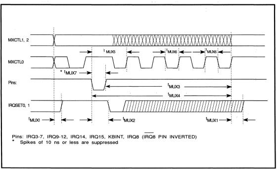
FIGURE 6-12. INTERRUPT MUX TIMING - B
