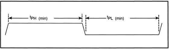
FIGURE 6-10. CLOCK GENERATION TIMING
